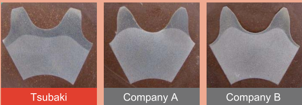
Cross-sectional observation of tooth hardening (darker area is the hardened layer)
