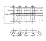
■Connecting link: Spring clip: RS35-NEP – RS60-NEP Cotter pin: RS80-NEP - RS160-NEP \*Riveting is standard on all Neptune chains.
