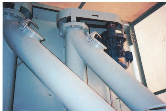
High-neck type used for screw conveyor outlet chutes
