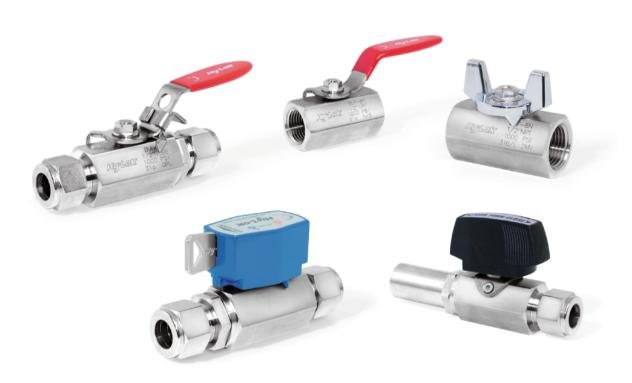
Max allowable working pressure up to 3000 psig (206 bar) at 100°F (38°C) Material available in 316 SS, Brass, Monel Alloy 400, Hastelloy® C-276, Super Duplex Size from 1/4" to 2" (Tube & Pipe Thread)
