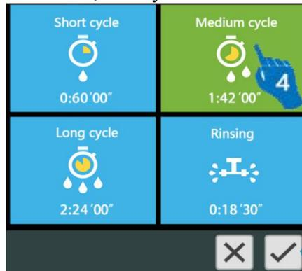
③ After setting the date and time, select a cleaning process and click  to confirm the setting
