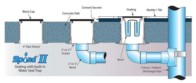
Special design from SPIND MALAYSIA of "SPIND" Floor Gully/Trap is unique in that it allows cleaning/rodding from the bathroom itself. There is no need to go below the floor slab or to remove the false ceiling for cleaning/rodding purposes. (ideal for ground floor, condominiums, flats, hotels, high rise and double storey house applications)
