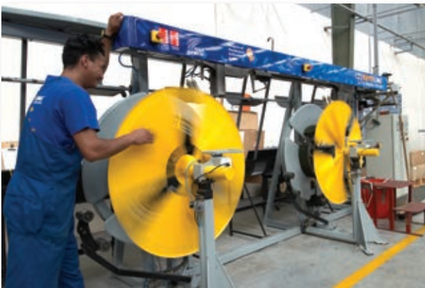
Manufacturing coils on the Buteline Pipewinder
