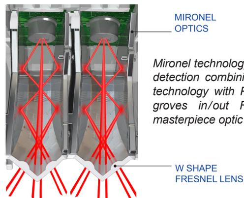
*Mironel technology is a step ahead in detection combining mirror reflection technology with Paradox's W shape grooves in/out Fresnel lens – a masterpiece optic solution package.*
