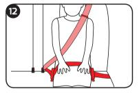
Ensure that the lap portion of the vehicle seat belt has passed through the lap belt slots on both sides of the booster seat.
