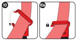
To position the shoulder belt guide, attach the shoulder belt guide to the diagonal portion of the vehicle seat belt, by opening the clip and inserting the seat belt. Then close the clip.
