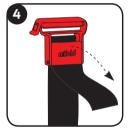
To access the shoulder belt guide strap, pull open the shoulder belt guide buckle.
