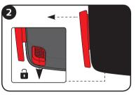
To unlock the lap belt guides, slide the Lap Belt Guide Release button forward. To lock the guides, release the Lap Belt Guide Release button.
