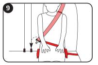
Extract the vehicle seat belt and pass it across the front of your child. Slide lap belt portion of vehicle seat belt through both lap belt guides and connect the seat belt tongue into the vehicle buckle.
