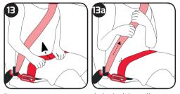
Remove any twists or seat belt slack by pulling on the lap portion and then the diagonal portion of the adult seat belt.
