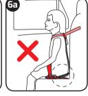
Ensure that the booster seat is laid flat and up against the back rest of the vehicle seat.
