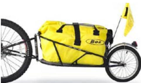
BOB YAK PLUS: A LONG-TIME FAVOURITE AMONG BIKE TOURISTS. SOLID, EASY TO ASSEMBLE AND CAN BE FLIPPED OVER TO USE AS A TABLE.
