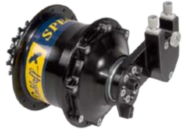
THE ROHLOFF HUB: A HIGH-TECH PIECE OF TOURING GEAR WITH MANY BENEFITS. IT ALSO ADDS $1,200 U.S. TO THE PRICE OF YOUR BIKE.
