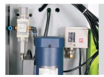
Efficient air filter device, to prevent moisture entry into machine inside. Real-time detection of low air source pressure to ensure machine normally working.
