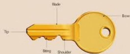
PARTS OF A KEY
