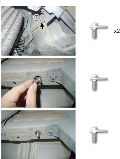
**STEP II:** Tighten the SUPERCIRCUIT Rear Under Brace with bolts & washer provided from the undercarriage direction.
