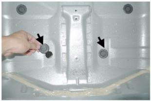
**STEP II:** Insert the bolts & larger washer from inside the spare wheel compartment through the holes after removing the rubber plugs in STEP I.
