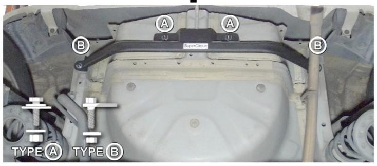
Thank you for the purchase. Please utilize the provided bolts & nuts to install the SUPERCIRCUIT Rear Under Brace to the Perodua Axia as shown in the picture above.
