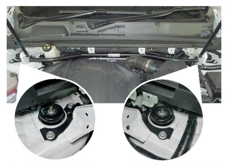
To reinstall the original engine covers after the SUPERCIRCUIT Front Strut Bar is installed, repeat Step 1-4 in reverse sequence.
