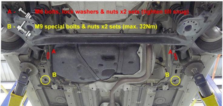
STEP 2: Insert the provided M6 bolts + washers to locations A. Tighten untill snug.
