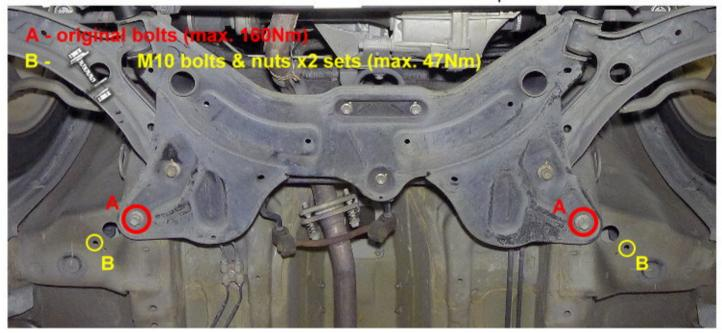
STEP 2: Insert the provided bolts + washers via the opening at B. Tighten according.
