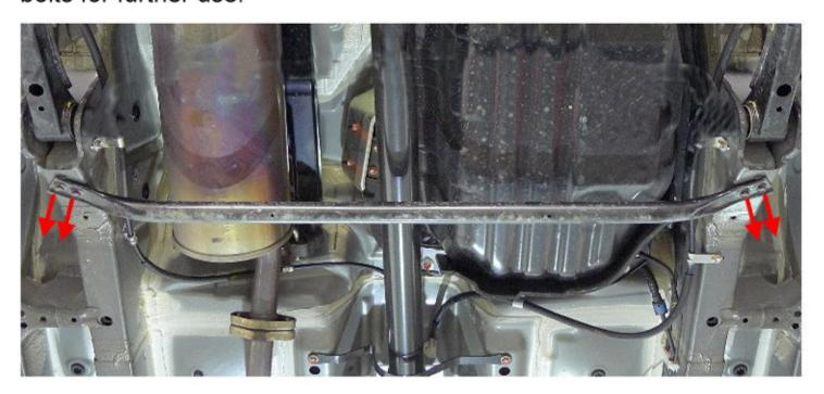
STEP 2: Insert the provided bolts via the bigger openings on the chassis and allow the thread section of the bolts pointing downwards.
