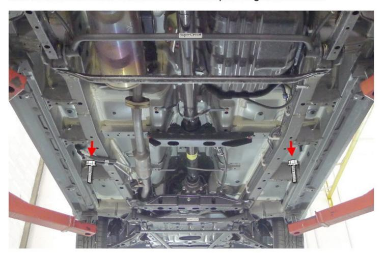
STEP 3: Fasten the washers and nuts provided to the bolts pre-inserted in STEP 2 to the front section of the SUPERCIRCUIT Mid Chassis Brace.
