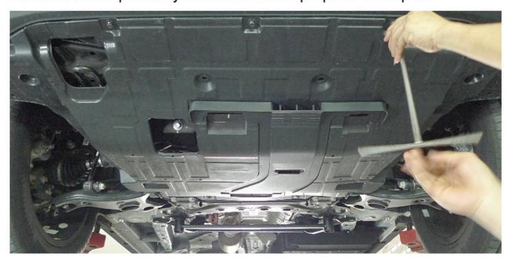
Step 2: Install the SUPERCIRCUIT Front Under Brace with the original bolts as shown in the pictures below.
