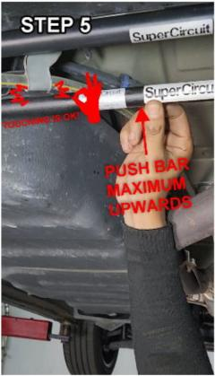
Push maximum upwards\* and tighten the bolts & nuts in STEP 4.
