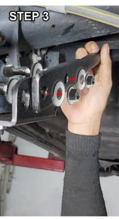
Insert the bolts & washer from the top as shown in the picture.
