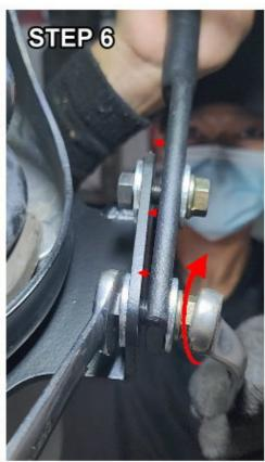
Now, you can tighten all the bolts & nuts with min. 25Nm tightening torque.
