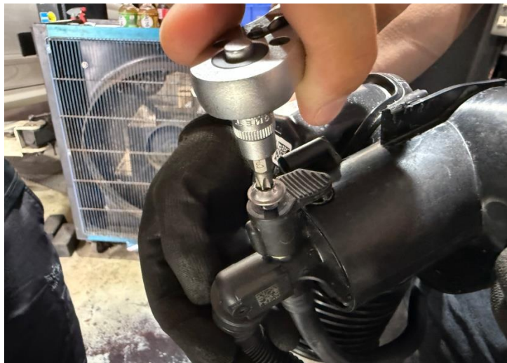
Figure 14: Remove the PCV assembly from the stock inlet tube.
