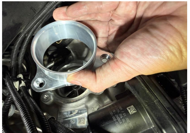
Figure 12: Install the MST turbo onlet adapter.
