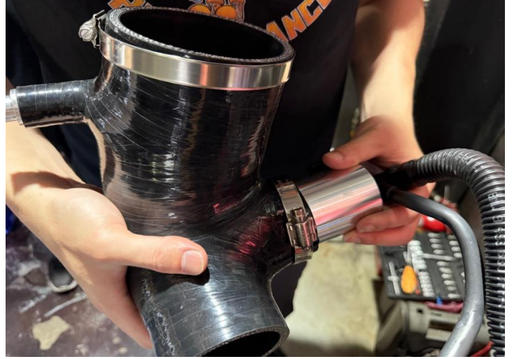
Figure 16: Install the PCV assembly onto the MST inlet hose.
