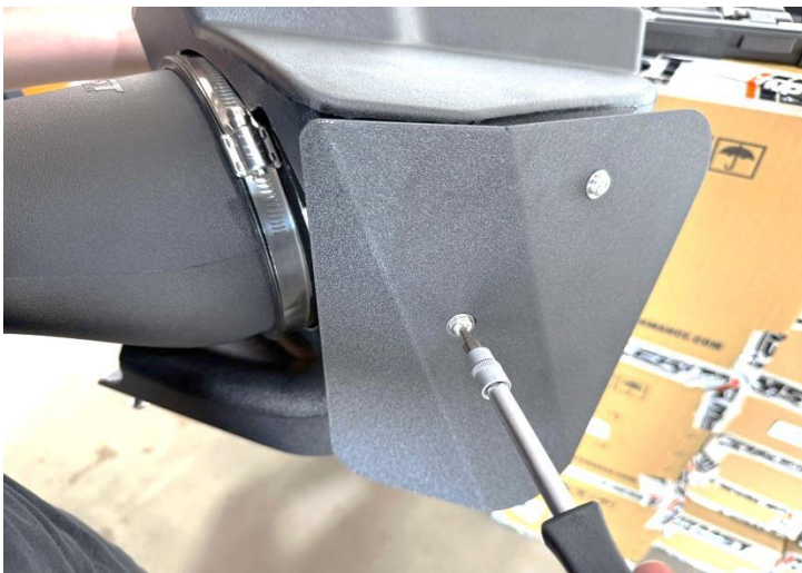
Figure 21: Install the heat shield on the air box and install the aluminum mounting standoffs on to the air box.
