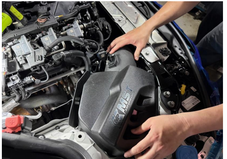
Figure 24: Install the heat shield on the air box and install the aluminum mounting standoffs on to the air box.
