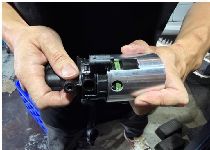
Figure 15: Install the PCV assembly onto the MST cnc adapter.
