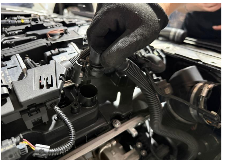
Figure 6: Remove the PCV hose from the engine.
