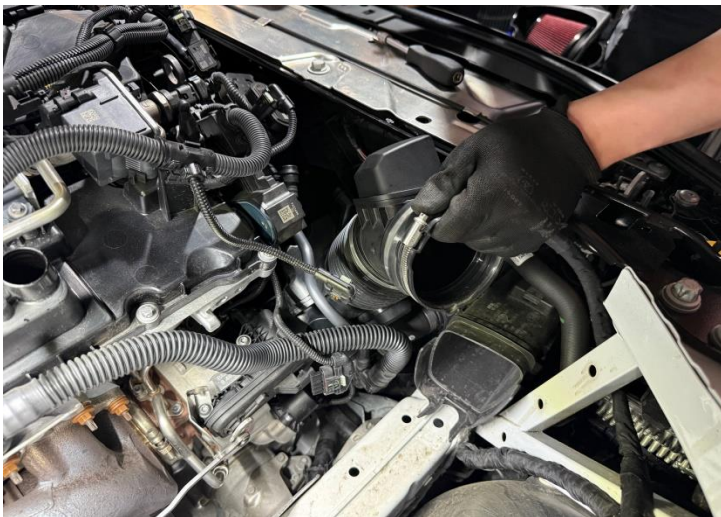
Figure 9: Remove the stock turbo inlet tube.
