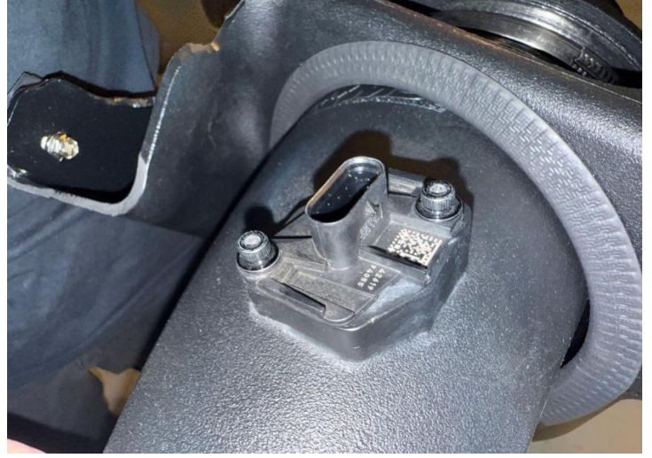
Figure 22: Install the MAF sensor on the MST tube.
