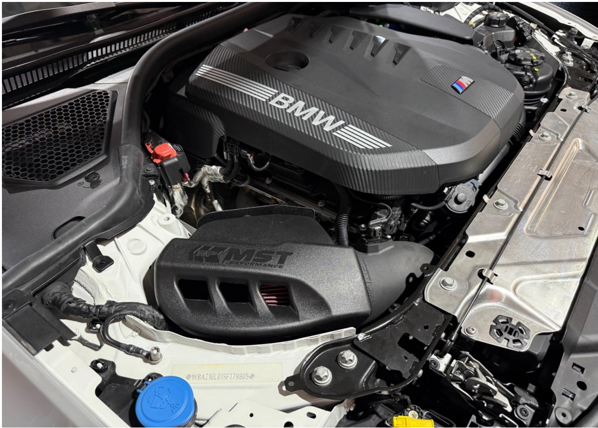
Figure 25: Congratulations! You have just completed the installation of this intake system. Periodically, check the alignment of the intake, normal wear and tear can cause nuts and bolts to come loose.
