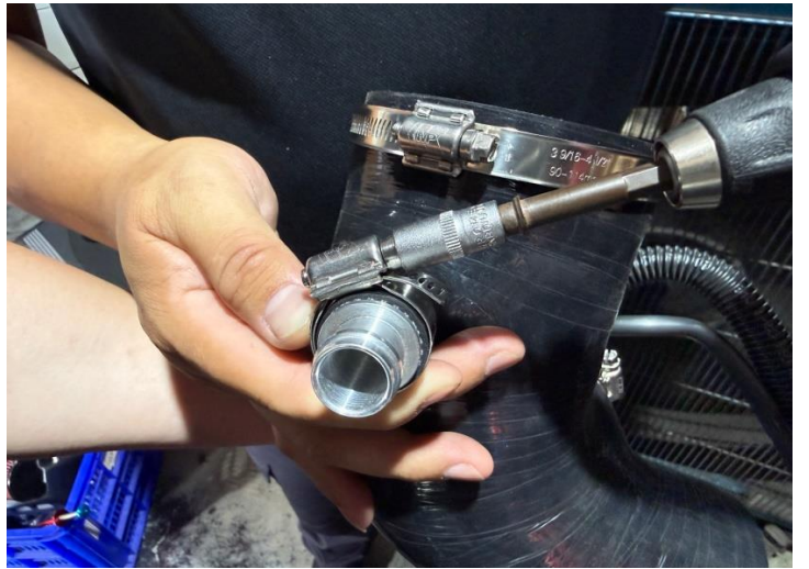
Figure 17: Install the PVC adapter onto the MST inlet hose.
