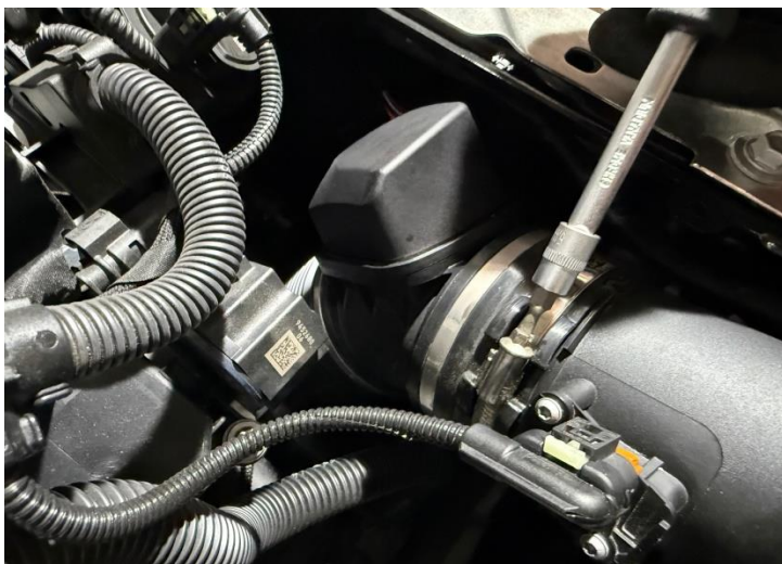
Figure 3: Loosen the hose clamp.
