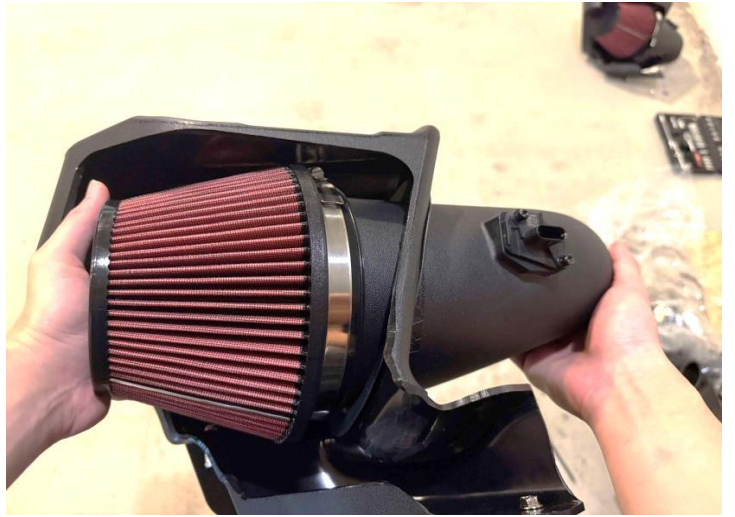
Figure 23: Install the air filter.
