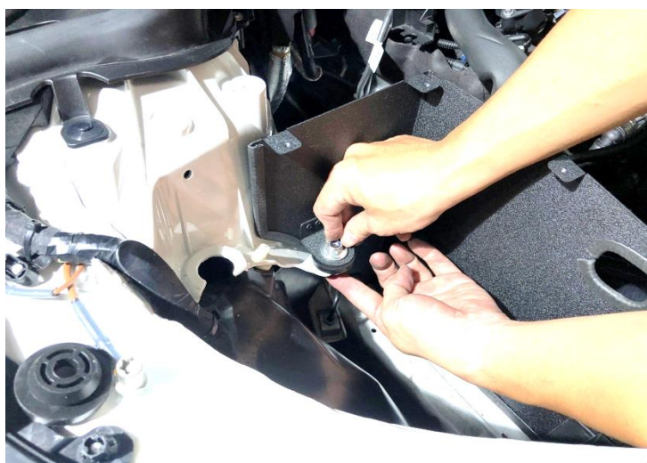
Figure 15: Secure the heat shield breaket with bolt. 用對鎖螺絲固定隔熱罩支架
