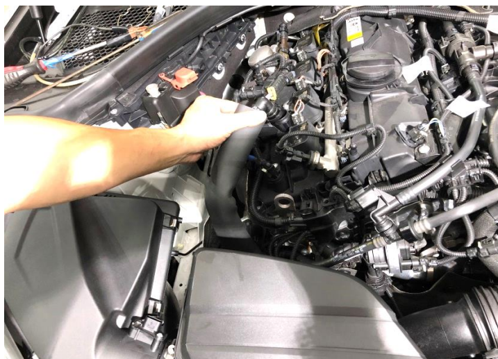
Figure 4: Remove the PCV. 移開PCV管
