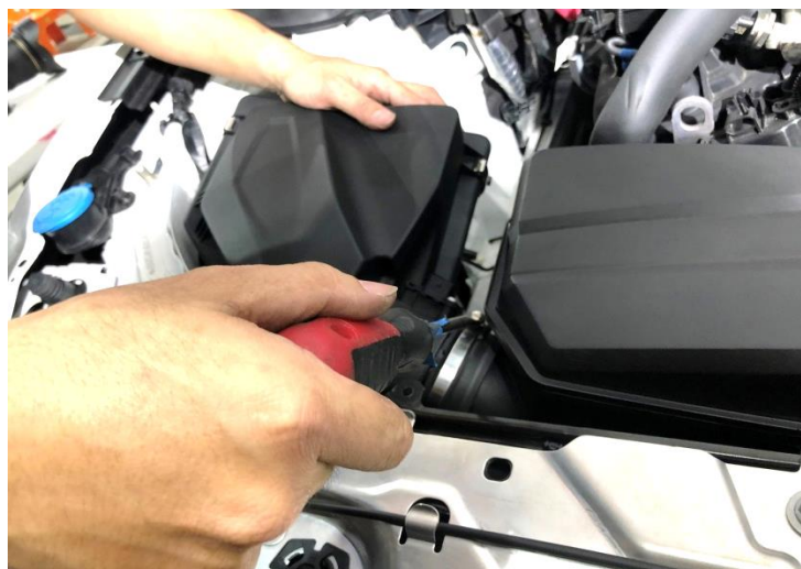
Figure 1: Loosen the hose clamp. 鬆開管束
