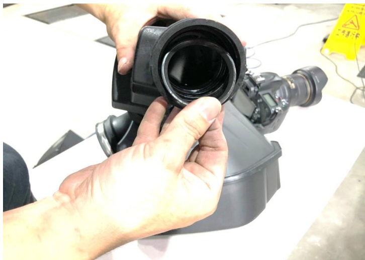
Figure 9: Remove the O-Ring. 拆下原廠氣密環
