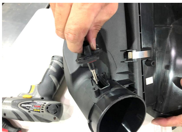
Figure 17: Remove the mass air flow sensor from the stock air box. 從原廠集氣箱移除空氣流量感知器
