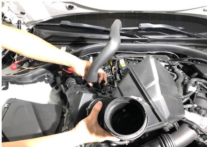
Figure 7: Remove the stock turbo inlet pipe. 移除原廠渦輪進氣管
