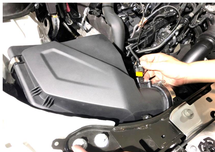
Figure 2: Disconnect the mass air sensor. 斷開空氣流量感知連接器
