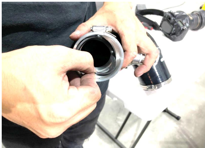
Figure 10: Install the O-Ring. 把原廠氣密環裝進MST渦輪進氣管
