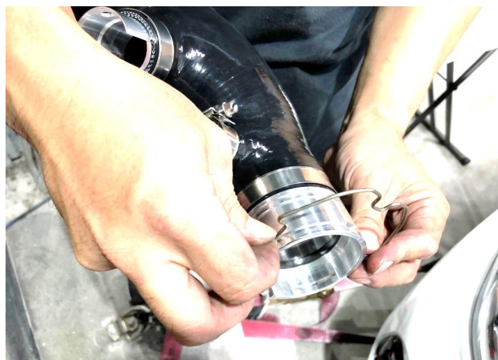
Figure 11: Install the spring. 把原廠渦輪進氣管彈簧裝上MST渦輪進氣管
