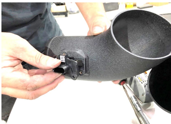
Figure 18: Install mass air sensor into the intake pipe. 將空氣流量感知器安裝在MST進氣管上
