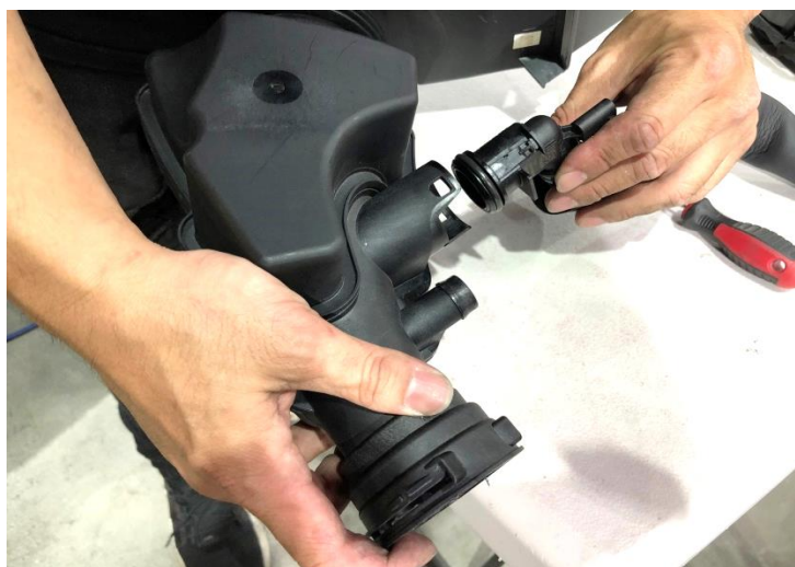
Figure 8: Remove the PCV. 移開PCV管
