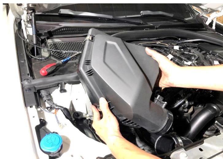
Figure 3: Remove the stock air box. 移除原廠集氣箱
