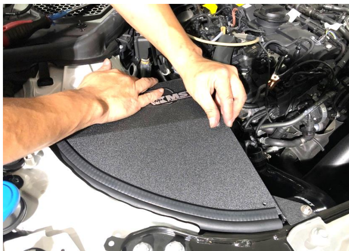
Figure 22: Install the heat shield cover and secure with bolt 蓋上隔熱上蓋並鎖上螺絲
