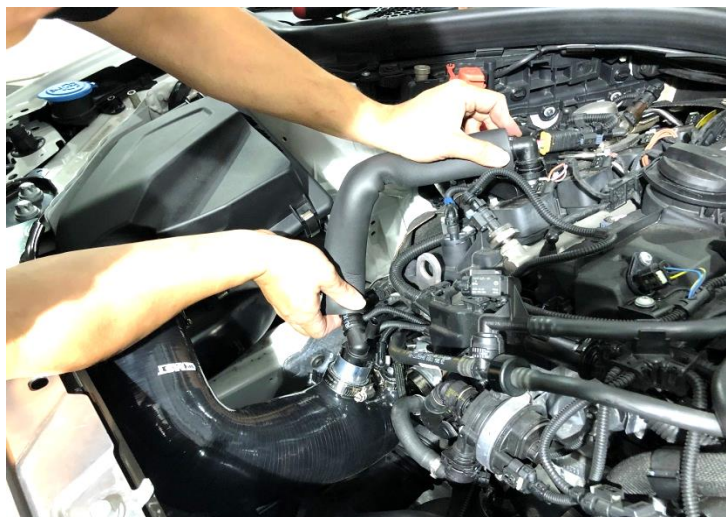
Figure 13: Install the PCV. 插上PCV管
