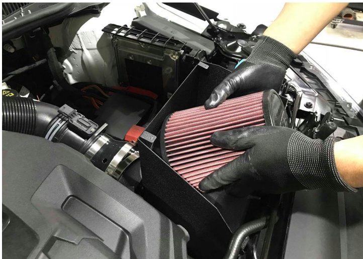
Figure 9: Install the air filter.
