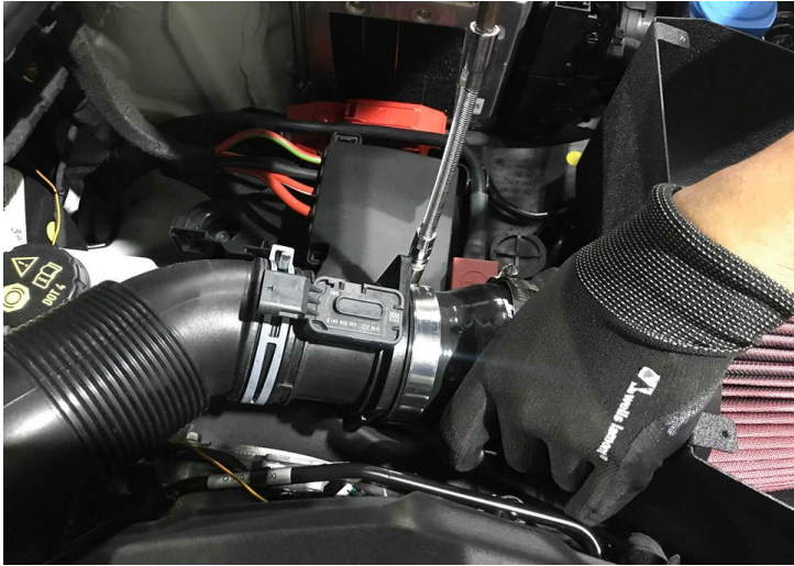
Figure 9: Tighten the hose clamp.
