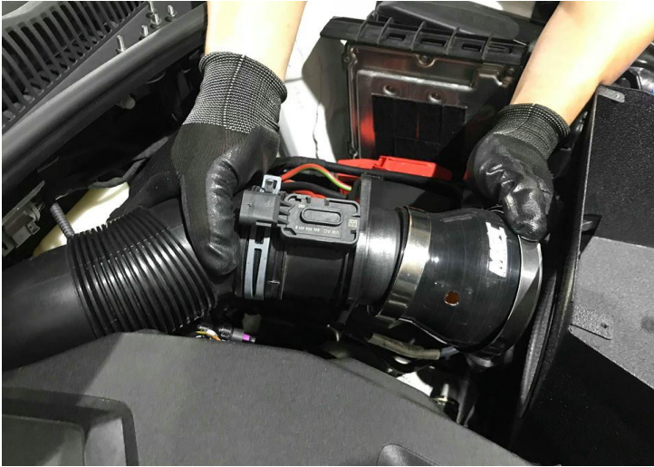
Figure 7: Install the silicone hose.
