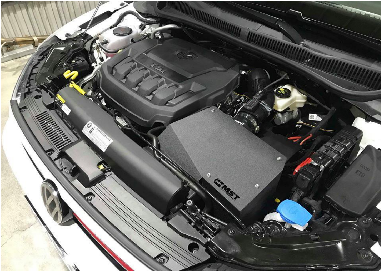
Figure 13: Congratulations! You have just completed the installation of this intake system. Periodically, check the alignment of the intake, normal wear and tear can cause nuts and bolts to come loose.
