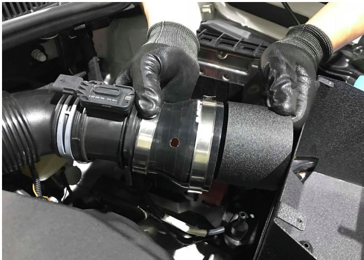
Figure 8: Install the intake tube.
