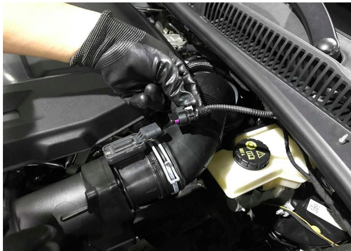
Figure 2: Disconnect the mass air sensor.
