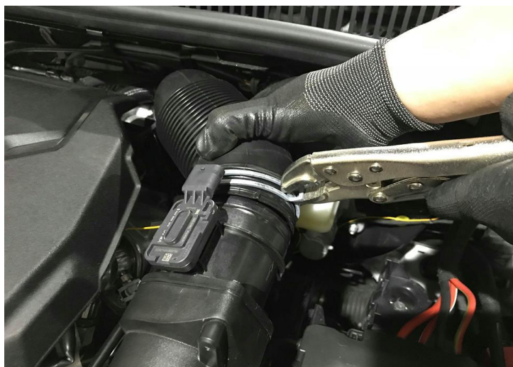
Figure 3: Loosen the clamp.
