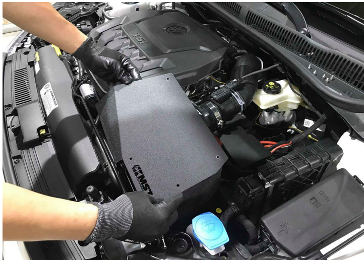
Figure 11: Install the heat shield cover.
