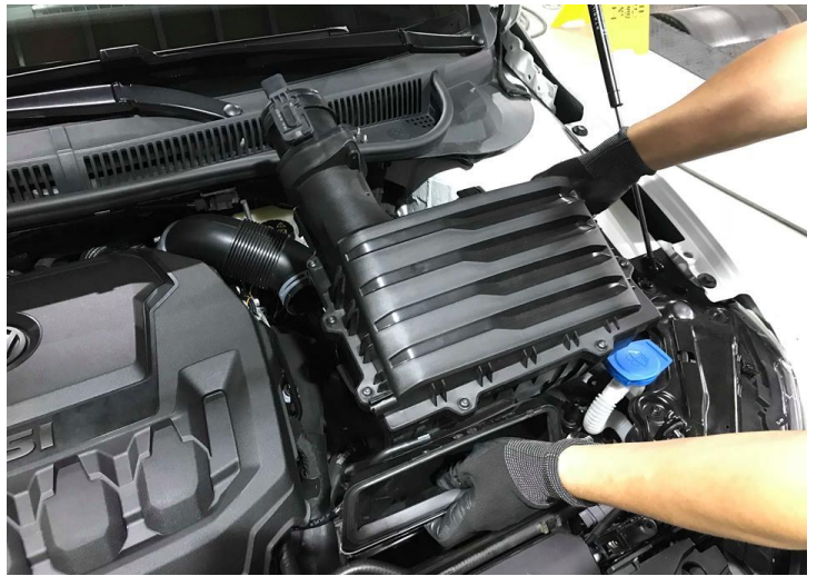
Figure 4: Remove the stock air box.
