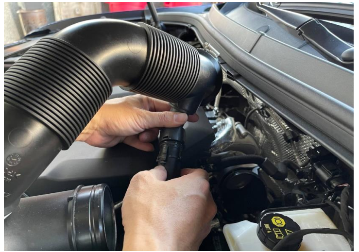
Figure 4: Remove the stock PCV and inlet tube
