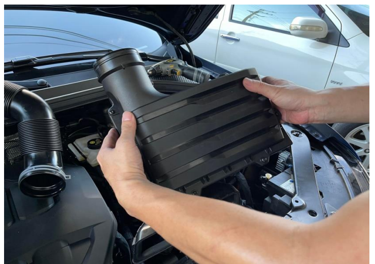
Figure 6: Remove the stock air box and air scoop.
