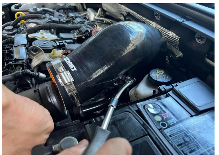
Figure 11: Connect the recirculation hose.
