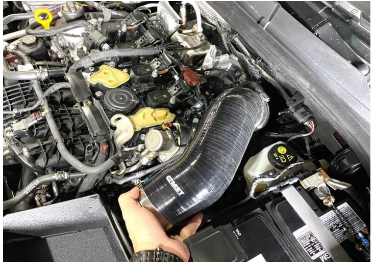
Figure 10: Install the MST silicone hose.
