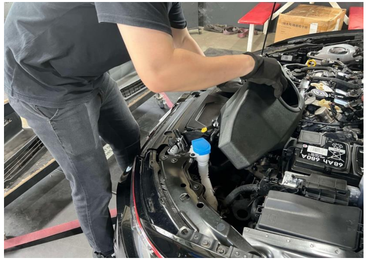
Figure 10: Install the MST air box.
