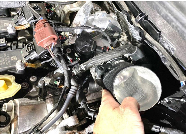
Figure 8: Install the MST inlet elbow and tight the bolt.
