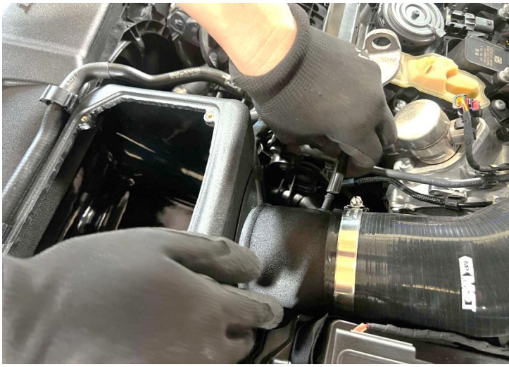
Figure 13: Install the MST tube and connect the 4mm hose.
