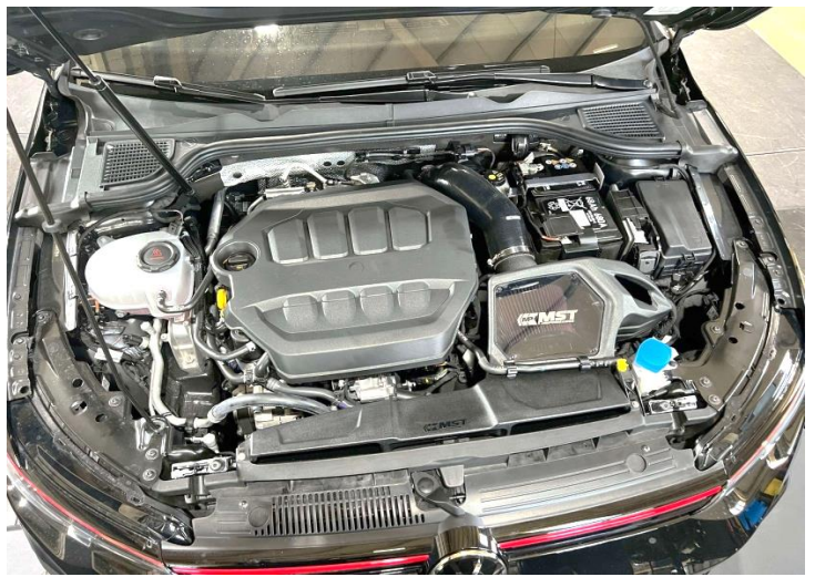
Figure 16: Congratulations! You have just completed the installation of this intake system. Periodically, check the alignment of the intake, normal wear and tear can cause nuts and bolts to come loose.
