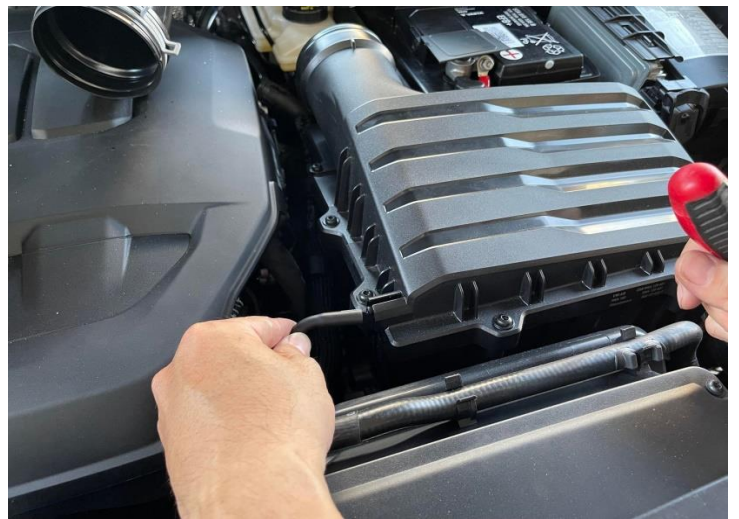
Figure 5: Remove the stock PCV hose.
