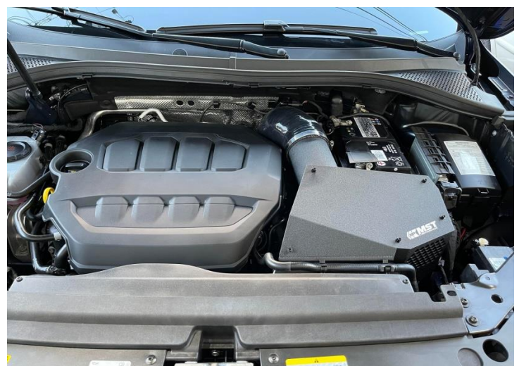
Figure 12: Congratulations! You have just completed the installation of this intake system. Periodically, check the alignment of the intake, normal wear and tear can cause nuts and bolts to come loose.
