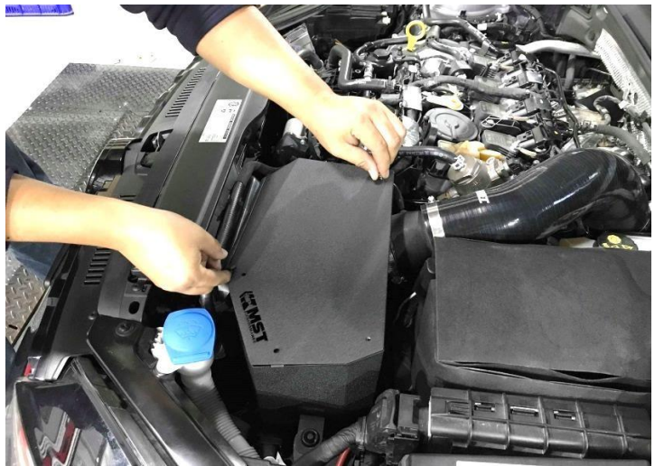
Figure 17: Install the heat shield cover and secure with bolt.
