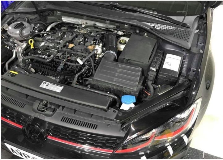
Figure 7: Turn the turbo inlet pipe clockwise (t theowards firewall) and it'll come off when it's rotated and you enough pull.
