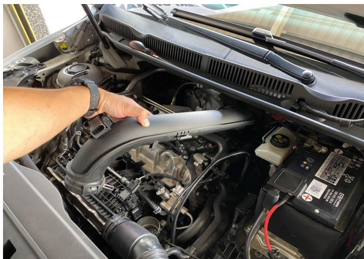
Figure 7: 移除原廠渦輪管
