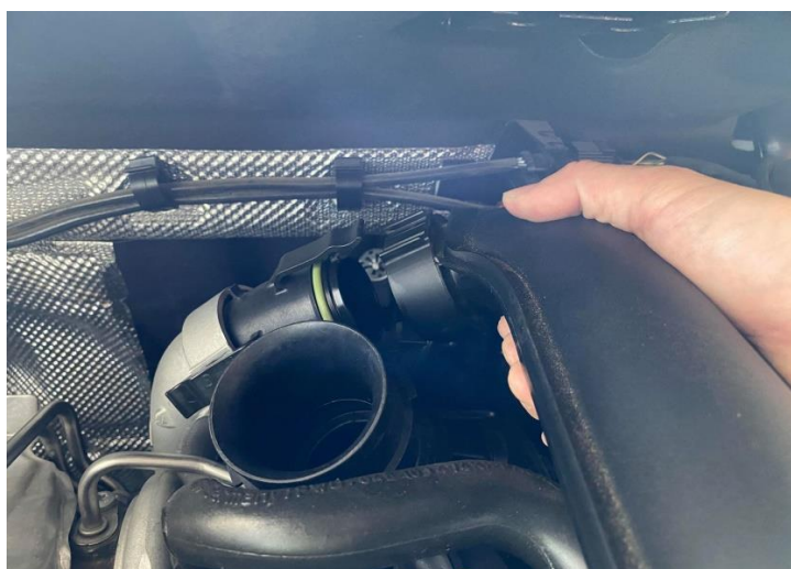
Figure 6: 鬆開原廠渦輪管卡扣
