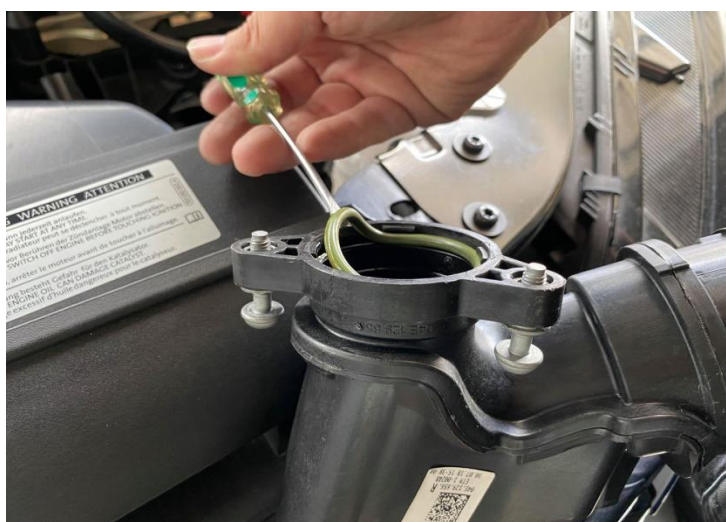
Figure 8: 將原廠渦輪管內部O-RING取出
