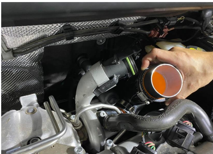
Figure 12: MST加大進氣管路安裝至MST轉座上
