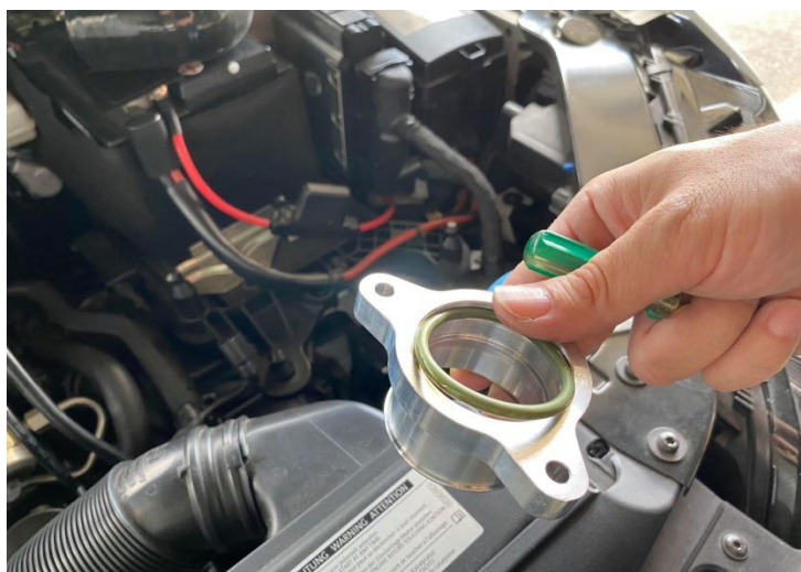
Figure 9: 將原廠O-RING安裝至MST轉接座內
