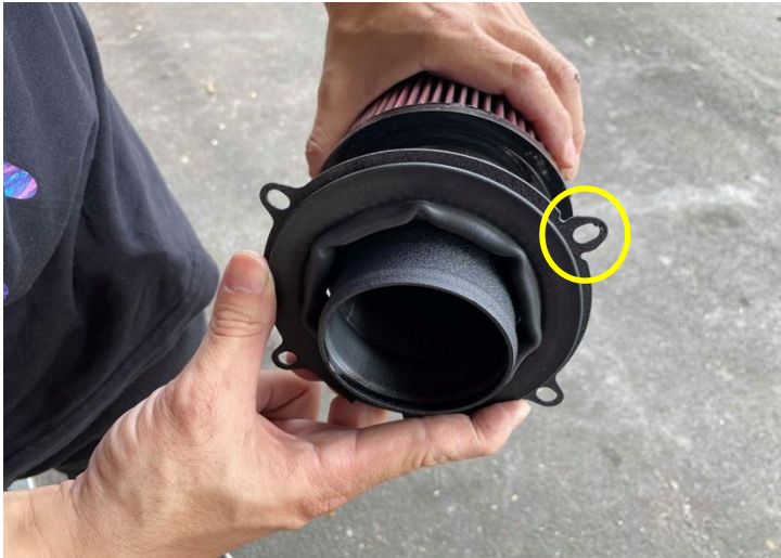
Step 7. Slide the adaptor pipe neck plate onto the air filter adaptor, please take note the position of the specially marked mounting tab of the neck plate
