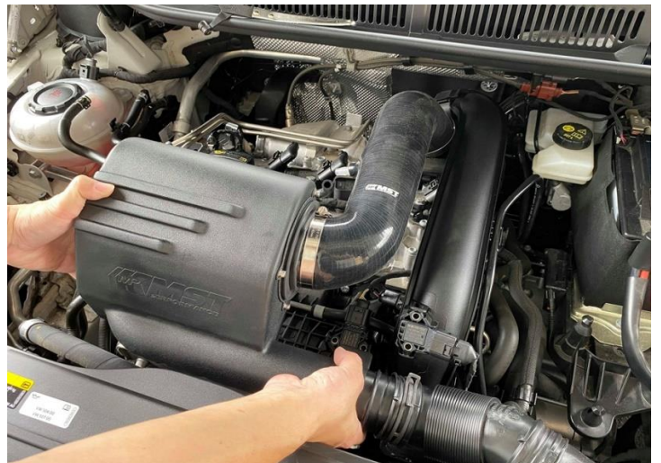
Step 12. Carefully position the 3 rubber gromets (under the air box) to the vehicle mounting points and install into position
