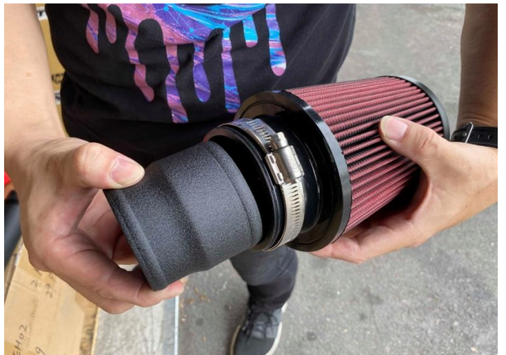
Step 5. Slide hose clamp onto the air filter, insert air filter adaptor pipe into the air filter as shown
