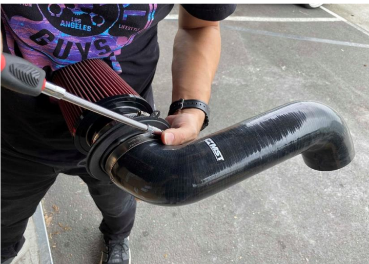
Step 9. Tighten the hose clamp on the main intake silicone pipe as shown
