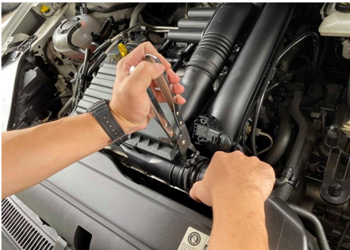
Step 2. Unclamp the intake duct spring clamp as shown and move away the spring clamp from the original clamped position
