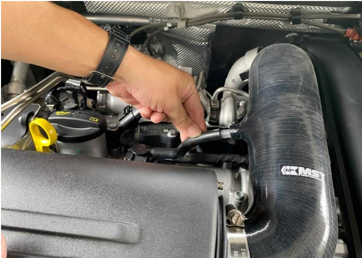
Step 13. Reconnect the PCV hose onto the plastic connector of the MST main intake silicone pipe
