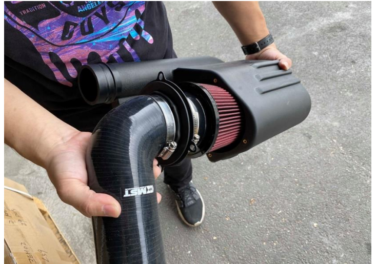
Step 10. Insert air filter into MST heat shield air box as shown
