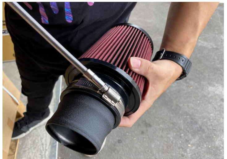
Step 6. Tighten the air filter hose clamp
