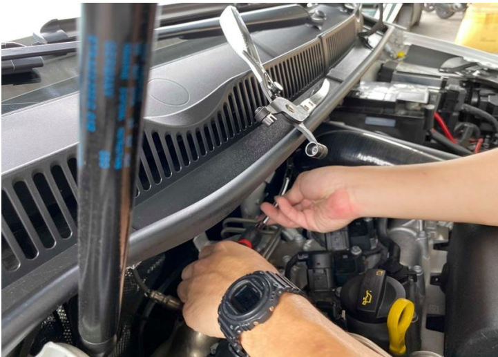
Step 14. Make sure the main intake silicone pipe is inserted onto the turbocharger intake and tighten the hose clamp
