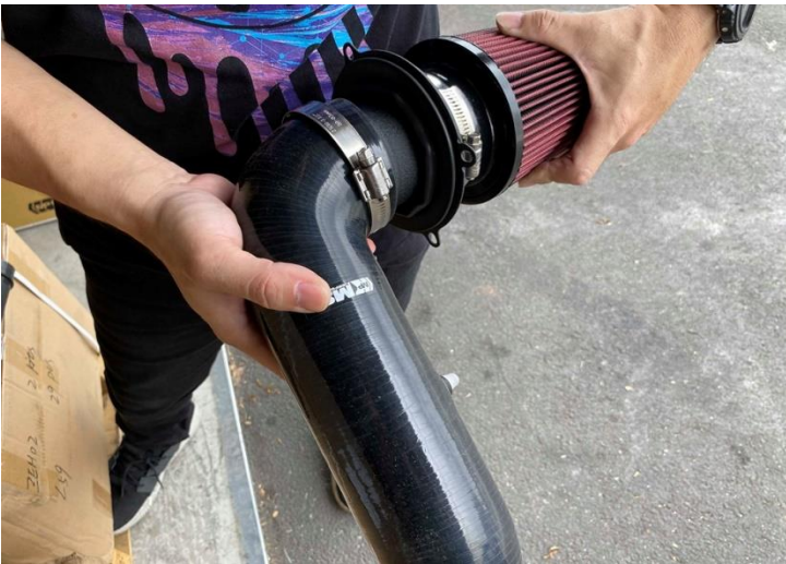
Step 8. Slide hose clamp onto the main intake silicone pipe and slide over the air filter adaptor pipe
