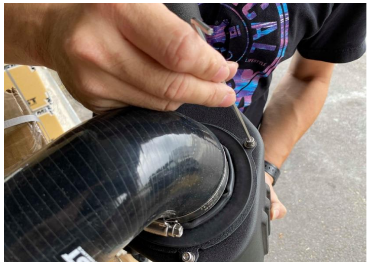
Step 11. Secure air filter adaptor plate onto heat shield air box utilizing M4 bolts
