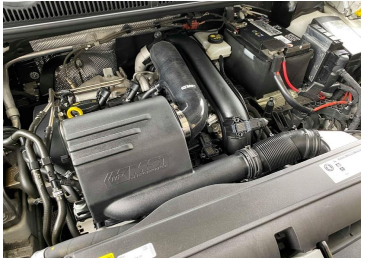
Step 16. Congratulations! You have just completed the MST Performance Induction system installation, be sure to periodically check all of the induction system mounting screws including hose/piping connections if they come loose at all
