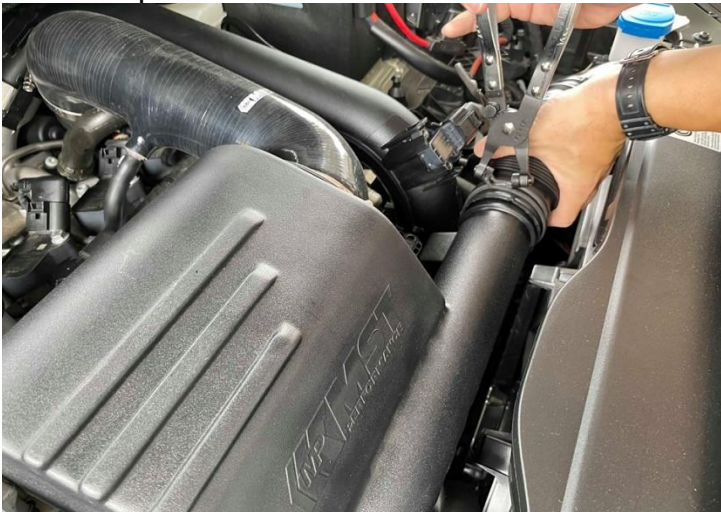
Step 15. Connect the stock air intake duct to the MST air box and clamp back with stock spring clamps
