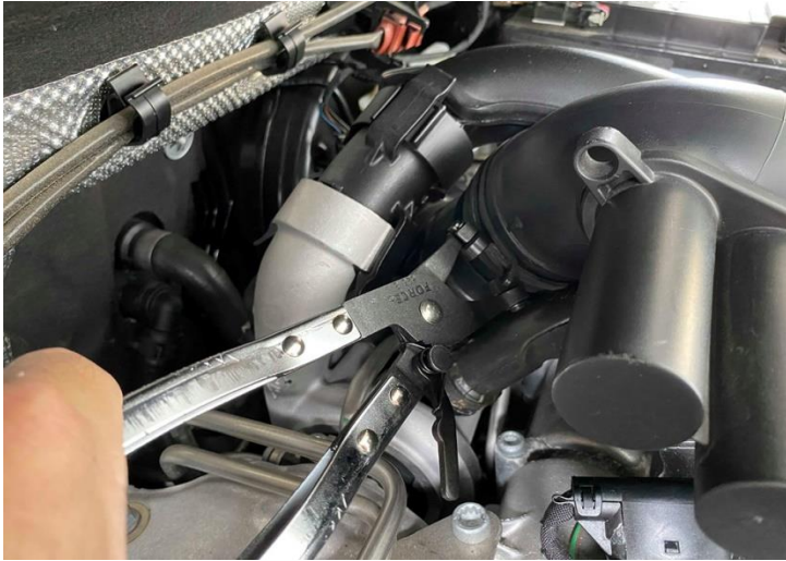
Step 1. Unclamp the stock air intake spring clamp as shown and move away the spring clamp from the original clamped position
