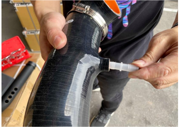
Step 4. Insert the plastic hose adaptor into the main intake silicone pipe as shown
