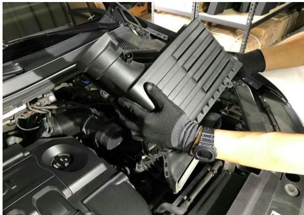
Step 5. Remove the stock air box
