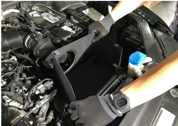
Step 6. Install the heat shield air box
