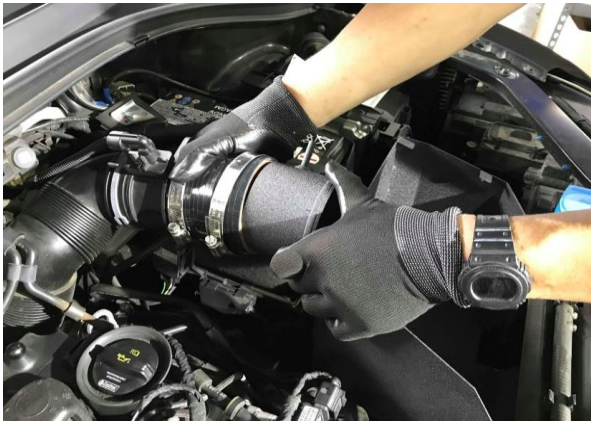
Step 7. Install the intake tube
