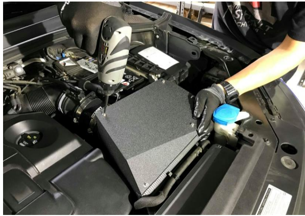
Step 10: Secure the heat shield top cover with 5x retaining screws
