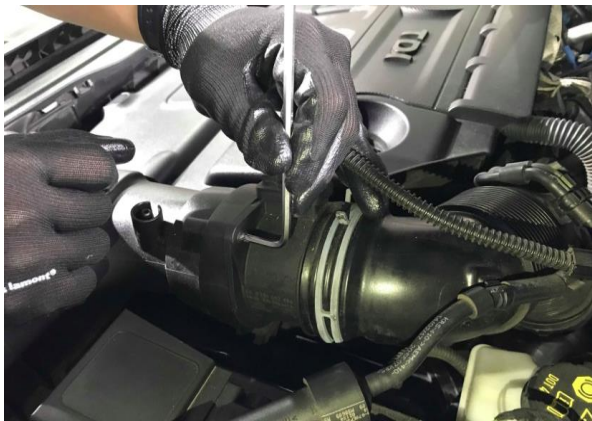
Step 3. Unscrew the MAF screw
