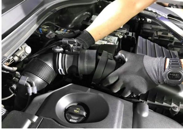
Step 4. Remove the MAF
