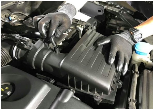
Step 2. Disconnect the Positive Crankcase Ventilation (PCV) hose from the stock induction pipe
