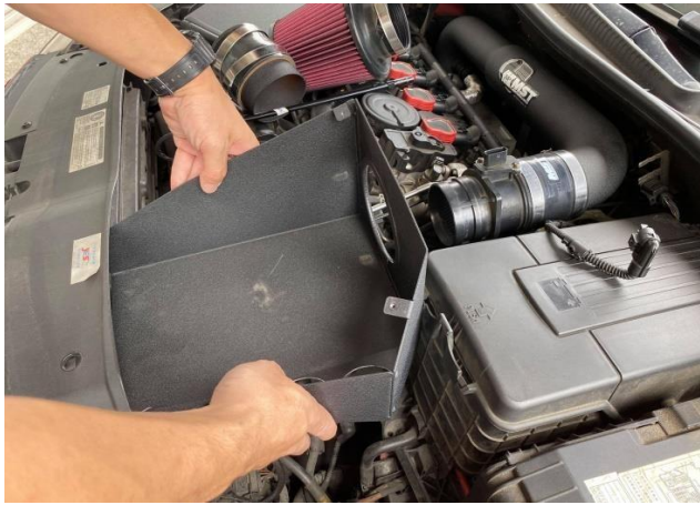
Figure 14: Install the MST heat shield
