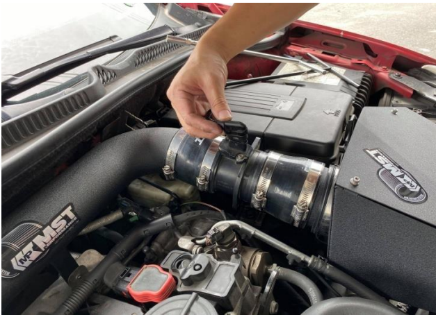
Figure 19: Connect the MAF sensor
