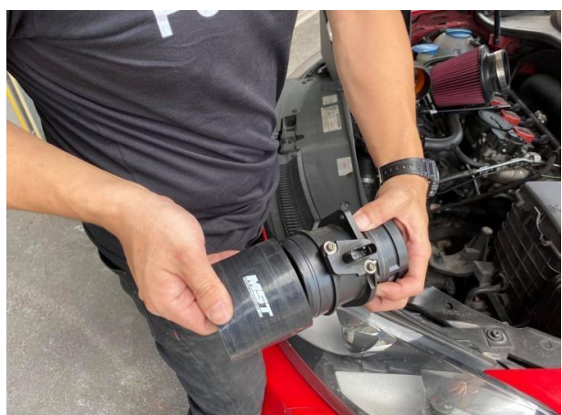
Figure 12: Install the silicone hose on MAF adapter
