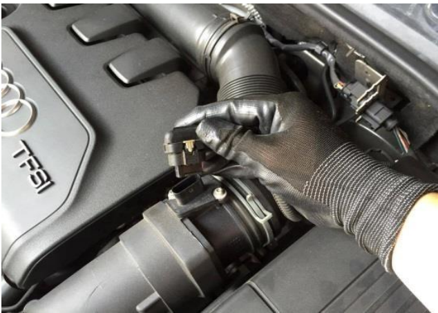
Figure 3: Disconnect the MAF sensor
