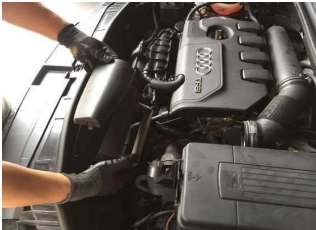
Figure 6 : Remove the air scoop and intake tube.
