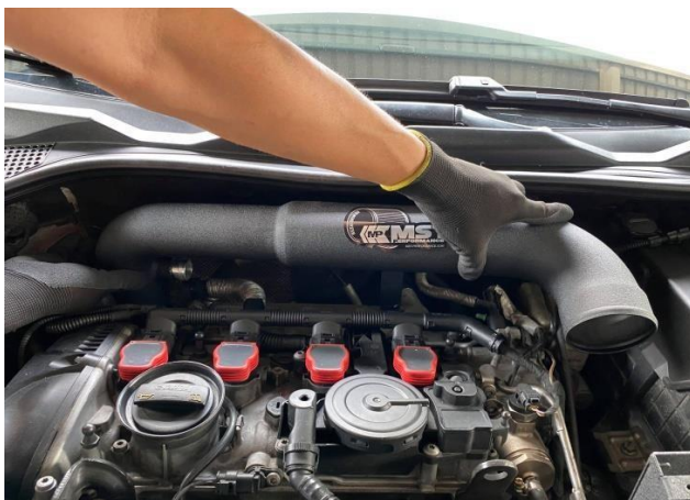
Figure 9: Install the intake pipe.
