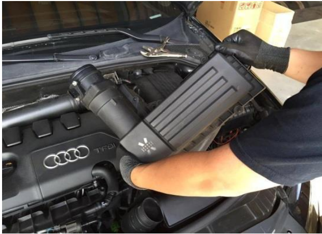
Figure 5: Remove the stock air box
