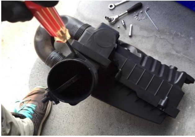
Figure 7: Remove the MAF from stock air box
