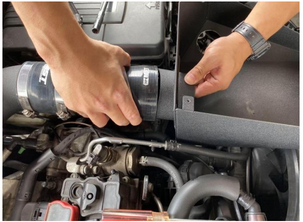
Figure 17: Install the silicon hose and tube on the MAF adapter
