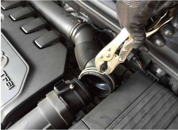
Figure 4: Unclamp the intake duct spring
