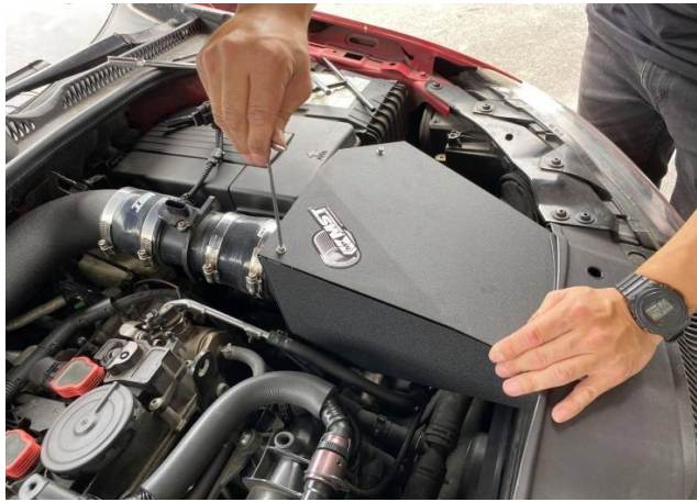
Figure 20: Install the heat shield cover
