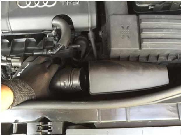
Figure 2: Remove the stock air scoop tube
