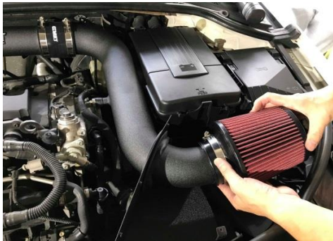
Figure 19: Install the air intake.
