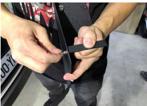
Figure 10: Install bracket on heat shield.
