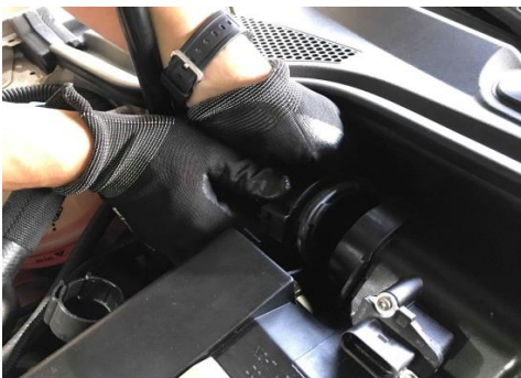
Figure 4: Open the stock inlet hose spring.
