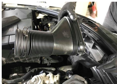
Figure 9: Remove stock scoop.
