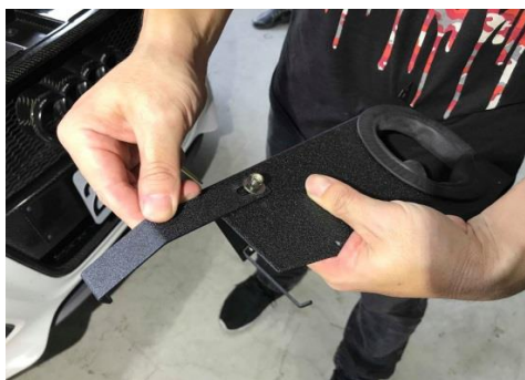
Figure 11: Install bracket on heat shield.
