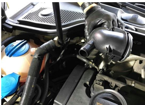
Figure 7: Remove the stock inlet hose.
