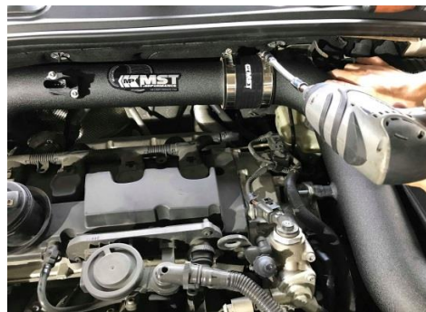
Figure 17: Tighten the hose clamp.
