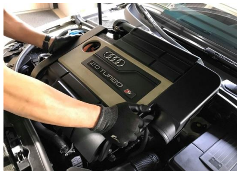
Figure 6. Remove the engine cover.
