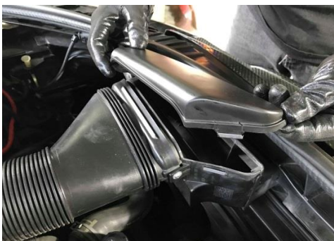
Figure 8: Remove stock scoop cover.
