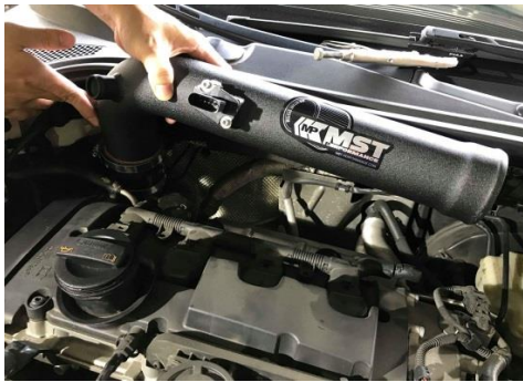
Figure 16: Install the intake pipe.
