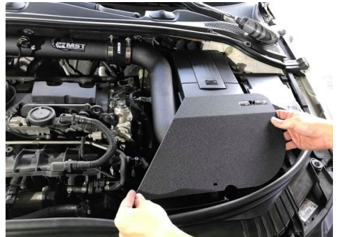
Figure 21: Install the heat shield cover.
