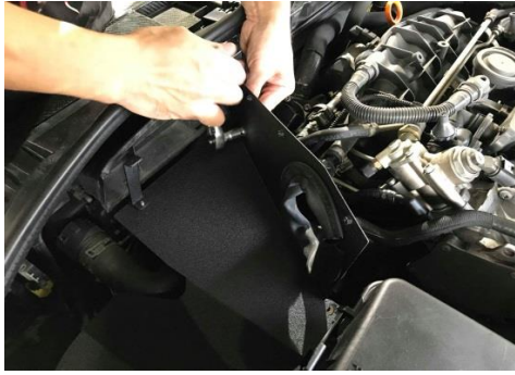
Figure 13: Install the heat shield and secure the breaket with bolt.
