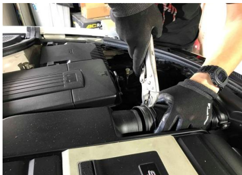
Figure 5. Loosen the hose clamp.
