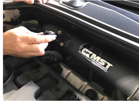
Figure 20: Install the MAF sensor.
