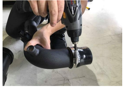
Figure 15: Install the silicone hose.
