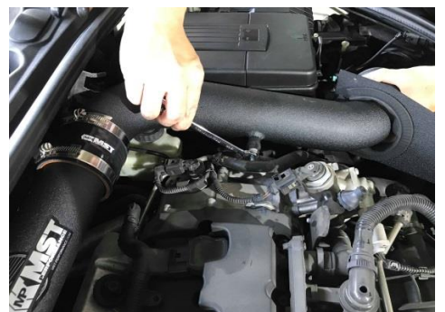
Figure 18: Secure the pipe breaket with bolt.
