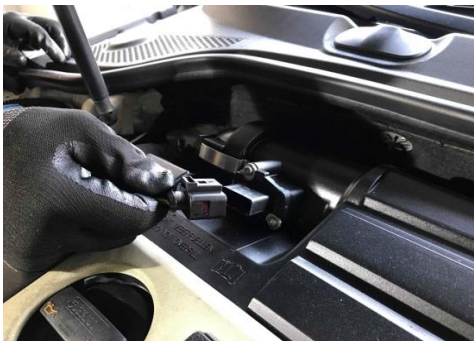
Figure 2. Disconnect the mass air sensor.
