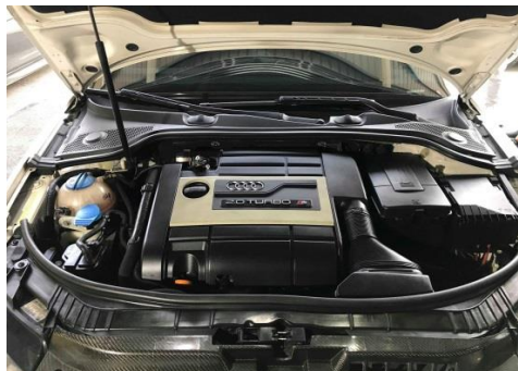
Figure 1. Stock air intake.
