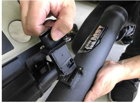
Figure 14: Instell MAF sensor.
