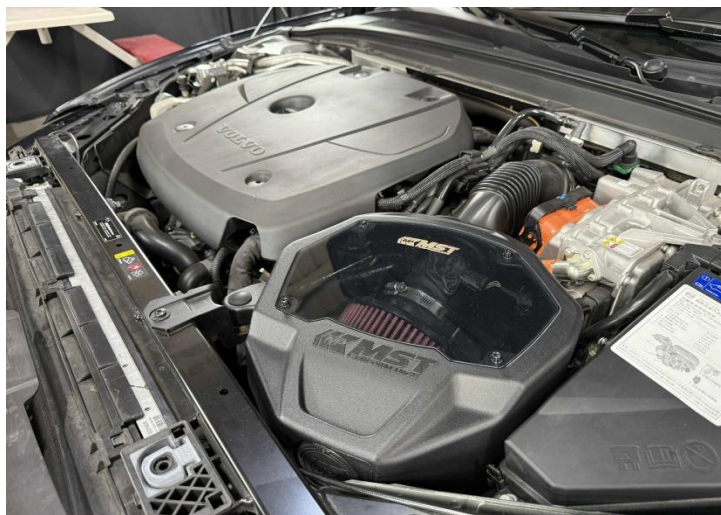
Figure 15: Congratulations! You have just completed the installation of this intake system. Periodically, check the alignment of the intake, normal wear and tear can cause nuts and bolts to come loose.
