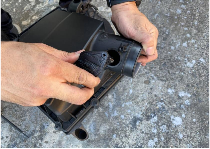
Figure 5: Remove the bolts and MAF sensor from the air box.
