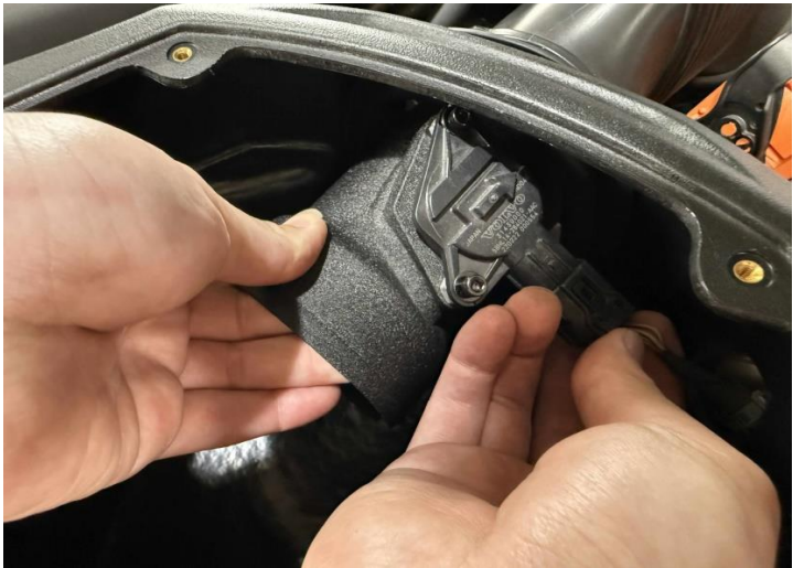
Figure 12: Connect the MAF wire.
