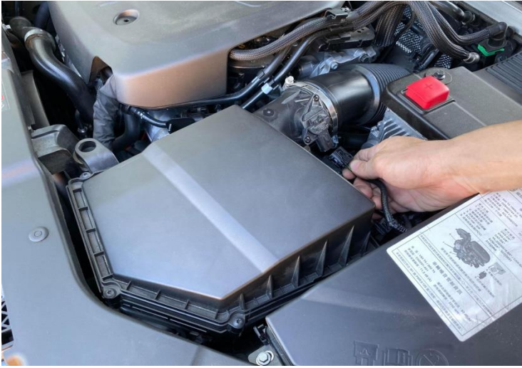
Figure 2: Disconnect the MAF sensor.
