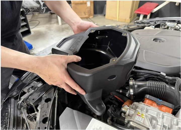
Figure 10: Install the MST heat shield.
