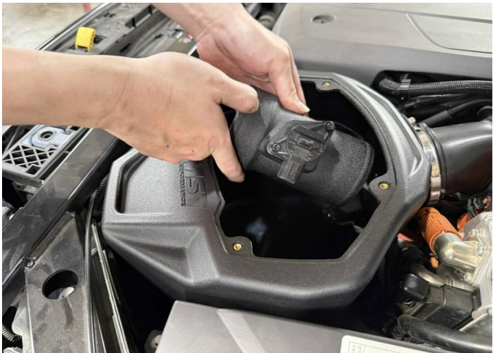
Figure 11: Install the MST tube.
