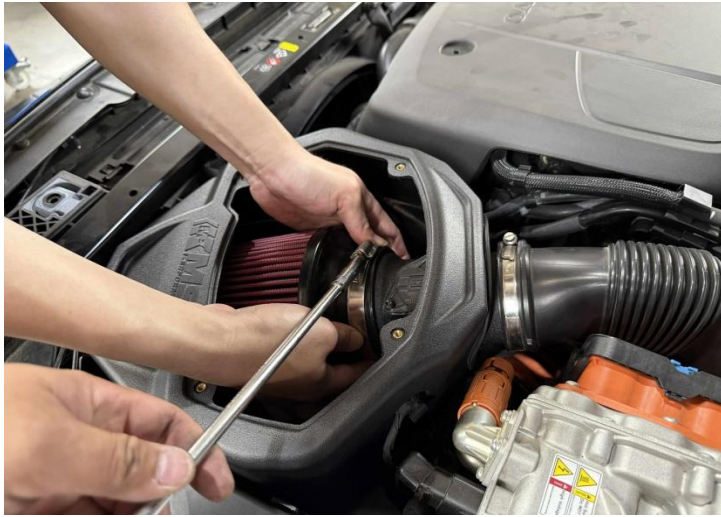
Figure 13: Install the MST filter.
