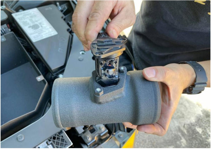
Figure 6: Install the MAF sensor on the MST pipe.
