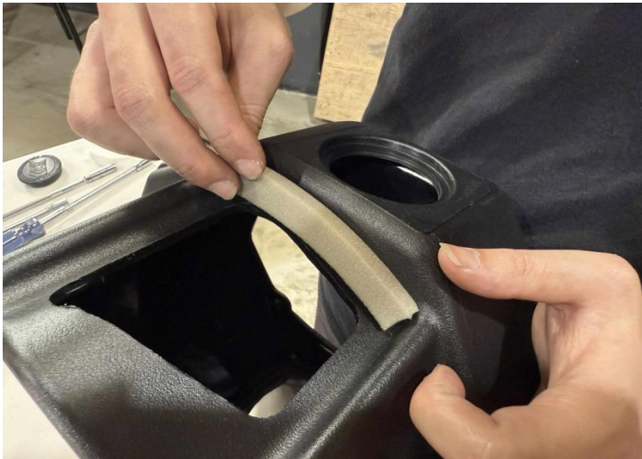
Figure 9: Stick foam on the air box.
