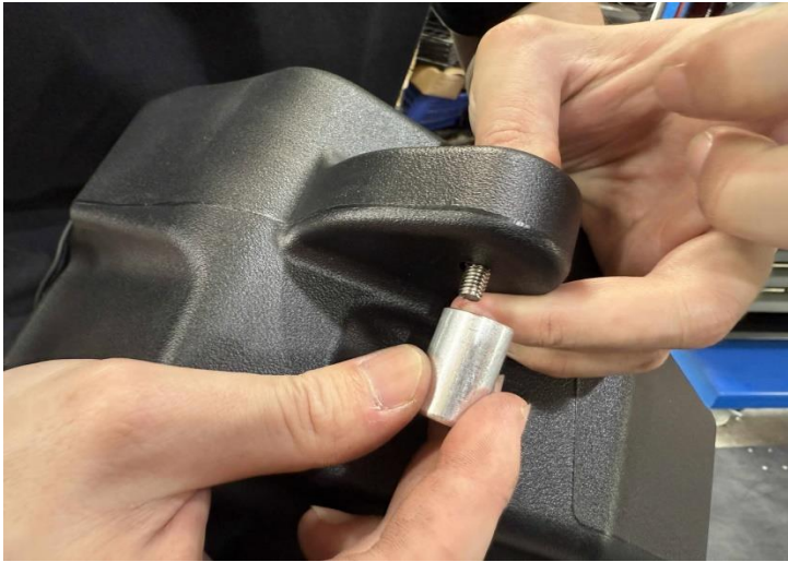
Figure 7: Install the alu-mount on MST heat shield.
