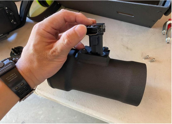
Figure 12: Install the MAF sensor in the MST pipe.
