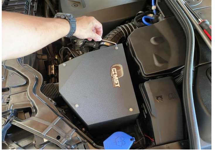
Figure 16: Install the heat shield cover.
