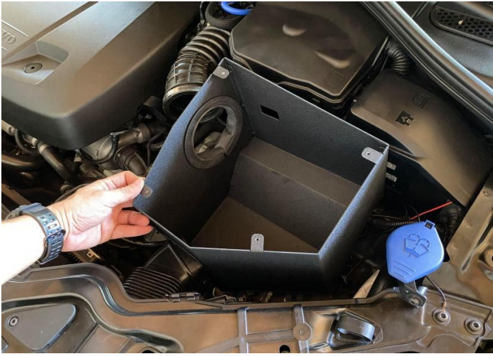
Figure 10: Install the MST heat shield.
