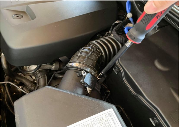
Figure 3: Loosen the hose clamp.
