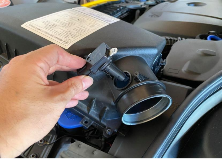
Figure 6: Remove the mass air flow sensor from the stock air box.
