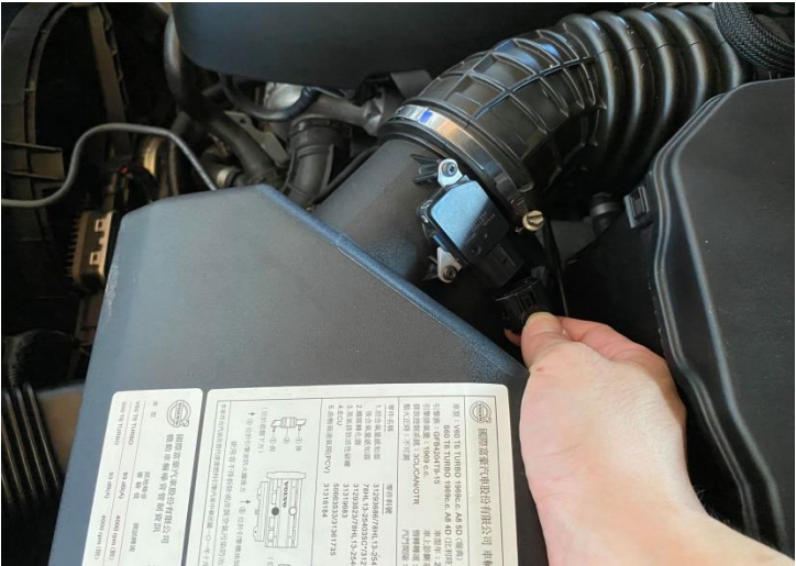
Figure 2: Disconnect the MAF sensor.
