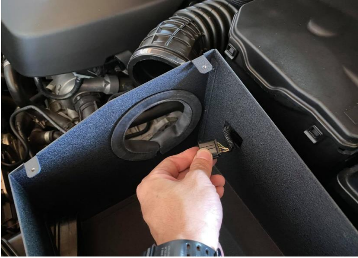
Figure 11: Place the MAF wire through the MST heat shield.
