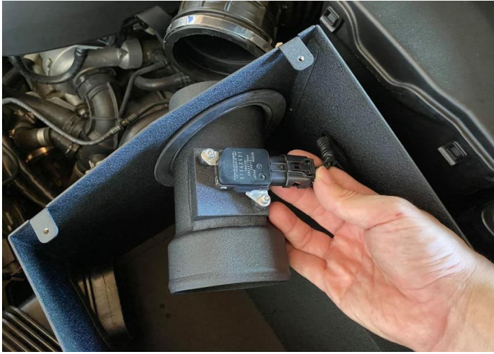
Figure 13: Connect the MAF wire.
