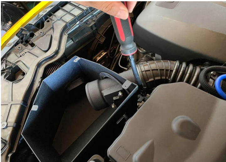
Figure 14: Connect the inlet pipes and tighten the hose clamp.
