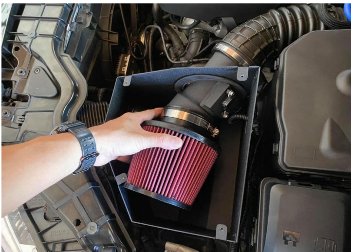
Figure 14: Connect the inlet pipes and tighten the hose clamp.
