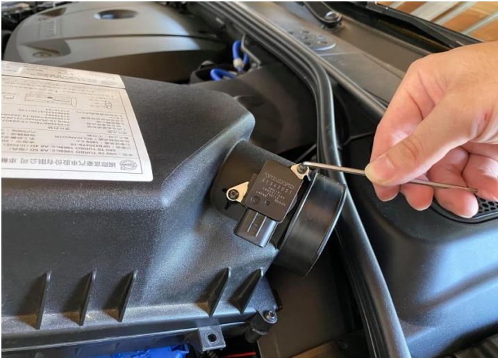
Figure 5: Remove the bolts from the MAF sensor.
