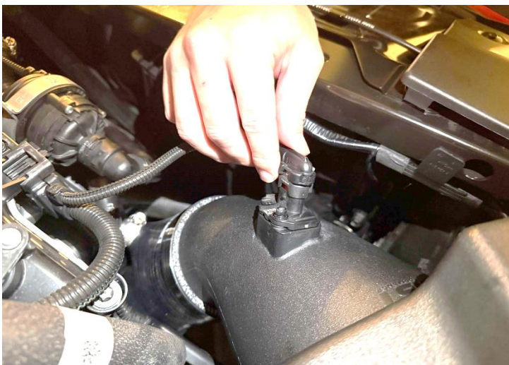
Figure 15: Plug in the mass air flow sensor connector.
