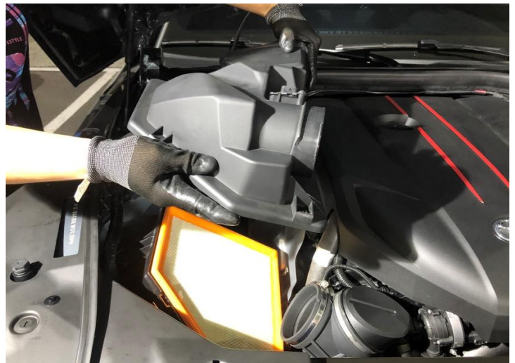
Figure 5: Remove stock air box cover.
