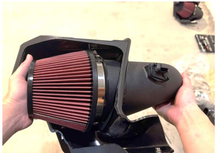
Figure 12: Install the filter, tube and aluminum mount on the air box.
