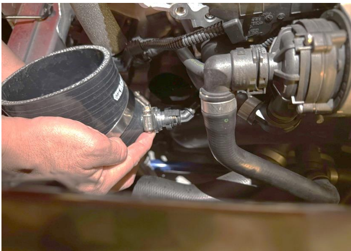
Figure 9: Before installing silicone turbo inlet, please connect the PCV hose first.
