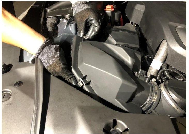
Figure 4: Loosen stock air box cover spring.
