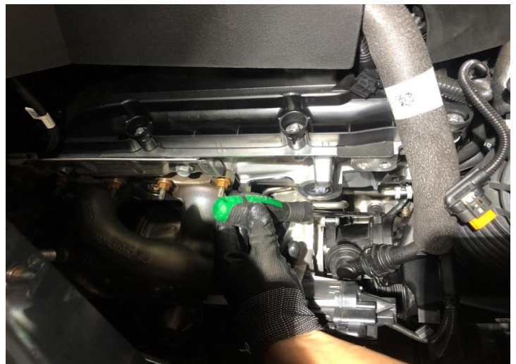
Figure 6: Remove the stock turbo inlet pipe spring.
