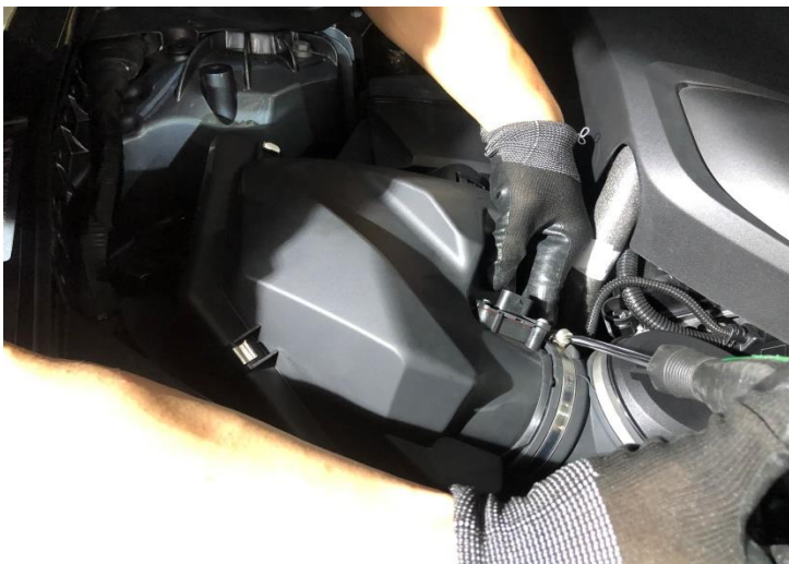
Figure 3: Loosen the hose clamp.
