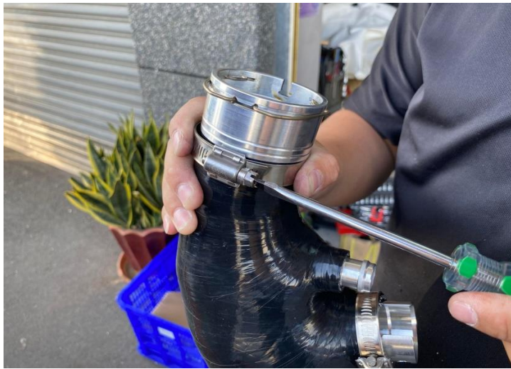
Figure 11: Install the inlet adapter.
