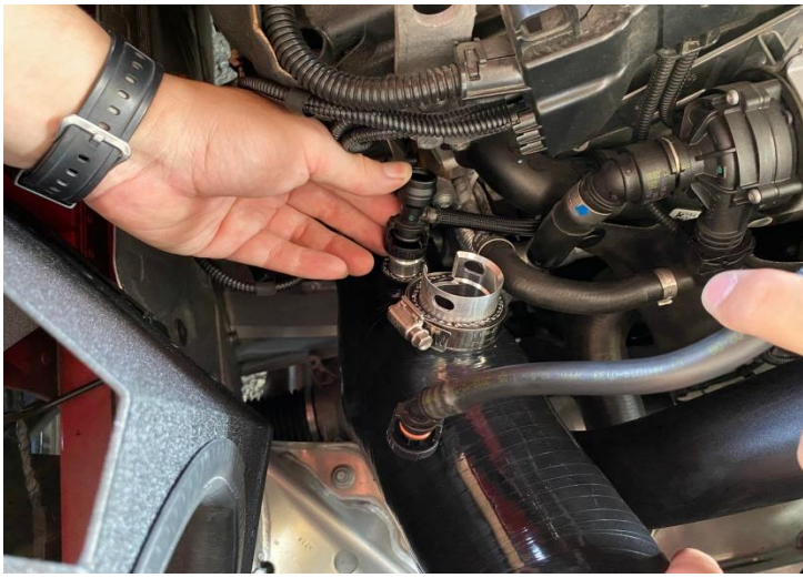
Figure 19: Install the PCV.
