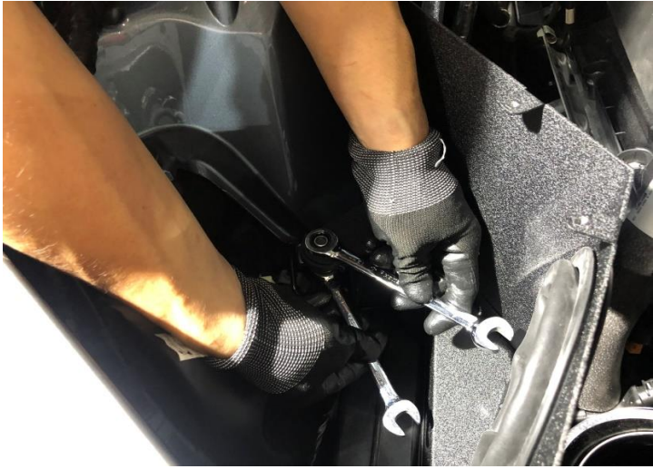
Figure 16: Secure the heat shield breaket with bolt.
