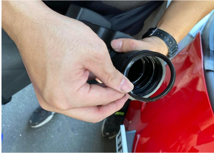
Figure 12: Remove the O-Ring from stock inlet pipe.
