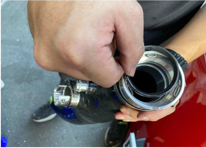
Figure 13: Install the O-Ring on MST adapter.
