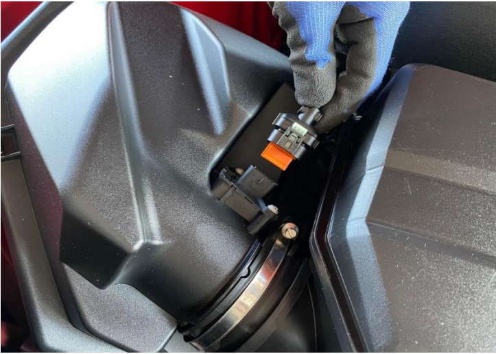
Figure 3: Disconnect the mass air sensor.
