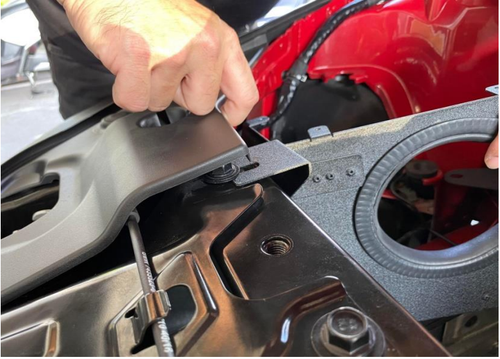
Figure 17: Secure the heat shield breaket with bolt.
