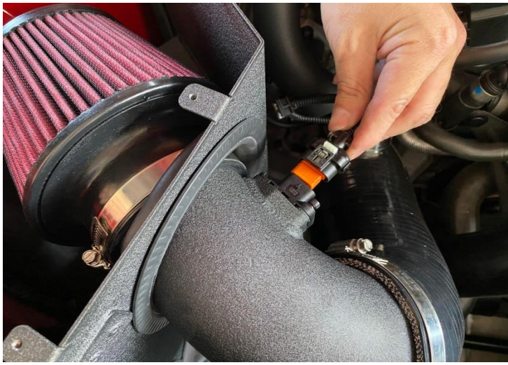
Figure 25: Plug in the mass air flow sensor connector.
