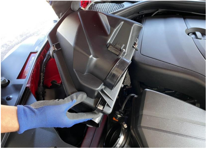
Figure 4: Remove the stock air box.
