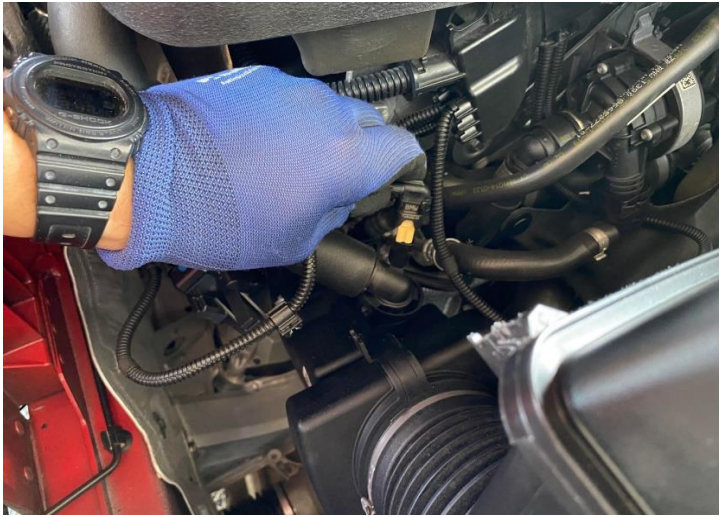
Figure 6: Disconnect the PCV sensor.
