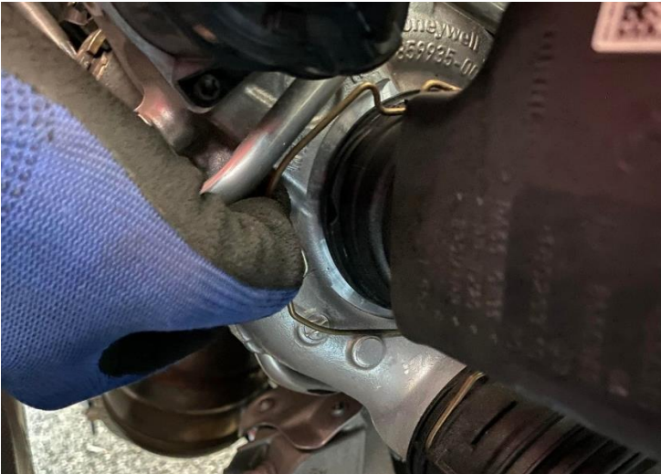
Figure 8: Remove the stock spring on inlet pipe.
