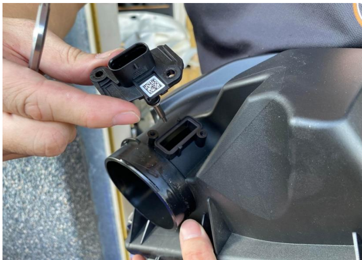
Figure 21: Remove the mass air flow sensor from the stock air box.
