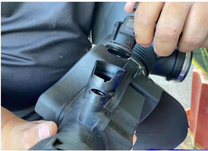
Figure 10: Remove the PCV.
