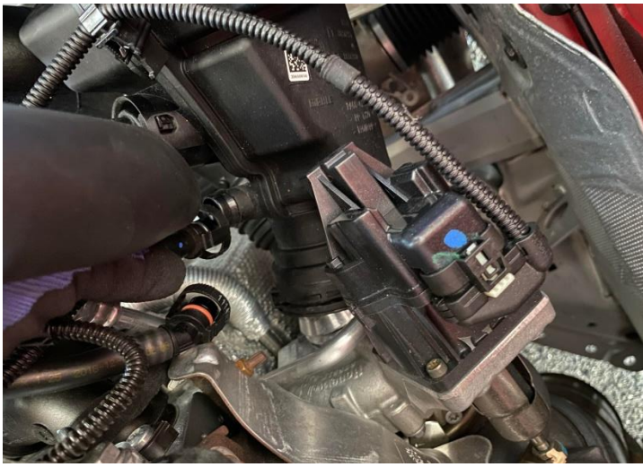
Figure 7: Remove the PCV.
