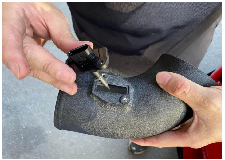
Figure 22: Install mass air sensor on the intake pipe.
