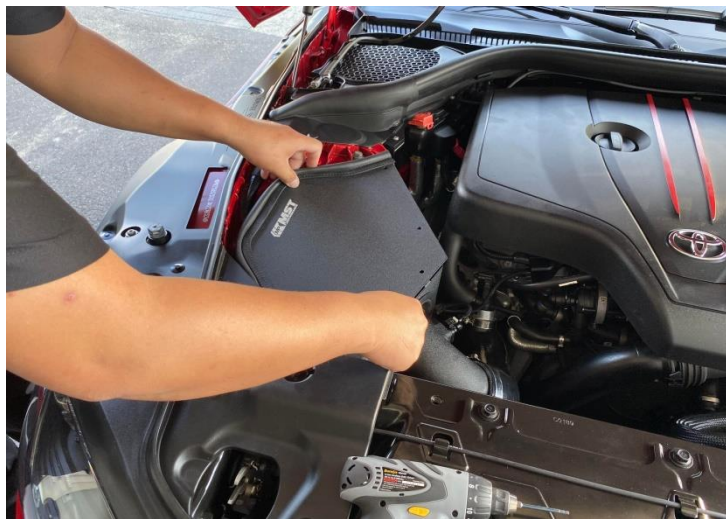
Figure 26: Install the heat shield cover and secure with bolt.
