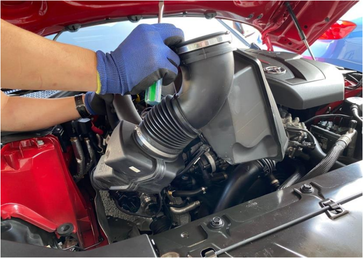
Figure 9: Remove the stock turbo inlet pipe.
