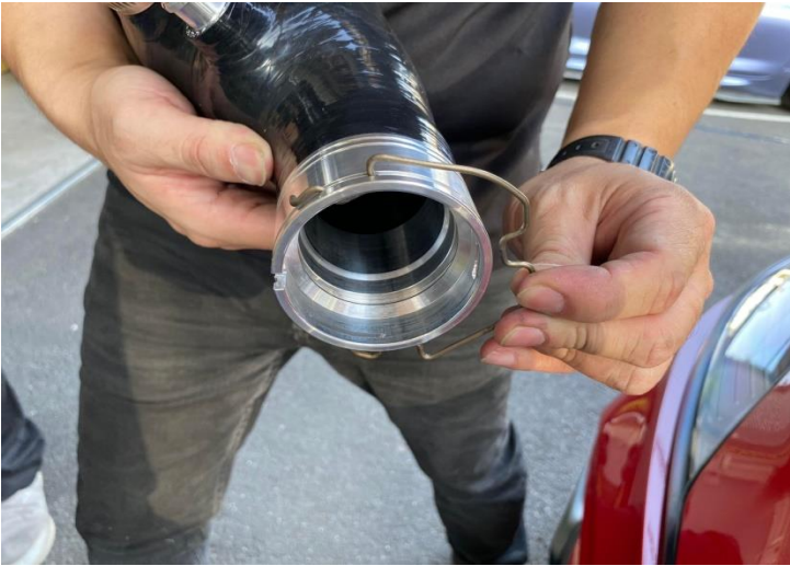
Figure 14: Install the spring.
