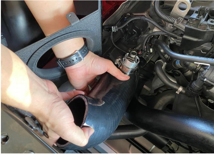
Figure 18: Install the silicone turbo inlet pipe.
