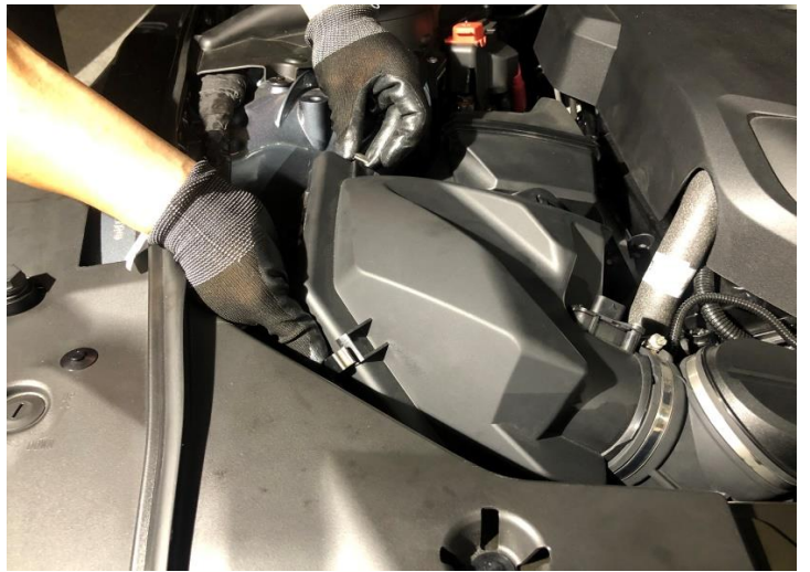
Figure 4: Loosen stock air box cover spring.
