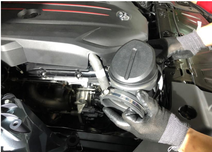
Figure 8: Remove the stock turbo inlet pipe.
