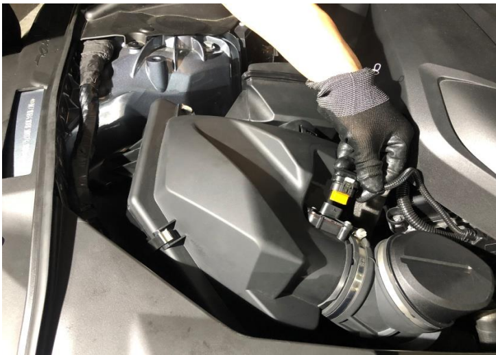
Figure 2: Disconnect the mass air sensor.
