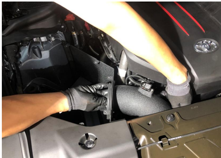
Figure 20: Install the intake pipe.
