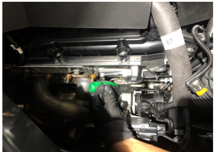
Figure 6: Remove the stock turbo inlet pipe spring.
