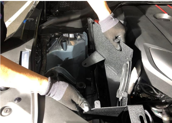
Figure 14: Install the heat shield.
