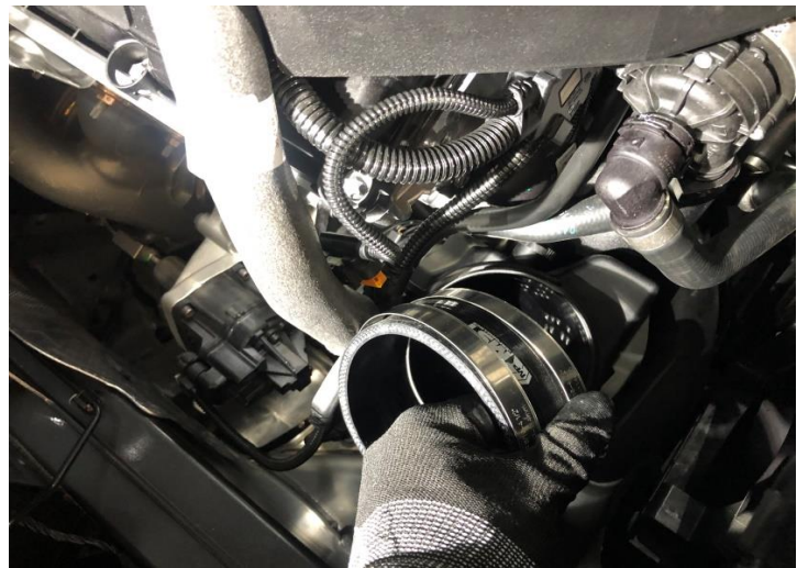
Figure 12: Install the silicone hose.
