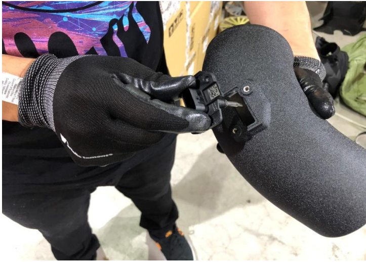
Figure 19: Install mass air sensor into the intake pipe.
