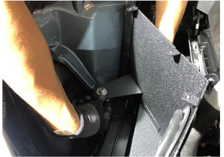
Figure 16: Install the heat shield bracket with bolt.
