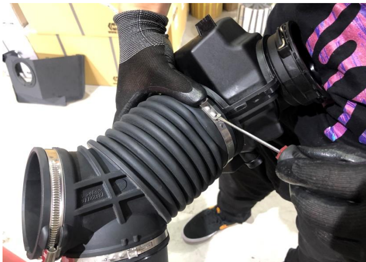
Figure 9: Loosen the hose clamp.
