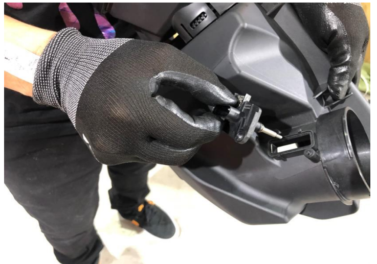
Figure 18: Remove the mass air flow sensor from the stock air box.
