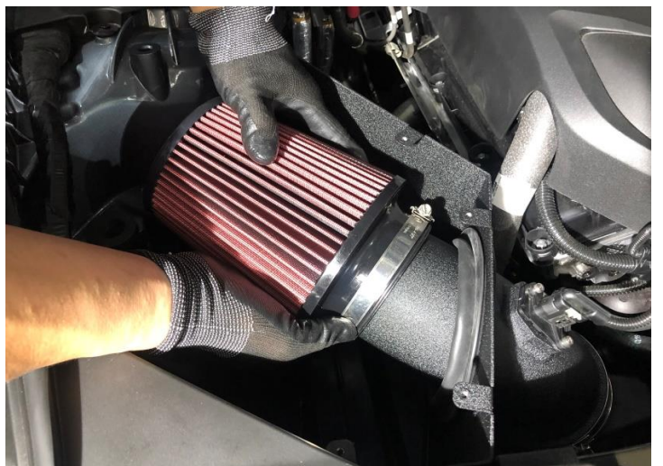
Figure 23: Install the air filter.
