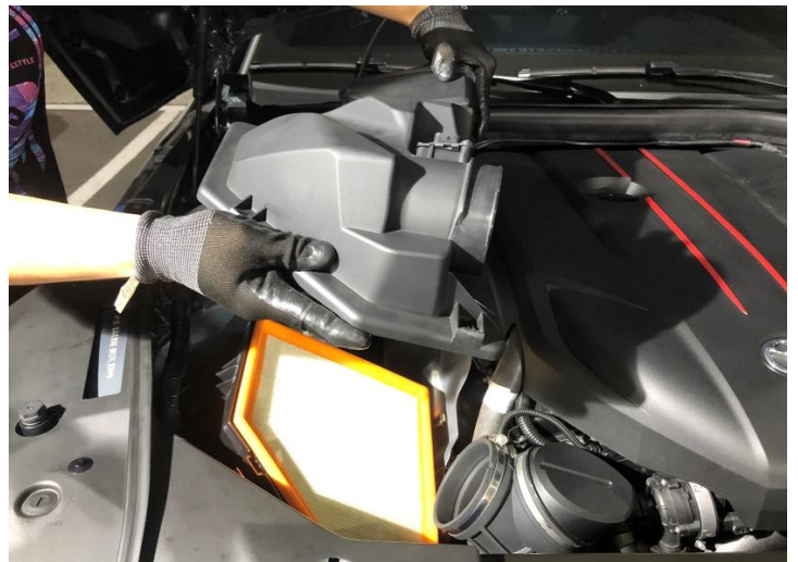
Figure 5: Remove stock air box cover.
