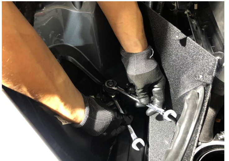
Figure 17: Secure the heat shield bracket with bolt.
