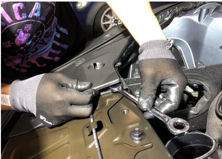
Figure 15: Secure the heat shield bracket with bolt.
