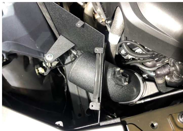
Figure 21: Tighten the hose clamp.
