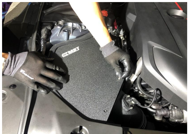
Figure 24: Install the heat shield cover and secure with bolt
