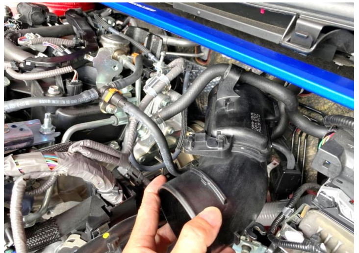
Figure 12: Remove the stock air tube.
