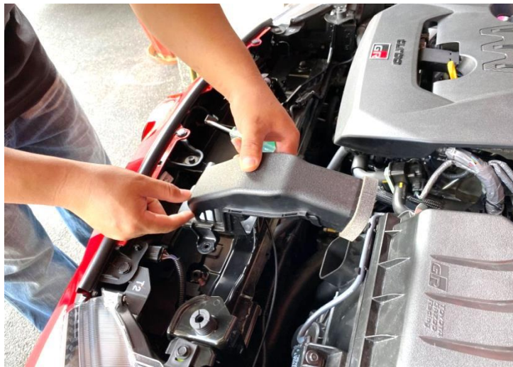
Figure 2: Remove air scoop.
