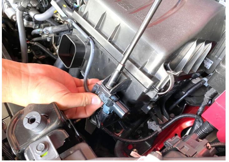
Figure 4: . Remove the vacuum module.
