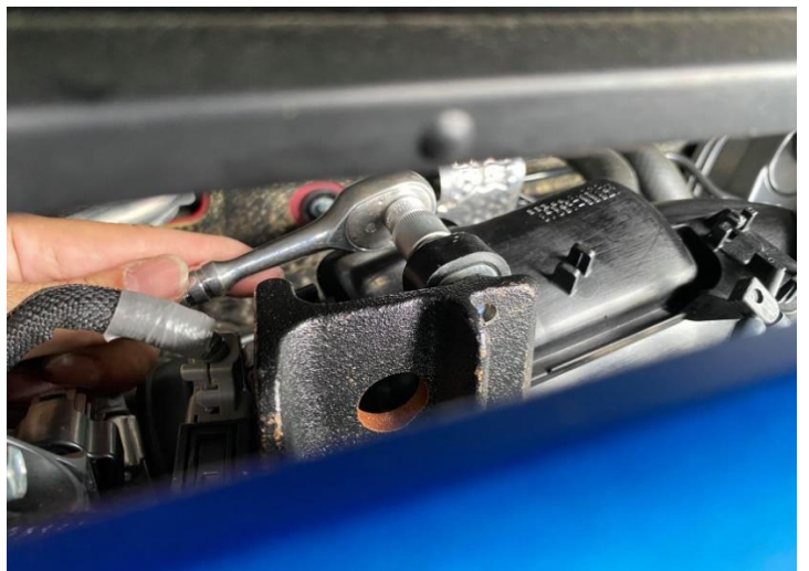
Figure 11: Remove the M8 bolt *2 holding the top of the tube and loosen the hose clamps.
