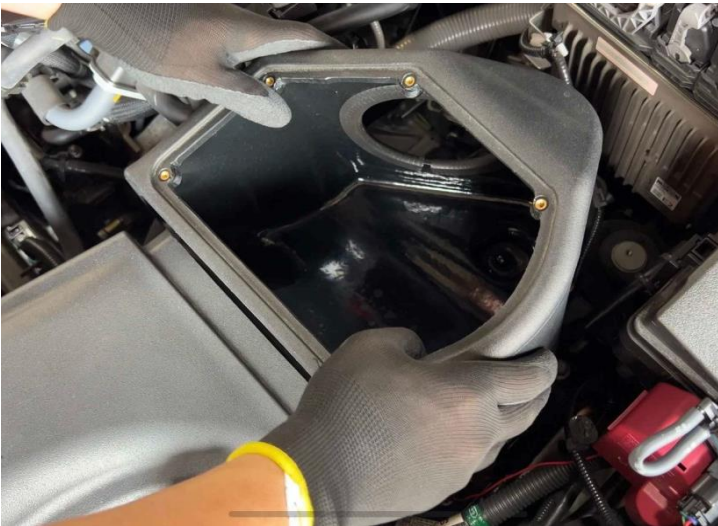
Figure 20: Install the MST air box.
