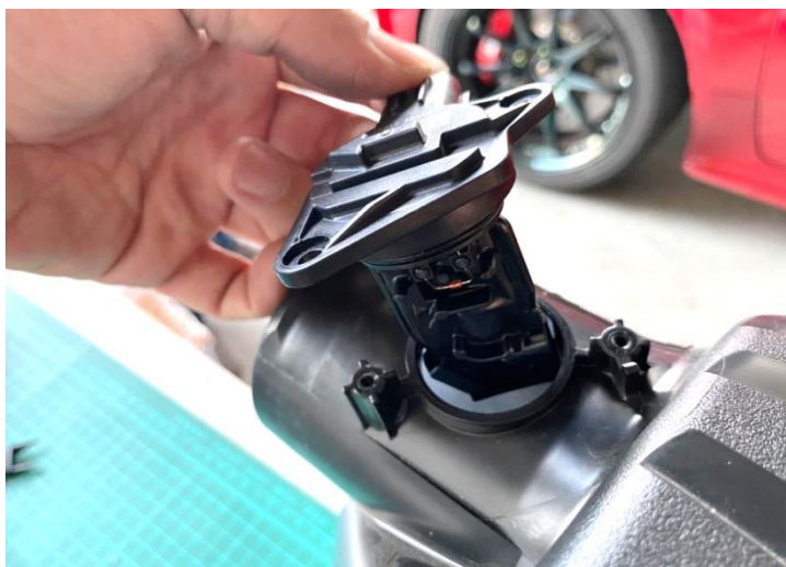
Figure 21: Revome the MAF sensor from stock air box.
