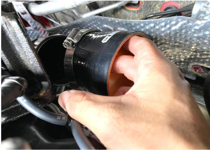
Figure 13: Install the 83-89 silicone hose.
