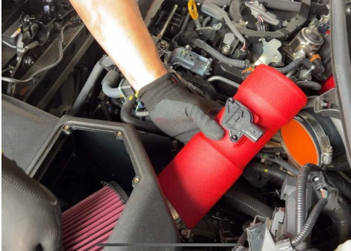
Figure 25: Install the MST tube.
