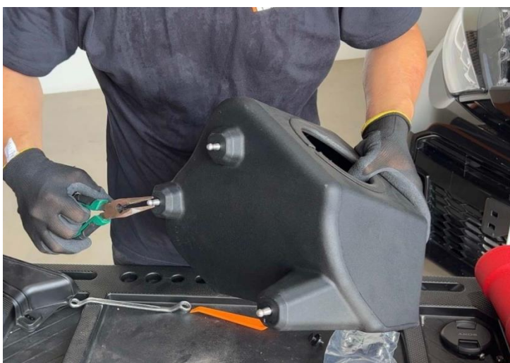
Figure 15: Install aluminum mount on the air box.
