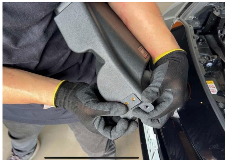
Figure 17: Install the bracket on scoop.
