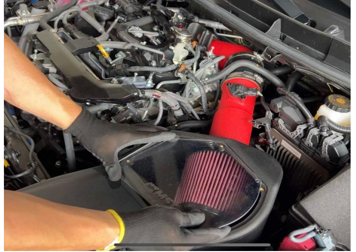
Figure 27: Install the air box cover.
