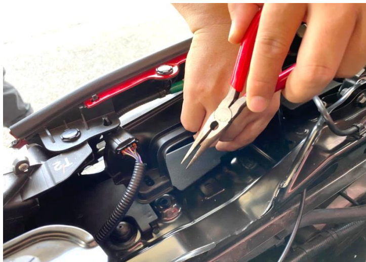
Figure 3: Remove air scoop.
