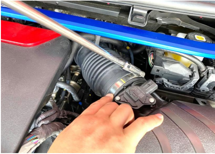
Figure 7: Loosen the stock inlet hose clamp.
