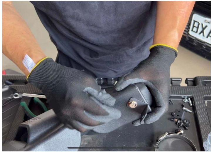
Figure 16: Install the bracket on scoop.
