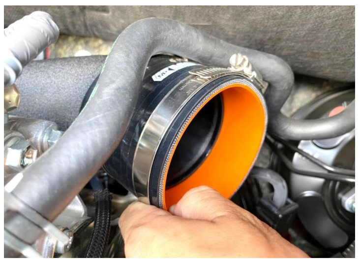
Figure 23: Install the 89-89 15 degree silicone hose.
