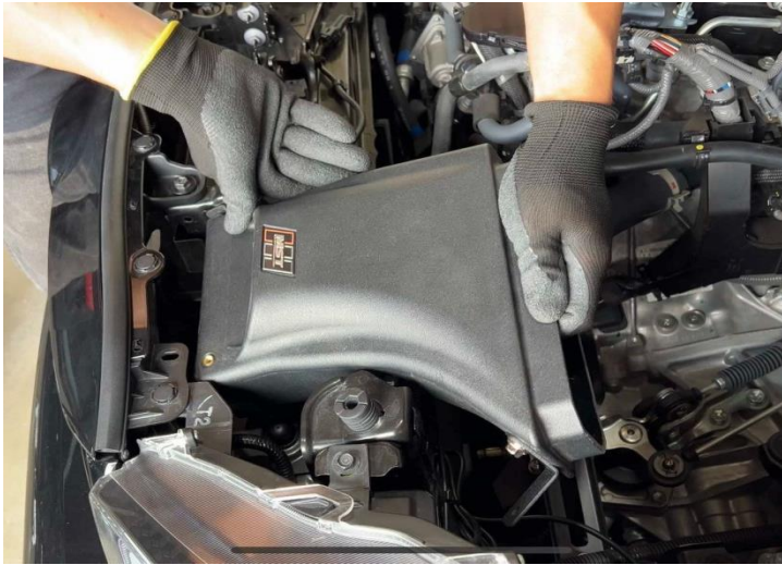
Figure 19: Install the MST scoop and tighten the screw*2.
