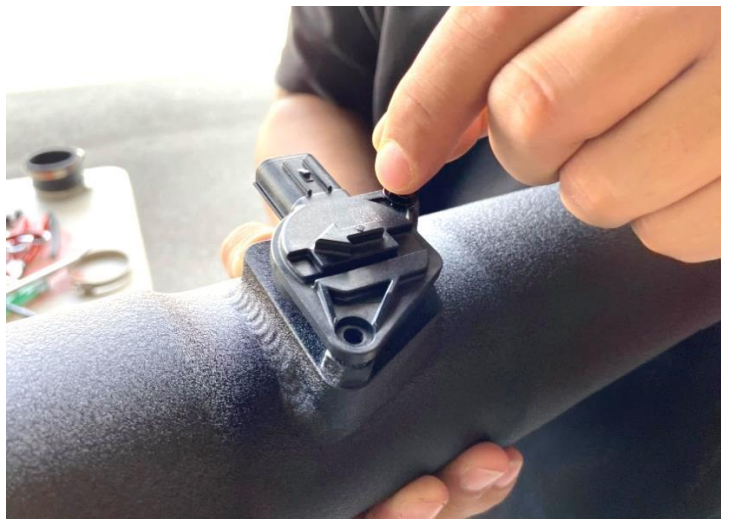
Figure 22: Install the MAF sensor on MST tube.
