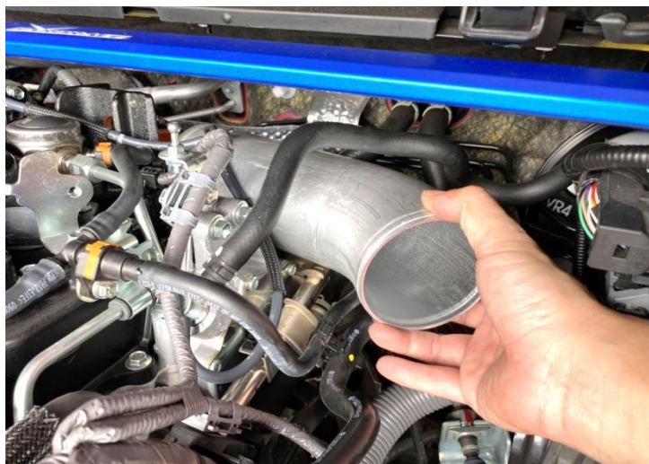
Figure 14: Install the MST tube and Use M8 screw to fix the tube bracket.
