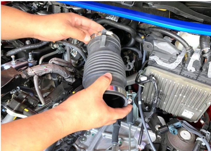
Figure 8: Remove inlet hose.
