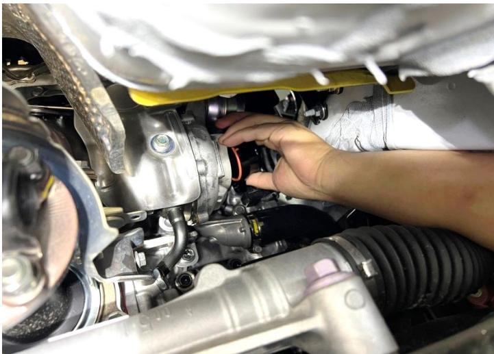
Figure 9: Install the MST inlet adapter on turbo.
