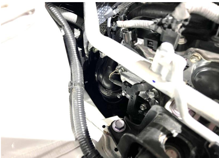
Figure 3: Loosen the stock inlet hose clamp.
