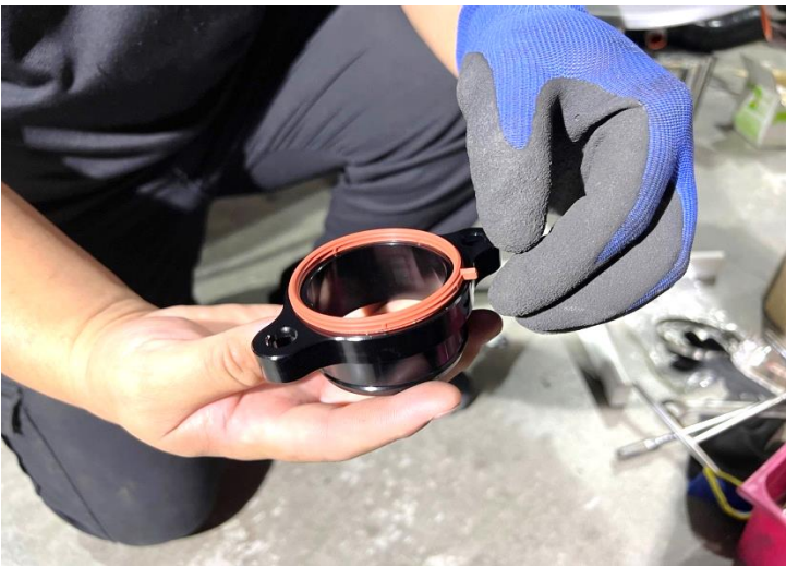
Figure 8: Install the stock o-ring on MST inlet adapter.
