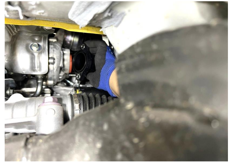
Figure 5: Remove the stock inlet from the turbo.
