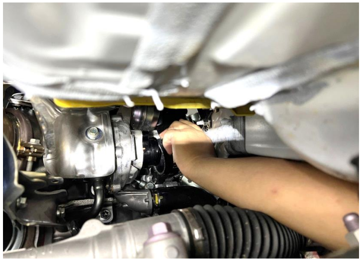
Figure 11: Install the MST silicone hose and 2 clamps.
