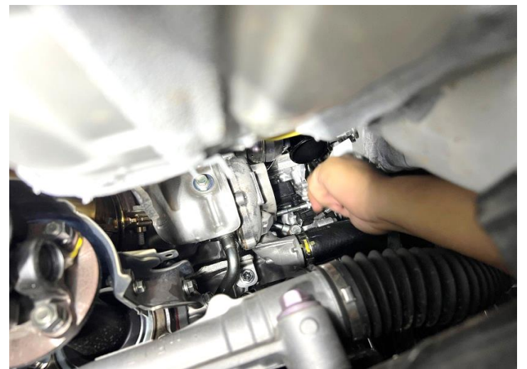
Figure 6: Remove the 10mm bolt from turbo.
