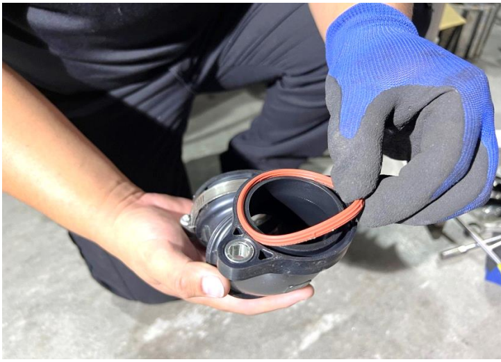
Figure 7: Remove the stock o-ring from stock inlet.
