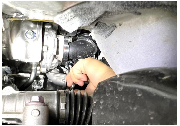
Figure 4: . Remove the 12mm nut X 2
