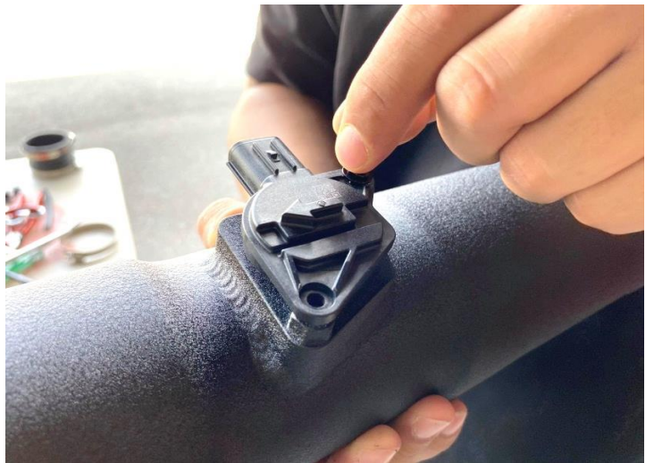
Figure 22: Install the MAF sensor on MST tube.
