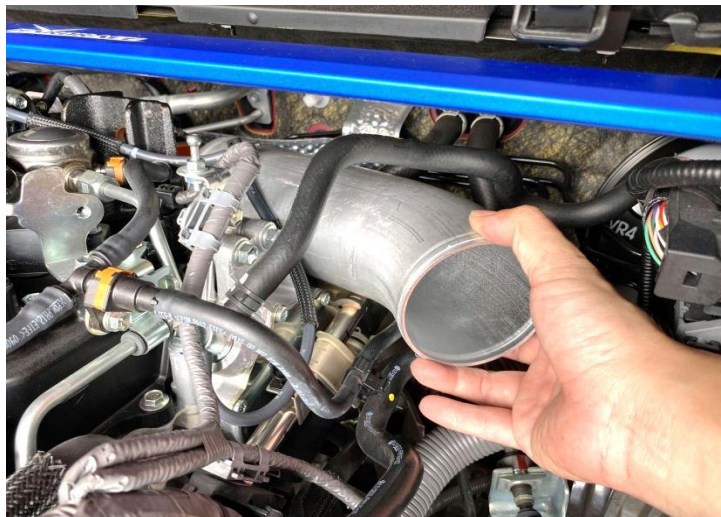
Figure 14: Install the MST tube and tight the clamps.
