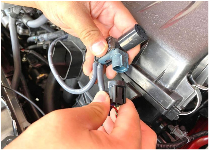
Figure 5: Unplug the module on the airbus and pull the vacuum line off the module on the airbox.
