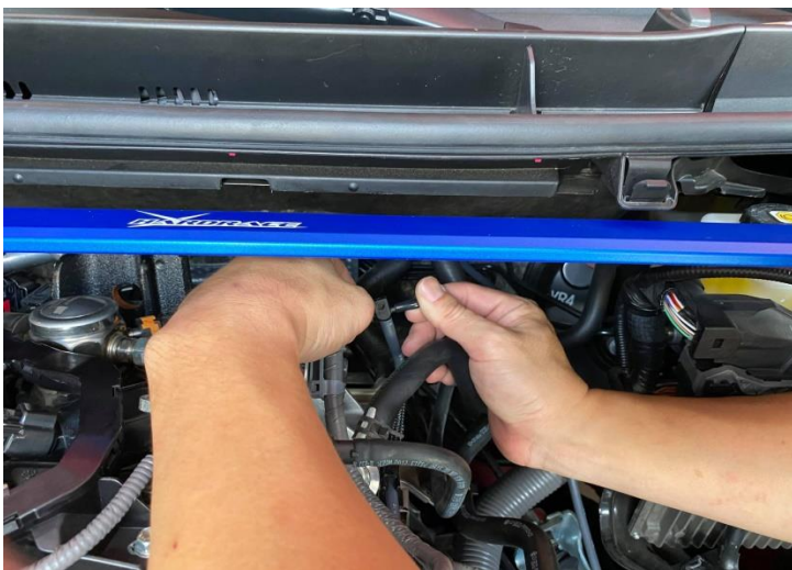
Figure 9: Disconnect the vacuum line from the T-Piece on top of the rear tube and remove the vacuum module from the engine bay.
