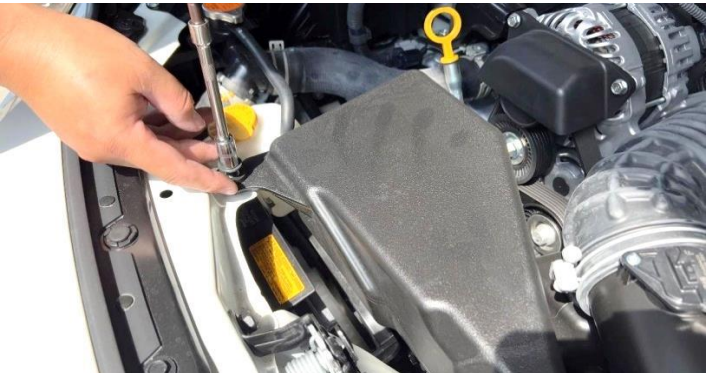
Figure 5: Remove the stock air box bolts x 3
