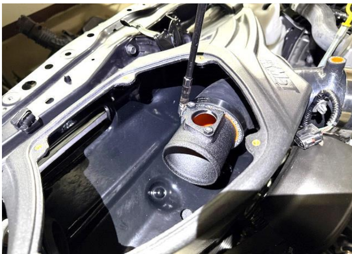
Figure 20: Install the MAF tube.
