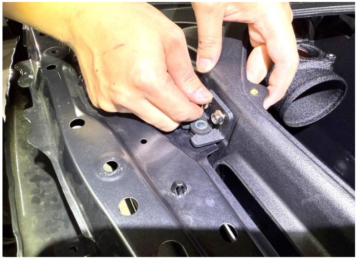
Figure 22: Install the bracket on the MST air box and use OEM bolt and rubber to tighten the MST air box.
