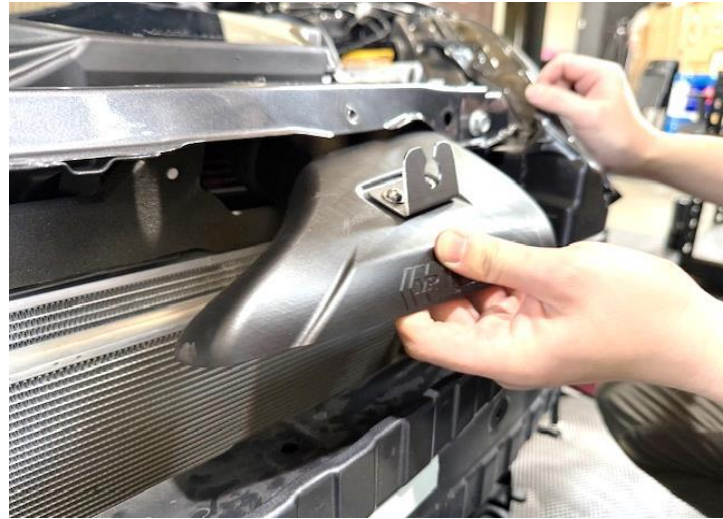
Figure 30: Install the MST air scoop. Note: Greedy and Big Mouth air scoops do not match the MST Intake and may cause the engine to stall.
