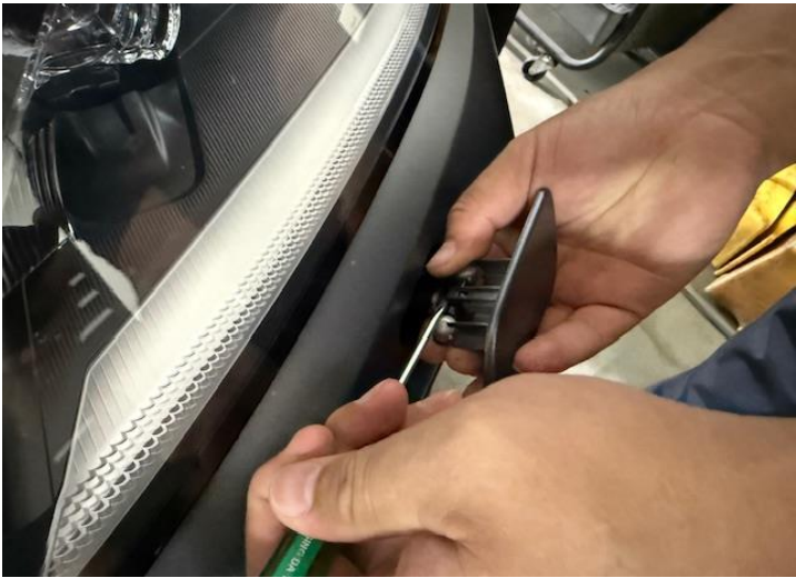
Figure 10: Remove the headlight washers cover.
