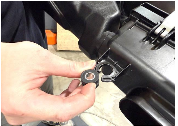
Figure 16: Remove the rubber *3 from stock air box and stock snorkel rubber *1
