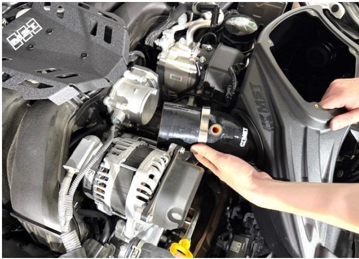
Figure 19: First install the intake silicone hose into the air box.
