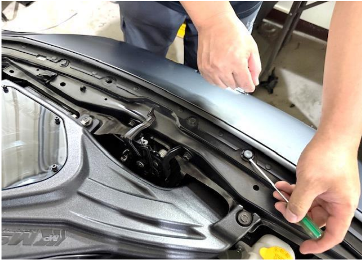
Figure 7: Remove the bolts * 5 and clips * 2.
