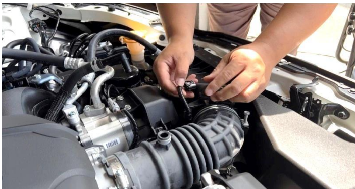
Figure 3: Disconnect the mass air sensor.
