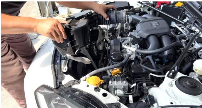
Figure 6: Remove stock air box from the vehicle.
