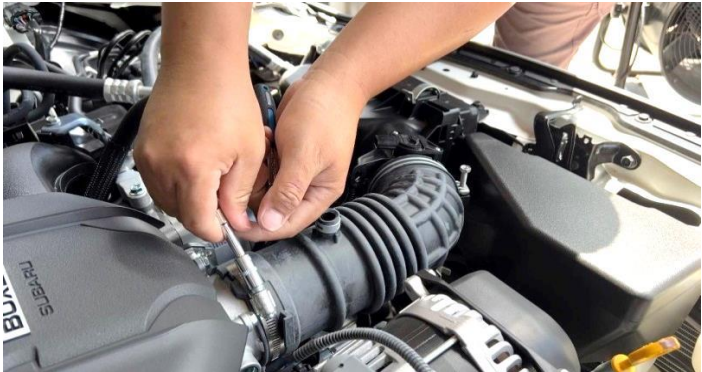
Figure 4: Loosen the hose clamp securing the intake hose to the throttle body.
