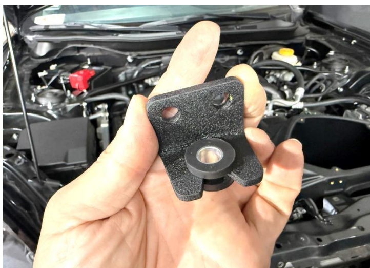
Figure 21: Install rubber on MST air box bracket.
