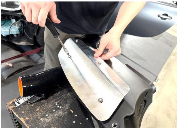
Figure 18: Install the heat shield under the MST air box.
