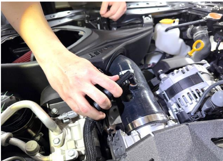
Figure 27: Connect the crank case vent.
