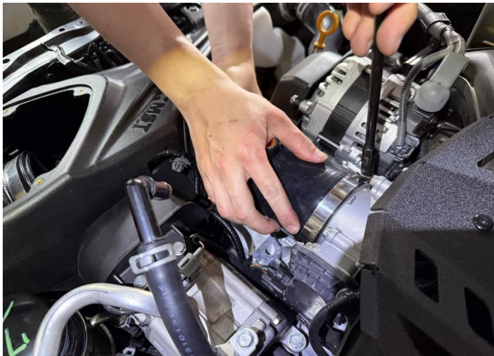
Figure 26: Silicone intake hose tighten into the throttle body.
