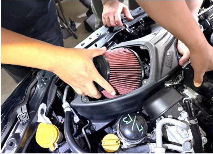
Figure 25: Install the air filter.
