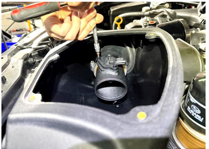
Figure 23: Install the MAF sensor on the tube and connect the sensor.
