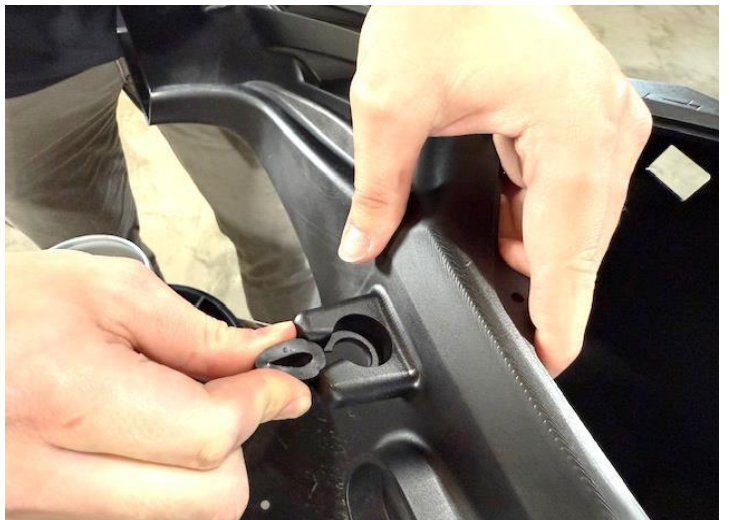
Figure 17: Install the MST rubber *2 on the MST air box .
