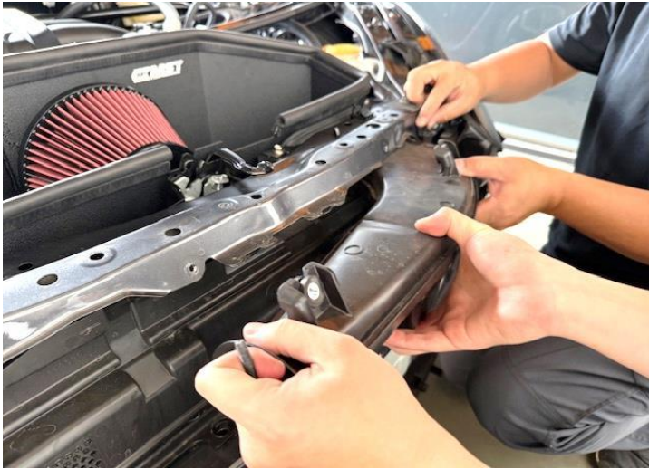
Figure 12: . Remove the bolts *2 and stock snorkel.
