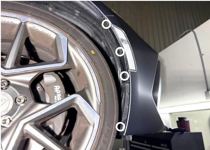
Figure 8: Remove clips * 8 left and right.
