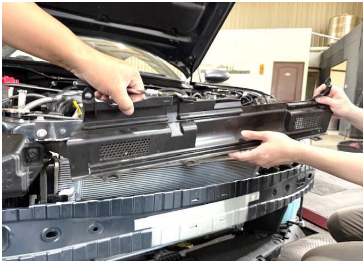
Figure 13: Remove the clips * 6 and plastic shroud.
