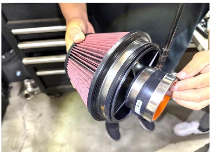
Figure 24: Install velocity stack and silicone hose on the air filter.
