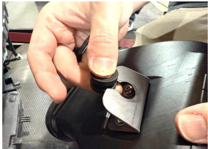
Figure 29: Install bracket and rubber on the MST air scoop.
