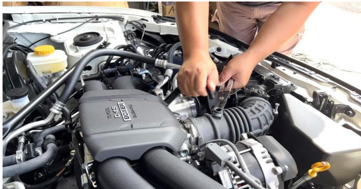
Figure 2: Release the spring clamp and then disconnect the crank case vent hose from the fitting.
