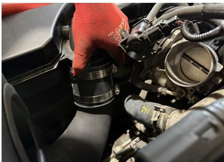
步驟 18: 鎖緊導風口矽膠
