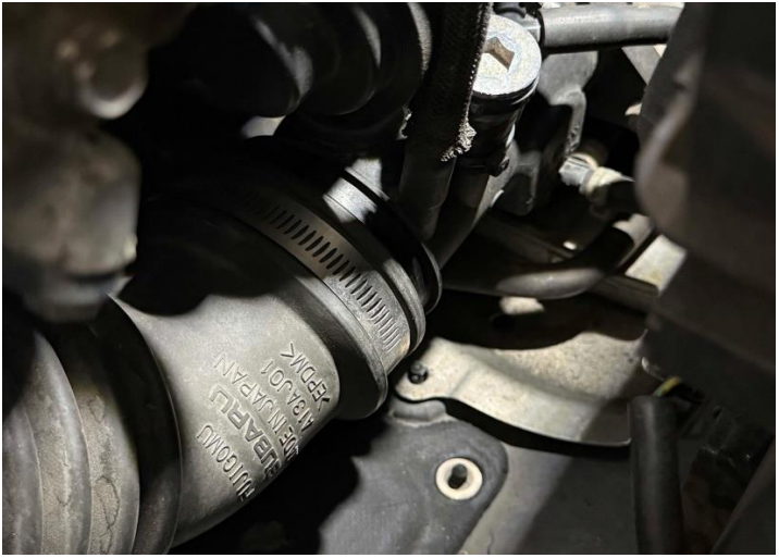
Figure 10: Loseen the clamp on the turbo inlet.
