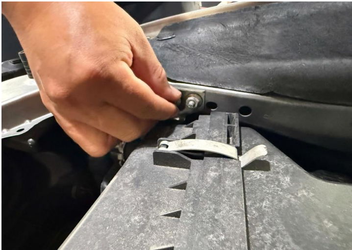
Figure 3: Remove the bolts from stock air box bracket.
