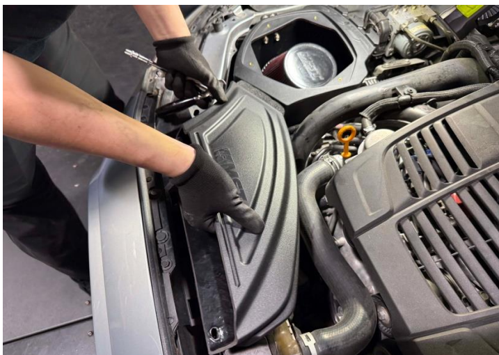
Figure 27: Install the MST air scoop.
