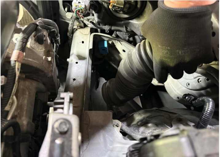
Figure 8: Loseen the stock tube clamp and rubber mount.
