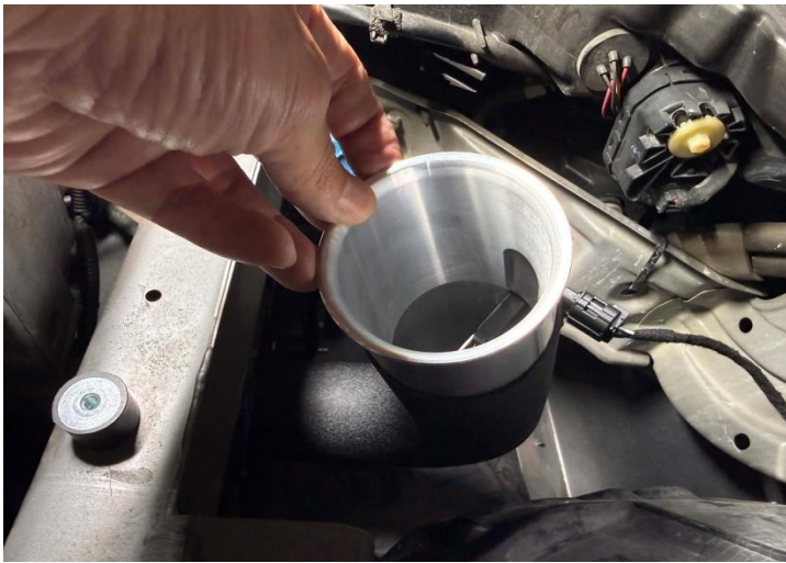
Figure 20: A sleeve is install inside the MST tube.
