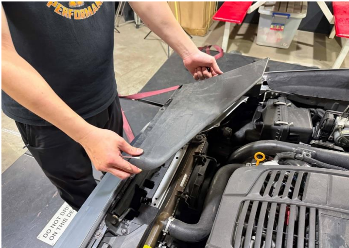
Figure 2: Revome the air scoop.
