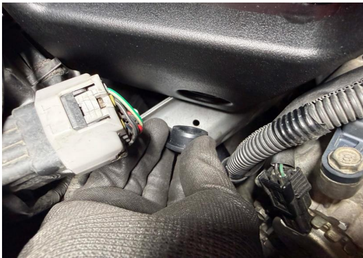
Figure 26: Install the rubber plug to seal the service access hole.
