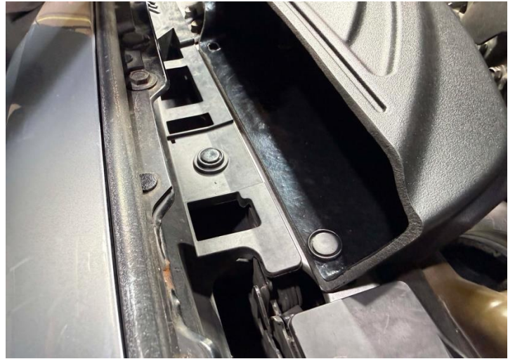
Figure 28: Install the air scoop retaining clips.
