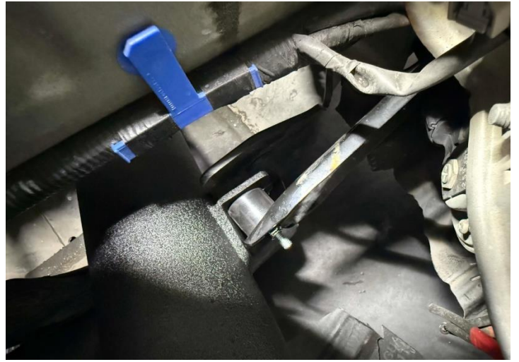
Figure 16: Tighten the MST tube onto the rubber mount.
