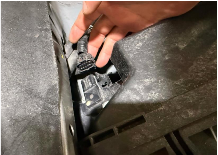
Figure 5: Disconnect the MAF sensor.
