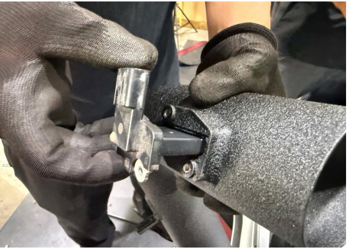
Figure 12: . Install the stock MAF sensor on the MST tube.
