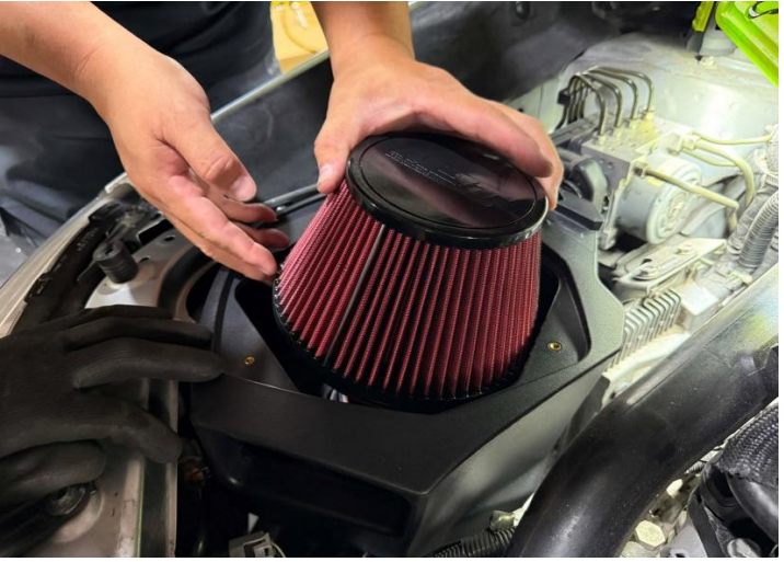
Figure 24: Install the MST filter.
