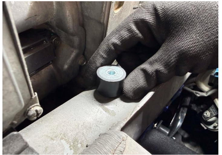
Figure 17: Install the rubber mount onto the vehicle body.
