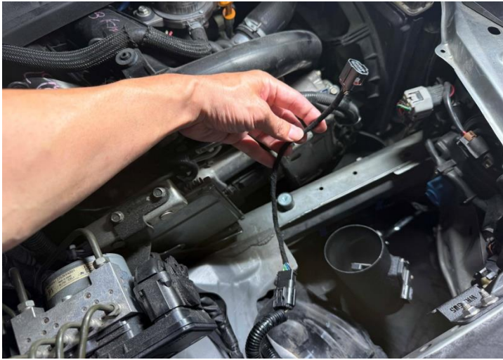
Figure 19: Connect the extension harness and connect the MAF.
