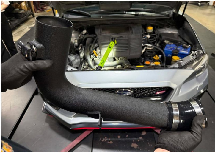
Figure 13: Install the silicone hose onto the MST tube, ensuring it is oriented at the correct angle.
