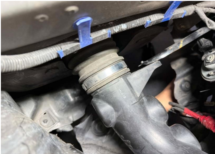
Figure 8: Loseen the stock tube clamp and rubber mount.
