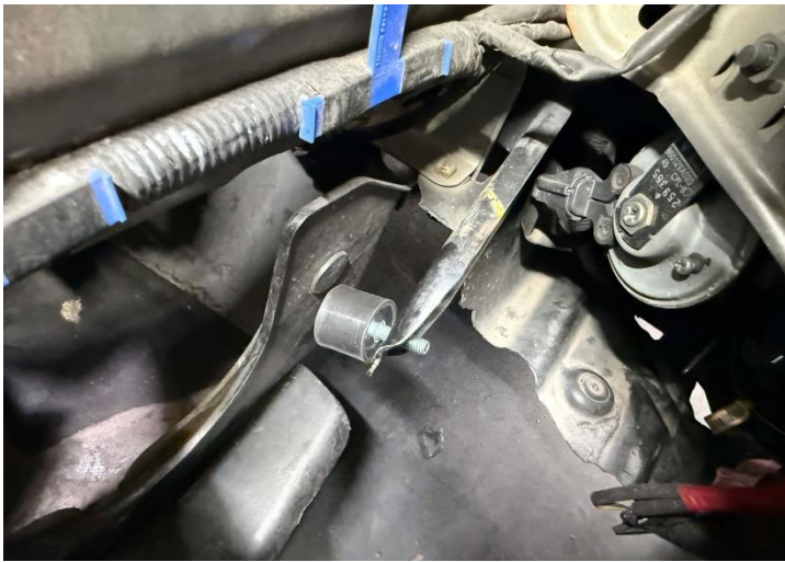
Figure 14: Install the rubber mount onto the bracket.
