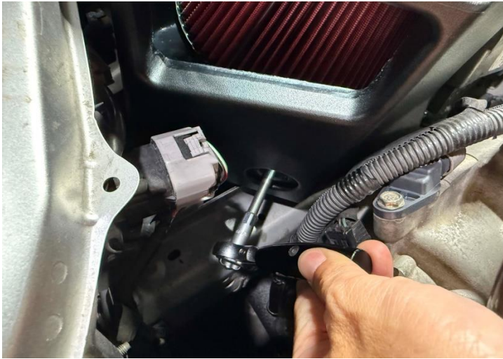
Figure 25: Tighten the air filter clamp through the service access hole in the MST air box.
