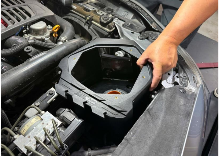
Figure 22: Install the MST air box.
