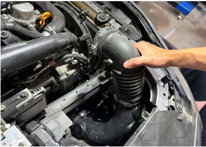
Figure 9: Remove the stock intake tube.
