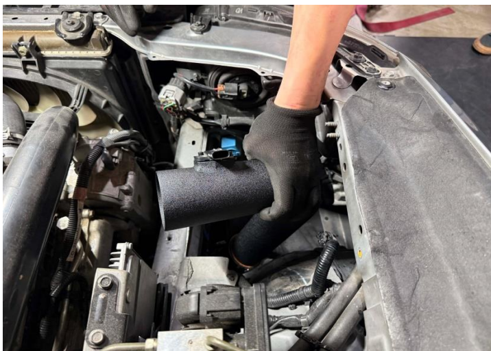
Figure 15: Install the MST tube and connect it to the turbo inlet. Tighten the hose clamp.
