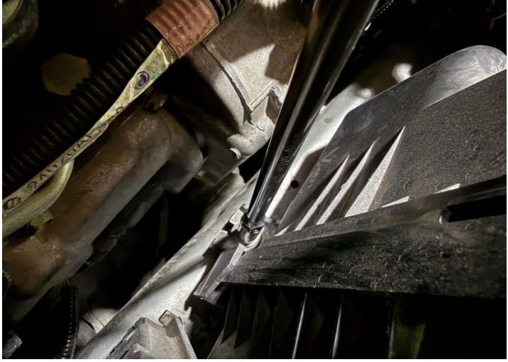
Figure 4: Remove the bolt from stock air box.
