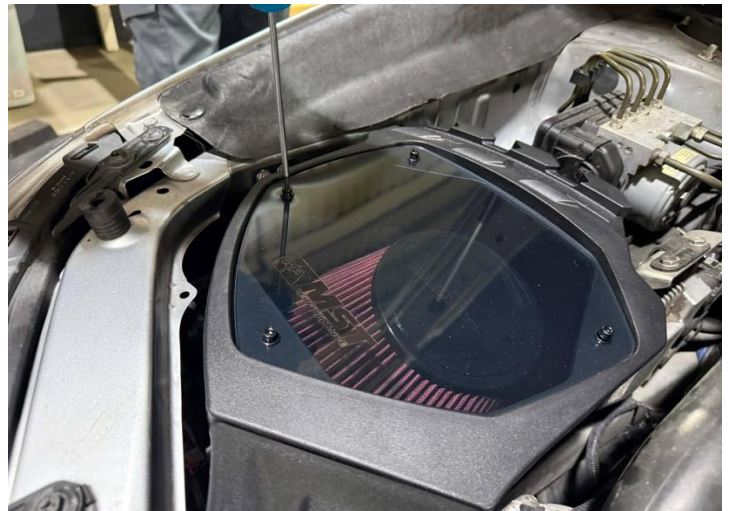
Figure 29: Install the air box cover and tighten the M4 bolts.
