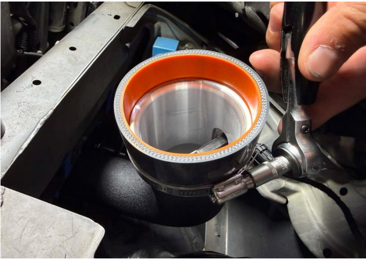
Figure 21: Install the silicone hose onto the MST tube
