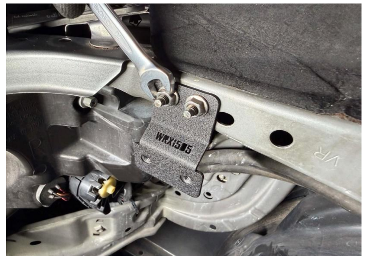
Figure 18: Install the MST air box bracket onto the vehicle body.
