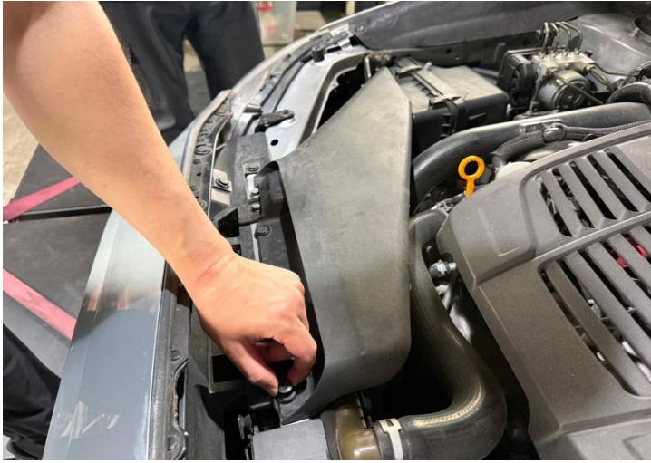
Figure 1: Remove the air scoop retaining clips.
