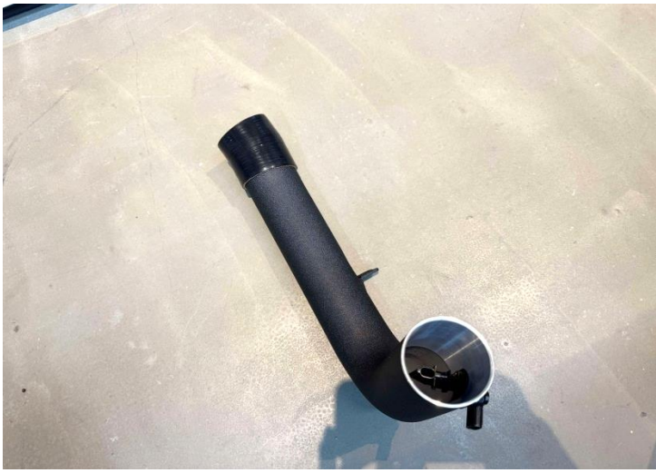
Figure 19: Install the 76-76 15 degree silicone hose into intake tube (Turbo side).
