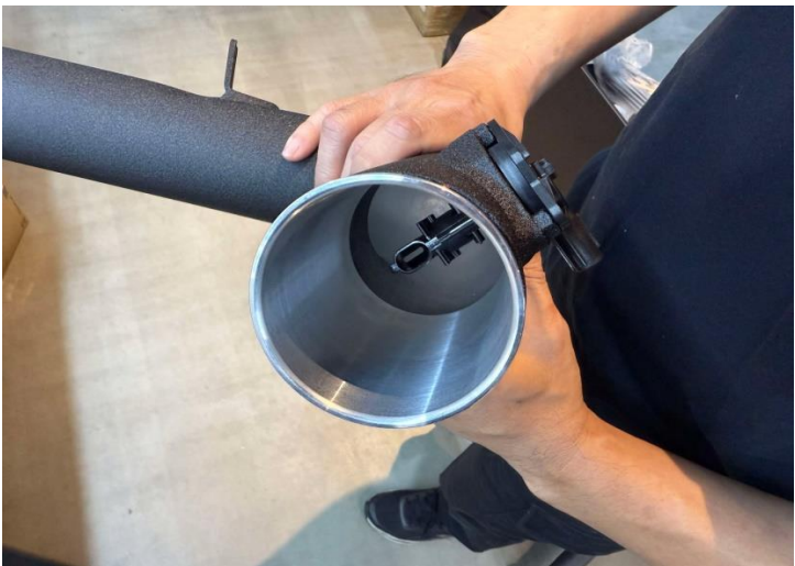
Figure 17: NO TUNING MUST INSTALL MAF SLEEVE!
