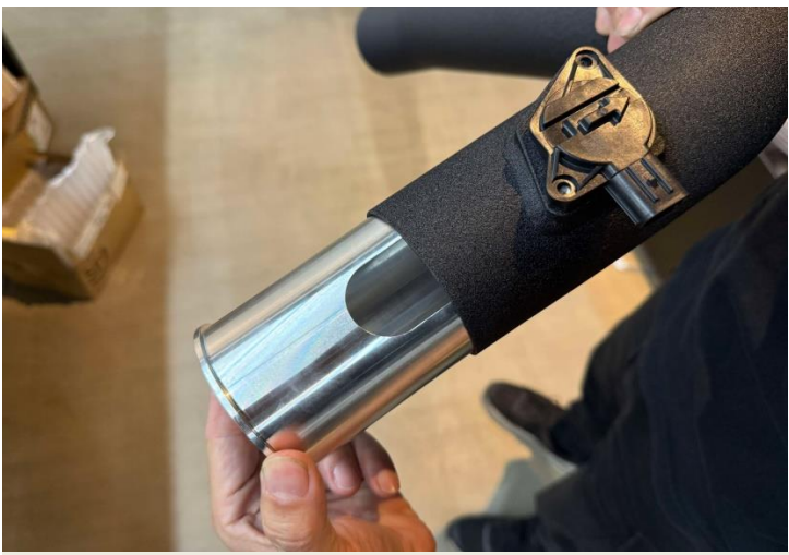
Figure 16: NOTE!! If your vehicle does not have TUNE and REMAP, please install MAF sleeve. No Tuning required in most cases using supplied MAF Sleeve
