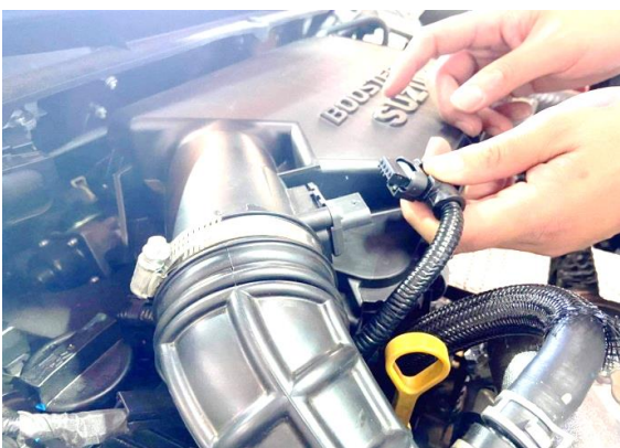
Figure 4. Disconnect the mass air sensor.
