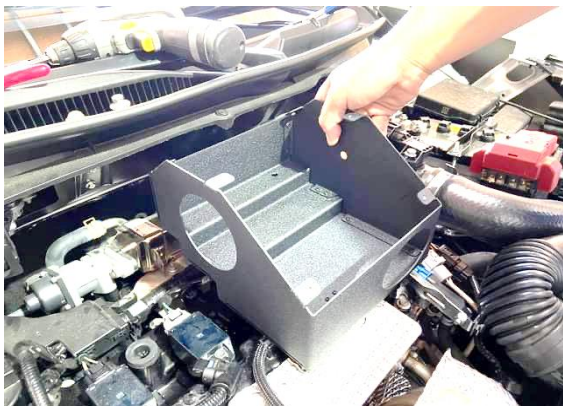
Figure 11. Install the heatshield.
