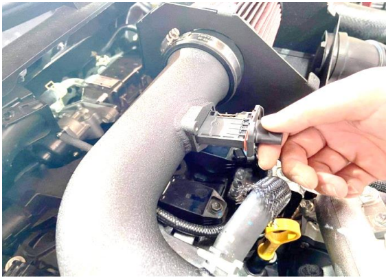
Figure 17. Install the MAF sensor.
