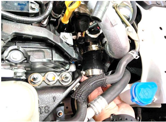
Figure14. Install the 45-57mm hose on turbo.
