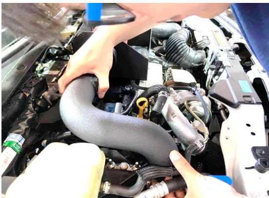
Figure 15. Install the MST tube.
