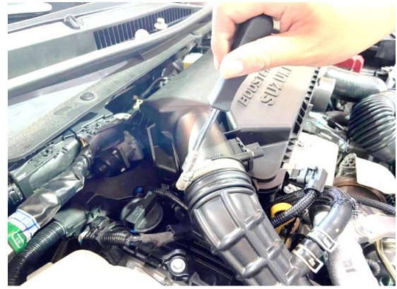
Figure 5. Loose the clamp.
