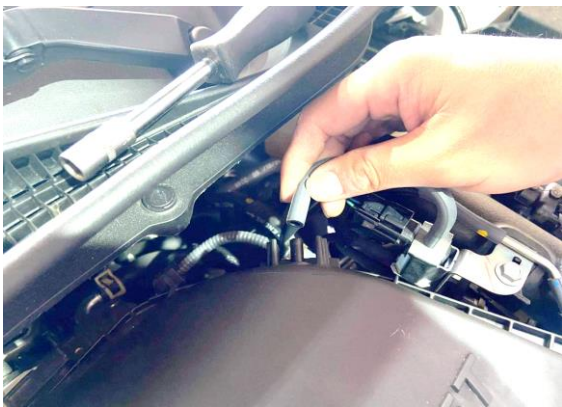
Figure 3. Remove pressure hose.
