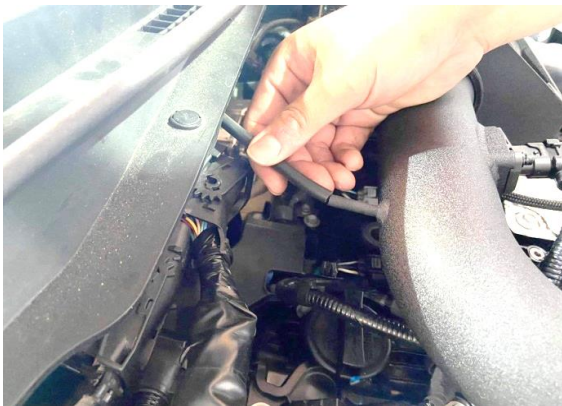
Figure 19. Install the pressure hose.
