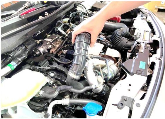
Figure 9. Remove the stock inlet tube.
