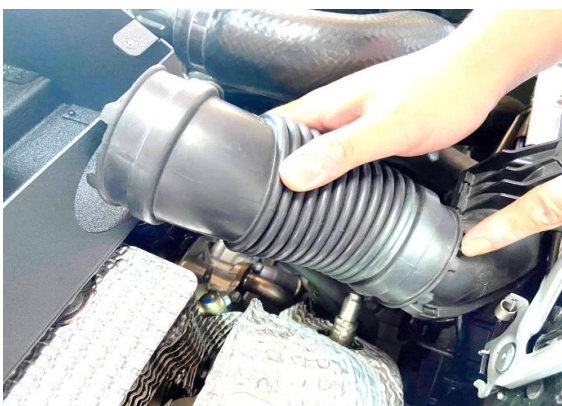
Figure 20. Rotate the inlet hose.
