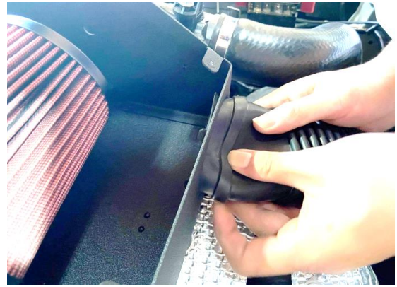
Figure 21. Install the inlet hose at heatshield.
