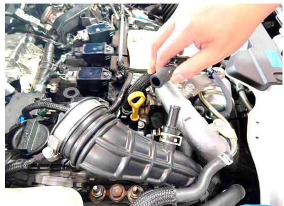
Figure 7. Remove the PCV.
