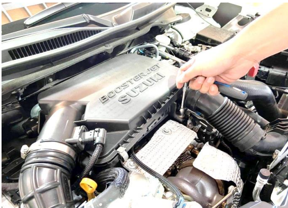
Figure 2. Remove the stock air box bolts.
