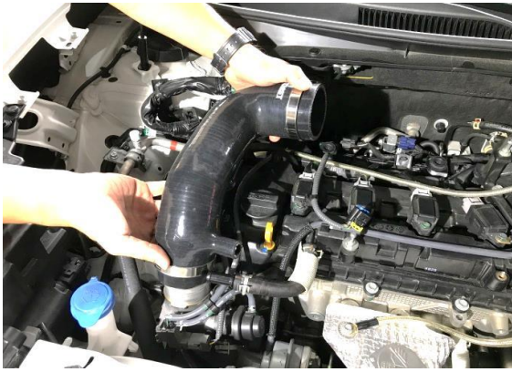
Figure 17. Install the MST silicone tube.
