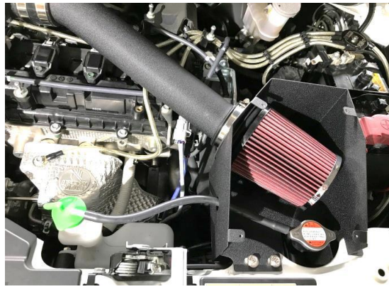
Figure 29. Install the air filter.
