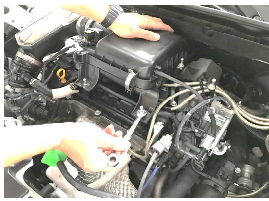
Figure 7. Remove the air box bolts.
