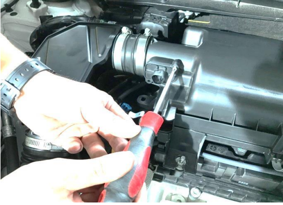
Figure 10 . Remove the MAF sensor from the airbox.
