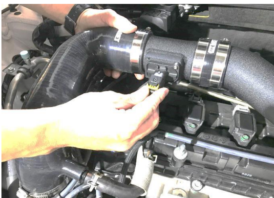
Figure 28. Connect the MAF plug to the MAF sensor.
