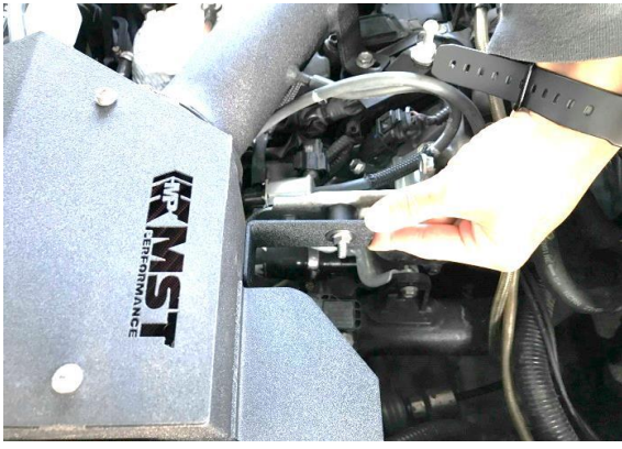
Figure 25. Install the bracket B ★Choose the proper bracket (A or B) for the model version
