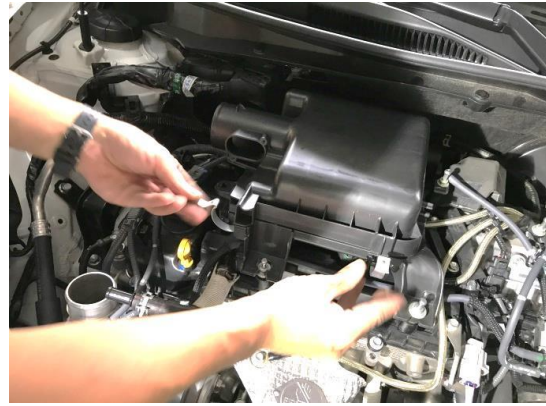
Figure14. Open the air box cover.
