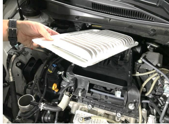
Figure 15. Remove the stock air filter.
