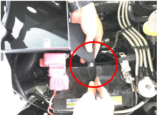
Figure 23. Secure the heat shield bracket A at battery side with bolt. *Choose Bracket B if there's no the same mounting point for your vehicle model.
