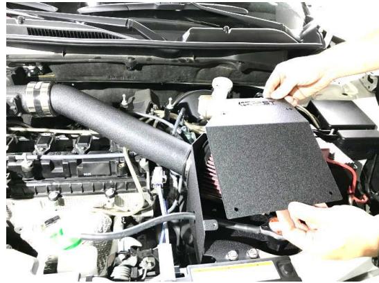
Figure 30. Install the heat shield cover.
