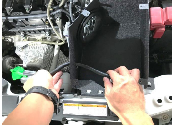
Figure 22. Get the hose through the heat shield.
