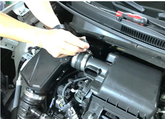
Figure 12. Loosen the hose clamp.
