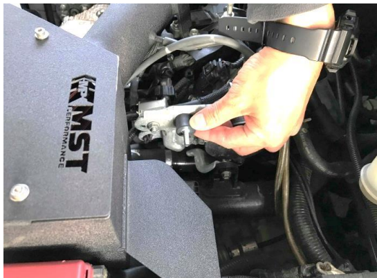
Figure 24. Install the mount Rubber. *Choose bracket B for your vehicle model
