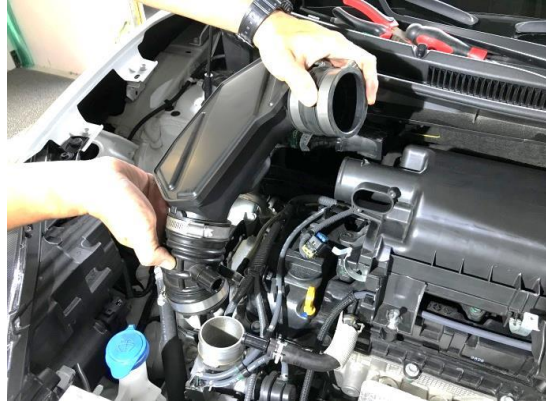
Figure 13. Remove the stock tube.
