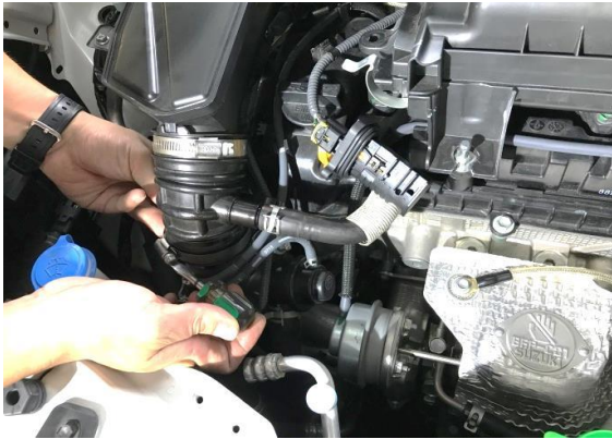
Figure 11. Loosen the hose clamp.
