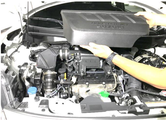
Figure 2. Remove the engine cover.
