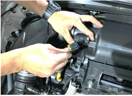
Figure 9. Disconnect the mass air sensor.
