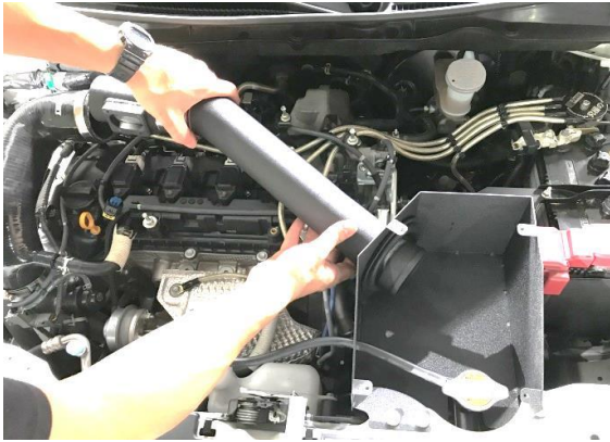
Figure 26. Install the intake tube.
