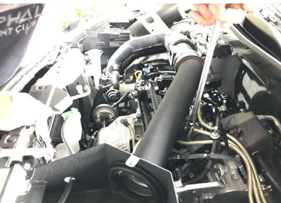
Figure 27. Connect the MAF plug to the MAF sensor.
