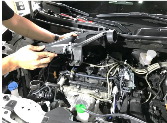
Figure 16. Remove the stock air box.
