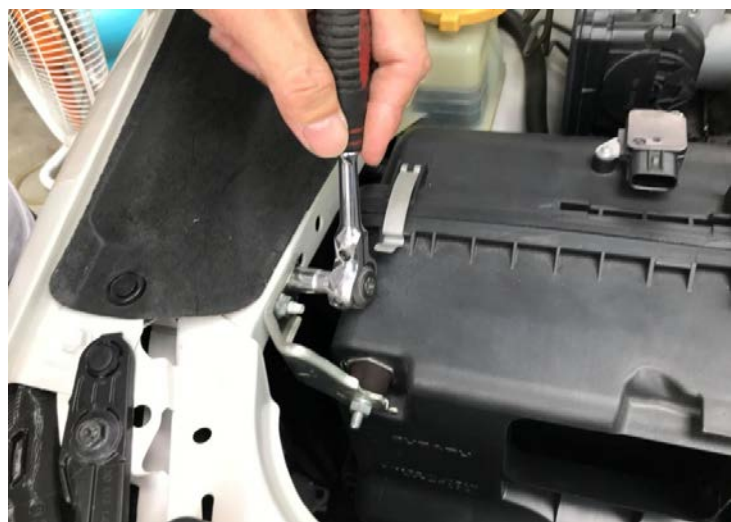
Figure 7: 轉開原廠集氣箱螺絲
