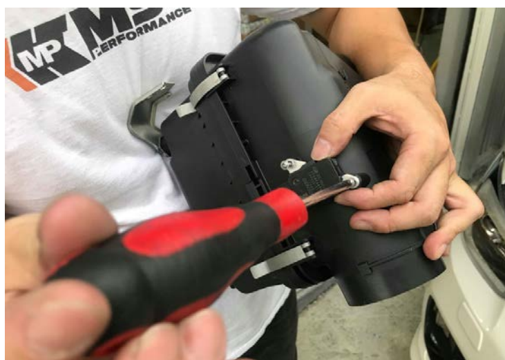
Figure 10: 轉開原廠MAF感應器螺絲
