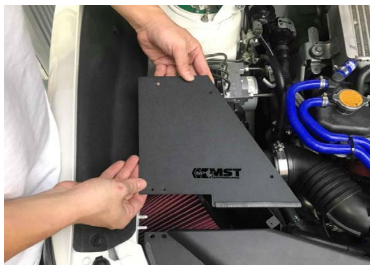
Figure 27: 安裝隔熱罩上蓋
