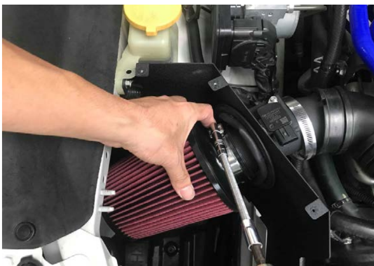
Figure 22: 鎖緊濾心管束
