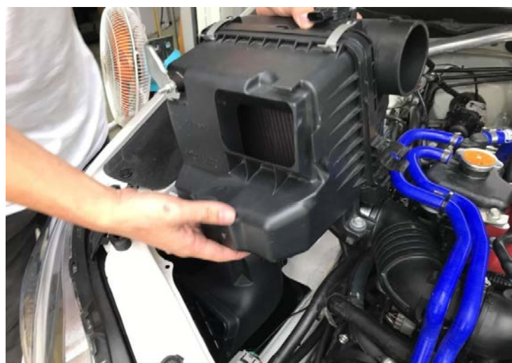
Figure 9: 移除原廠集氣箱
