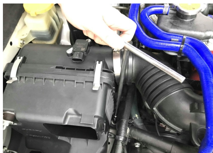
Figure 8: 轉開原廠集氣箱螺絲
