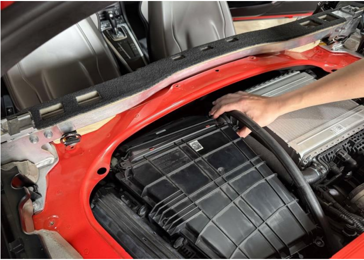
Figure 2: Separate the buckle on the stock intake tube from the stock air box.
