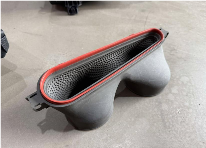
Figure 8: Instakk the o-ring on the MST tube.
