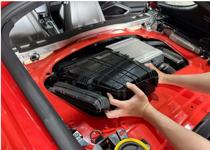
Figure 3: Remove the stock air box and air scoop.
