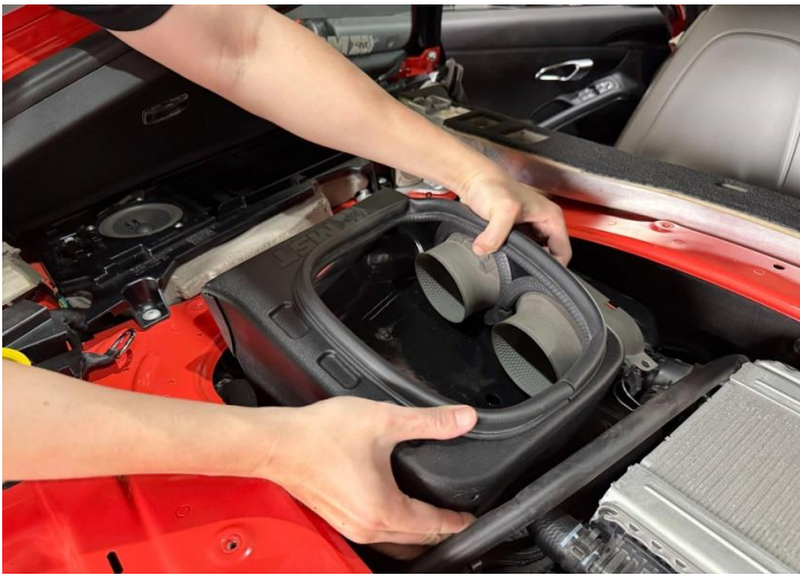
Figure 10: Install the MST air box and tube.
