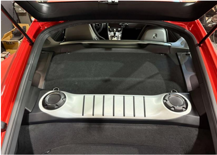
Figure 14: Re-install the engine cover. Congratulations! You have just completed the installation of this intake system. Periodically, check the alignment of the intake, normal wear and tear can cause nuts and bolts to come loose.
