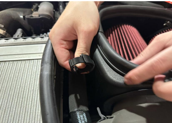
Figure 12: Lock radiator hose.
