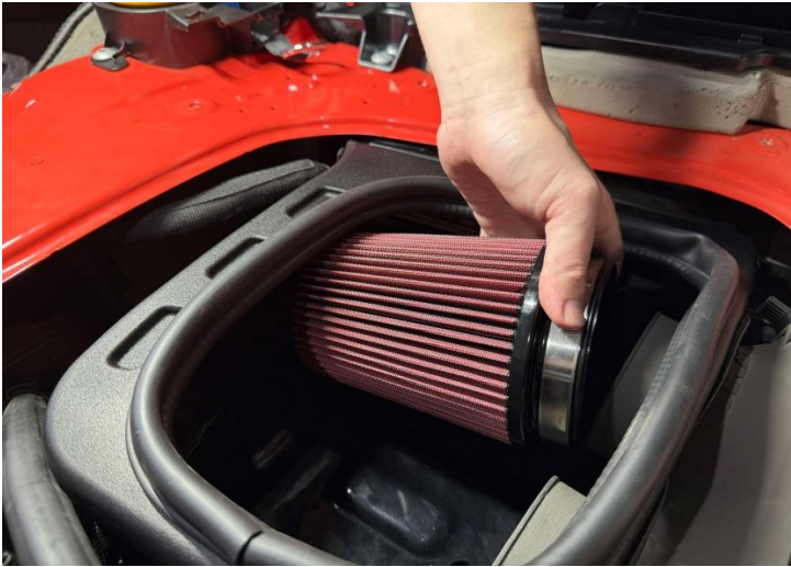
Figure 11: Install the MST air filter.
