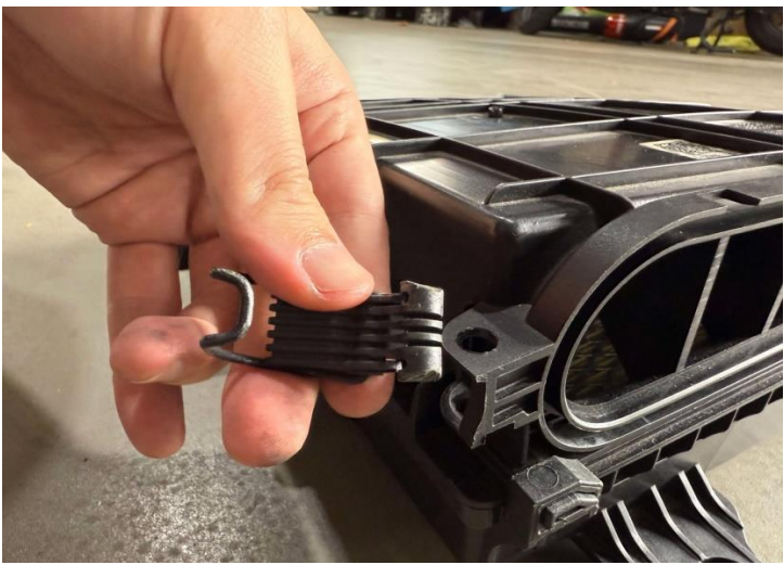
Figure 4: Remove the buckle from stock air box.
