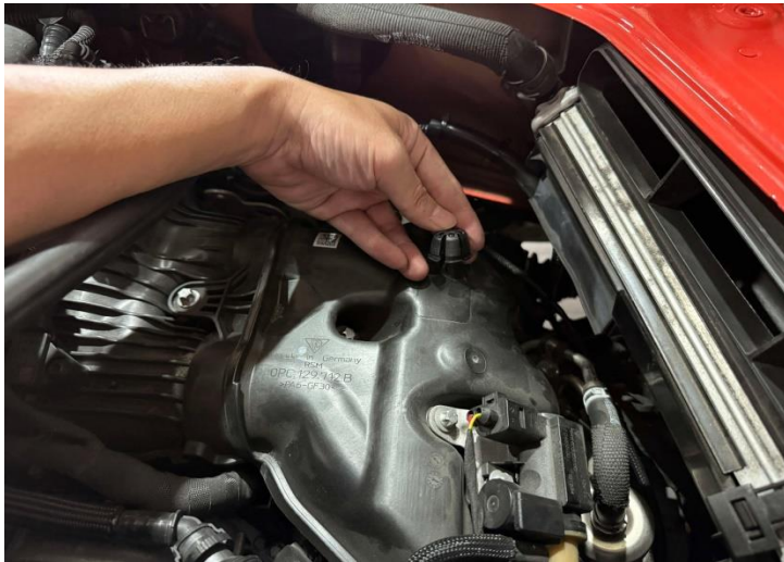
Figure 9: Install the fixed buckle *3 on the engine.
