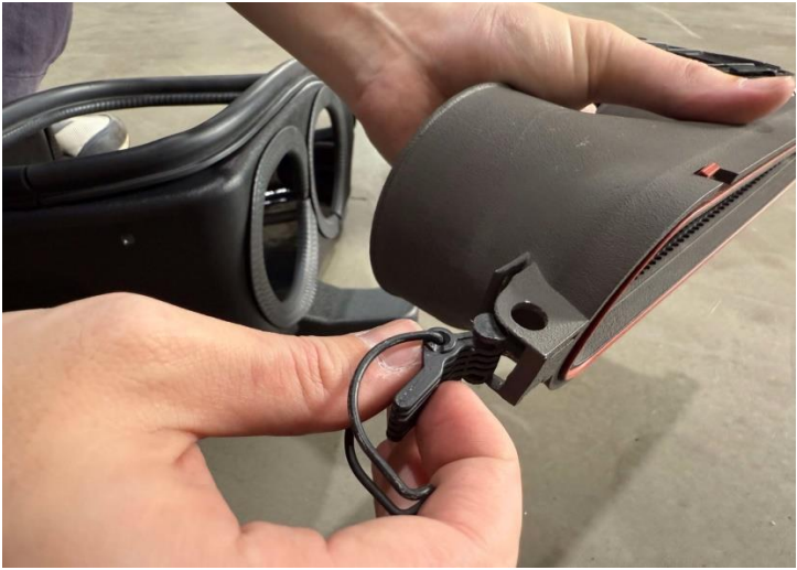
Figure 6: Install the buckle on the MST tube.
