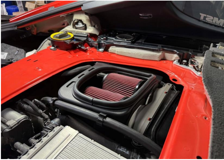
Figure 13: MST intake install completed.
