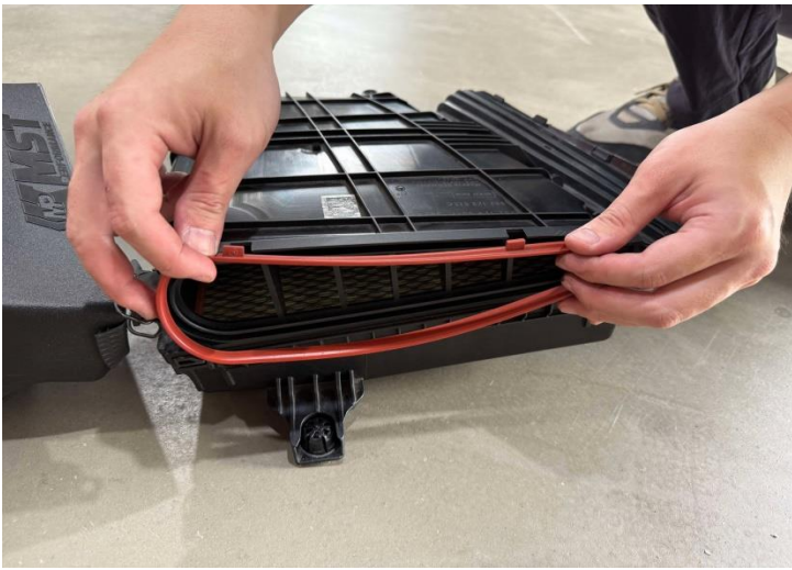
Figure 7: Remove the o-ring from stock air box.
