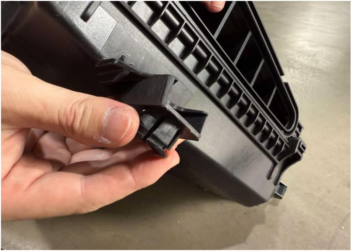
Figure 5: Remove the fixed buckle *3 from stock air box.
