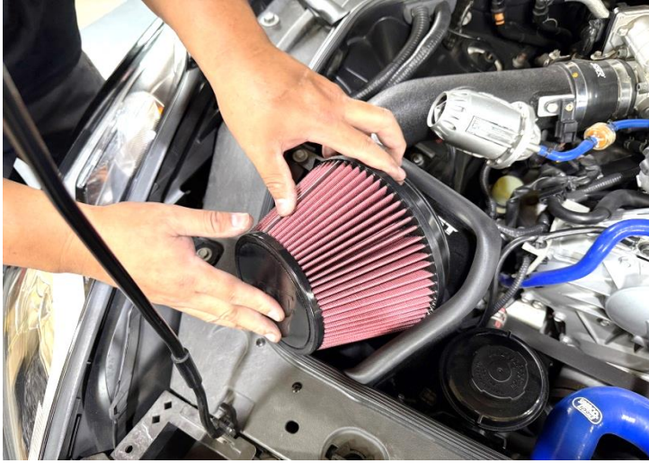
Figure 25: Install the MST filter.
