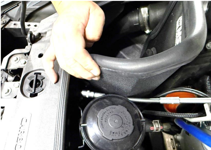
Figure 14: Install heat shield bracket and tighten the bolts.
