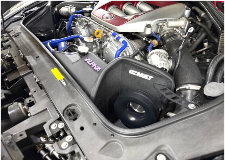
Figure 24: Heat shield and air intake tube installation completed
