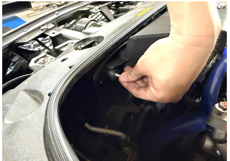
Figure 17: Remove the stock rubber mount.
