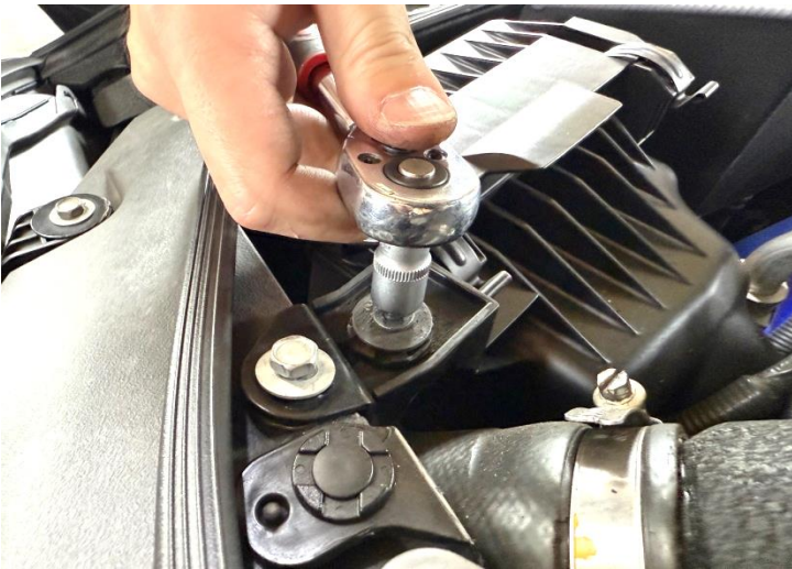
Figure 2: Remove stock air box bracket bolts and air box cover.
