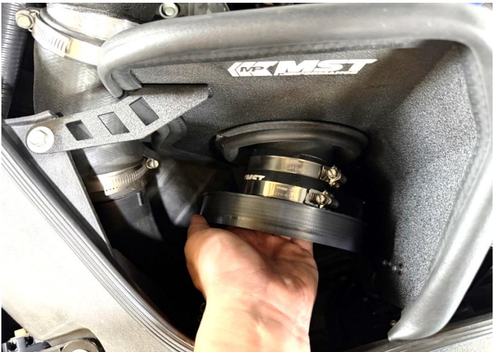
Figure 23: Install the velocity stack on the MST tube.
