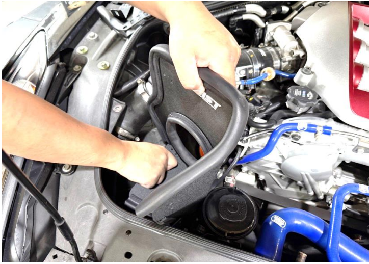
Figure 13: Install the heat shield.
