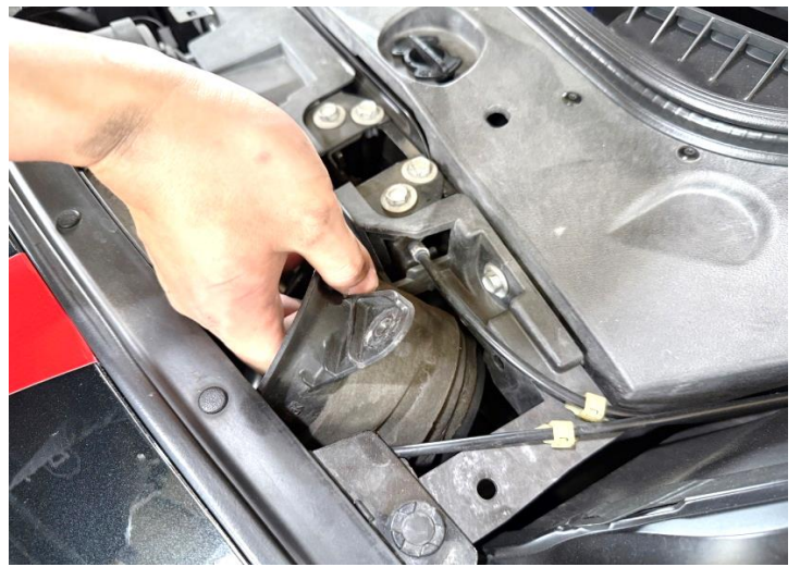
Figure 4: Remove the stock snorkel.
