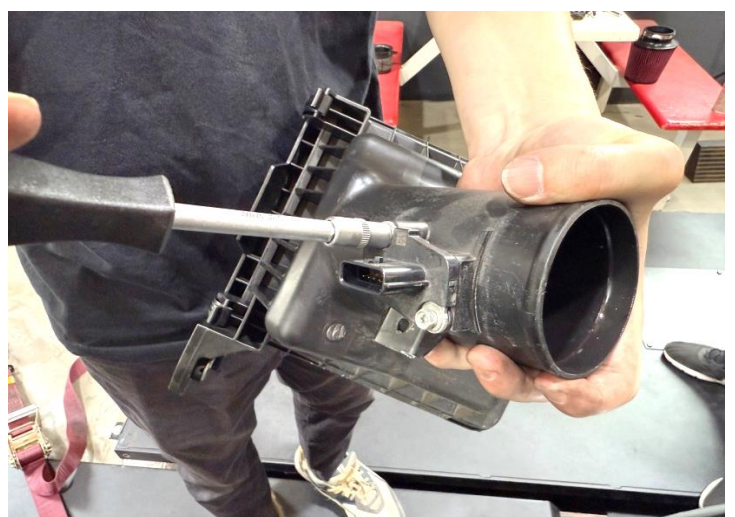
Figure 12: Remove the MAF from the stock air box.
