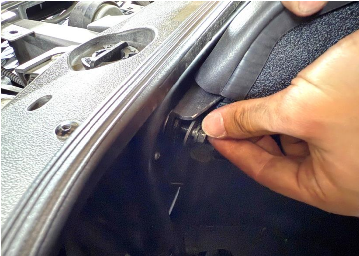
Figure 19: tighten the bracket bolts.
