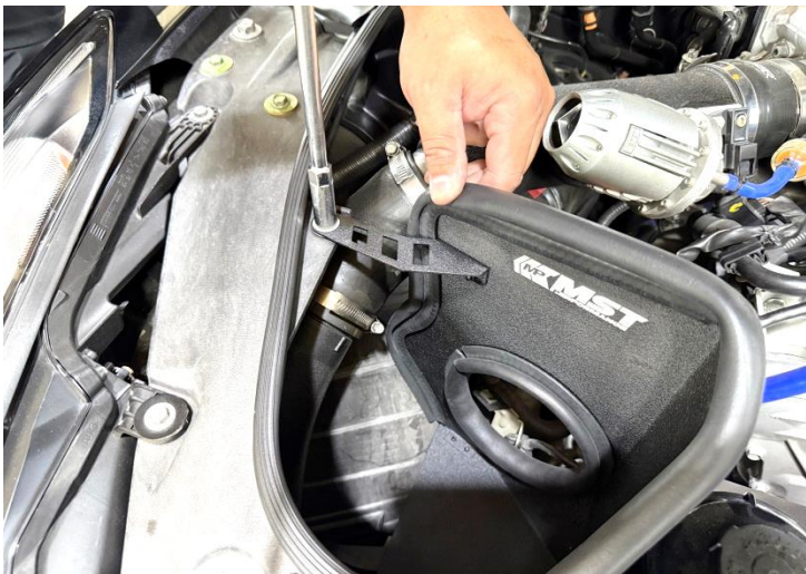
Figure 15: Install heat shield bracket and tighten the bolts.
