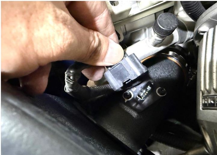
Figure 21: Install the MAF sensor and plug in the sensor connector.
