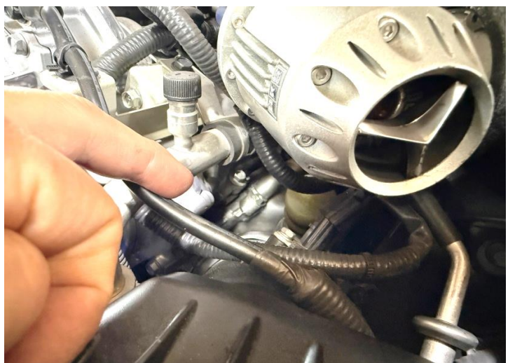
Figure 6: Disconnect the MAF sensor.
