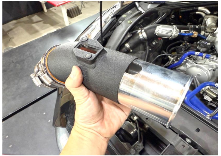
Figure 10: * Vehicle is stock tune please install MAF sleeve.
