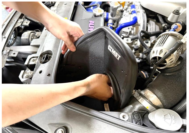
Figure 18: Install the heat shield.
