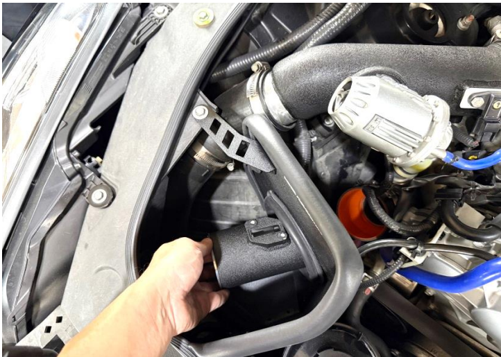
Figure 20: Install the MST tube.
