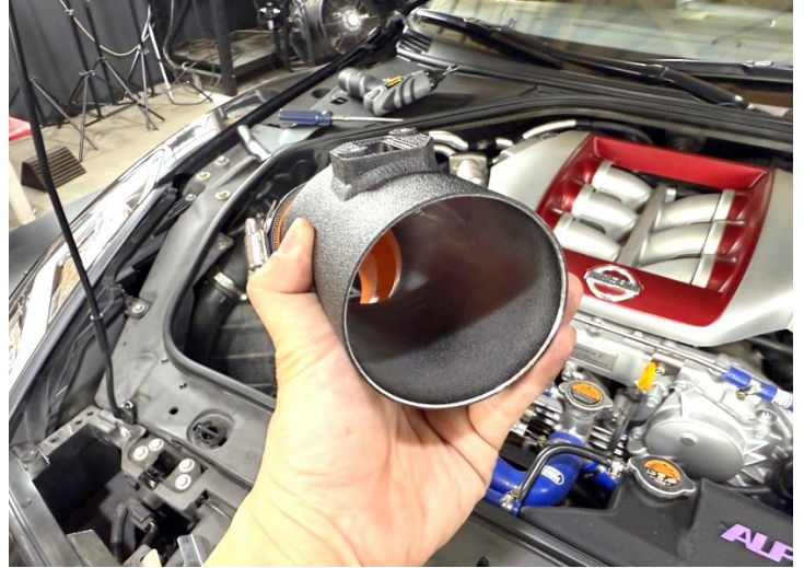
Figure 11: * Vehicle is a 3" tube remap tune, do not install the MAF sleeve.
