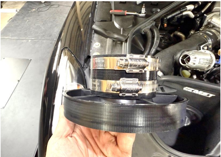
Figure 22: Install the 76-76 hose on the velocity stack.
