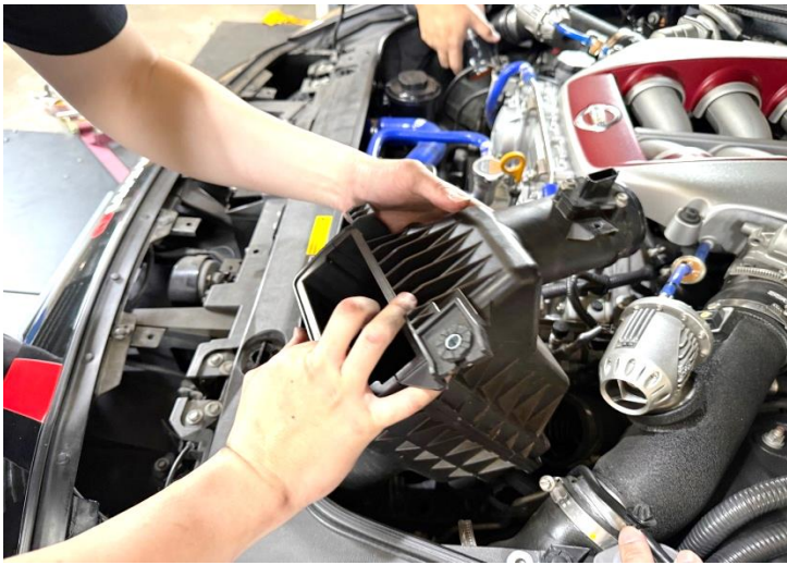
Figure 7: Remove the stock air box.
