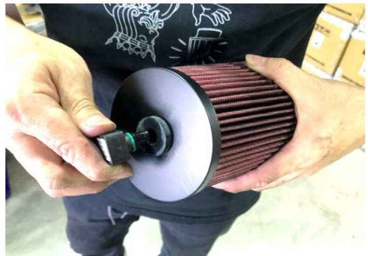
Figure 12: Put into the filter rubber and feel it tight 圖十二: 將之放進濾膠並感受到緊實度
