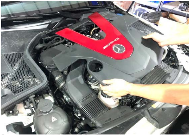
Figure 1: Remove the engine cover by lifting up at all for corners.圖一: 藉由四角處將引擎蓋掀起
