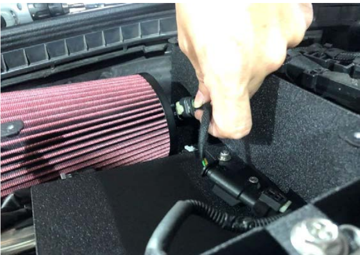
Figure 15: Connect the mass air sensor. Make sure the wire is smooth and has "No twist" 圖十五: 連結空氣質量傳感器。務實線路是順的且沒有任何彎曲。
