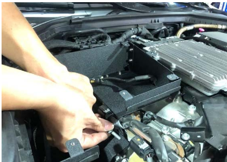
Figure 9: Secure with bolt. 圖九: 用螺栓將其鎖緊
