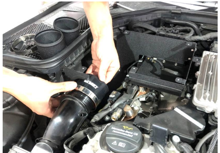
Figure 9: Install the intake tube and silicone hose. 圖十: 安裝進氣管和矽利康軟管
