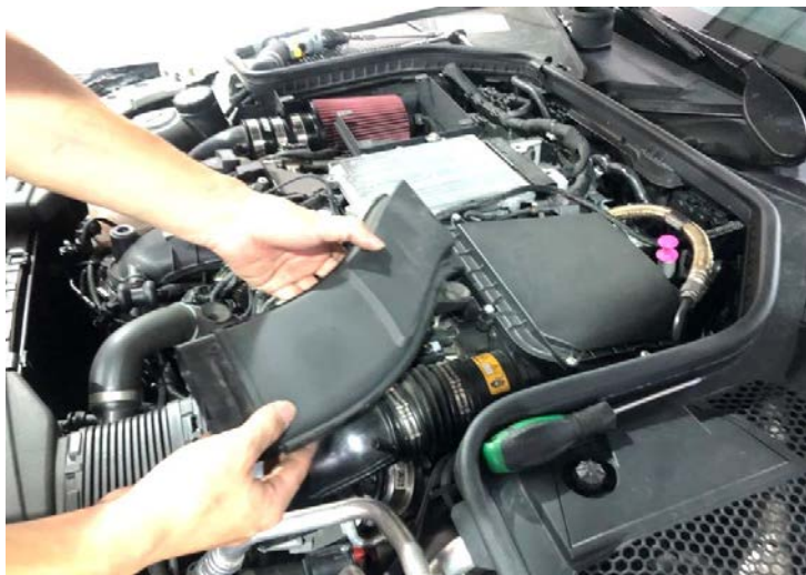
Figure 2: Remove the air ducts. 圖二: 移除風管
