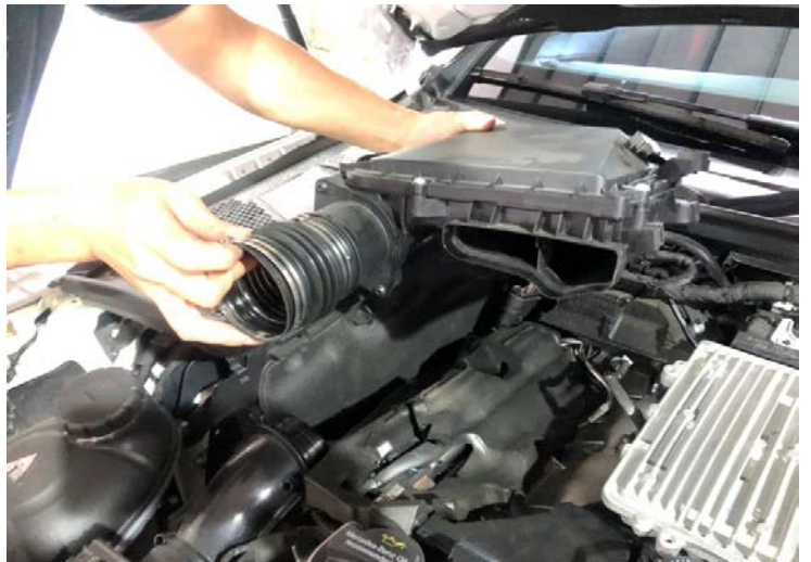
Figure 5: Remove the factory airbox assembly from the vehicle. 圖五: 將原廠空氣箱零件從車子移除
