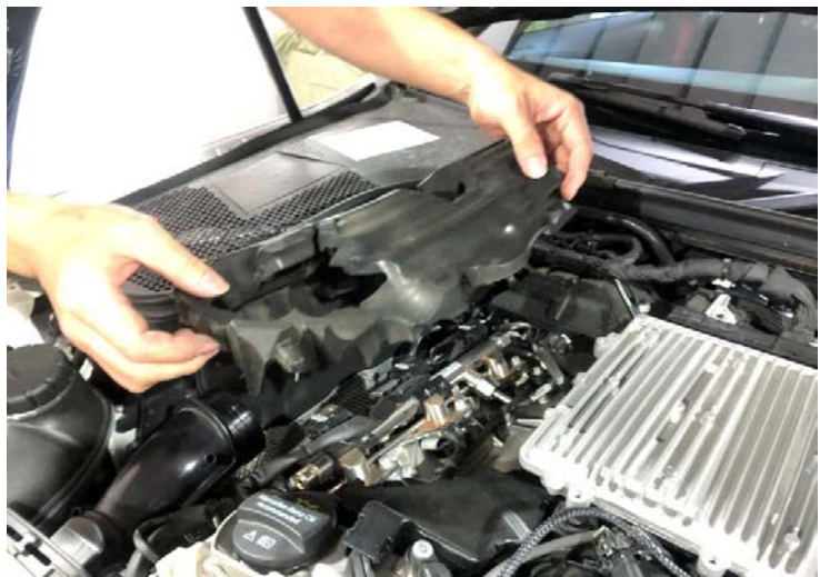
Figure 6: Remove the insulated foam. 圖六: 移除絕緣泡沫板
