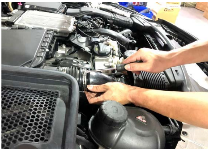
Figure 3: Loosen hose clamp at the factory airbox. 圖三: 鬆開空氣箱的軟管夾
