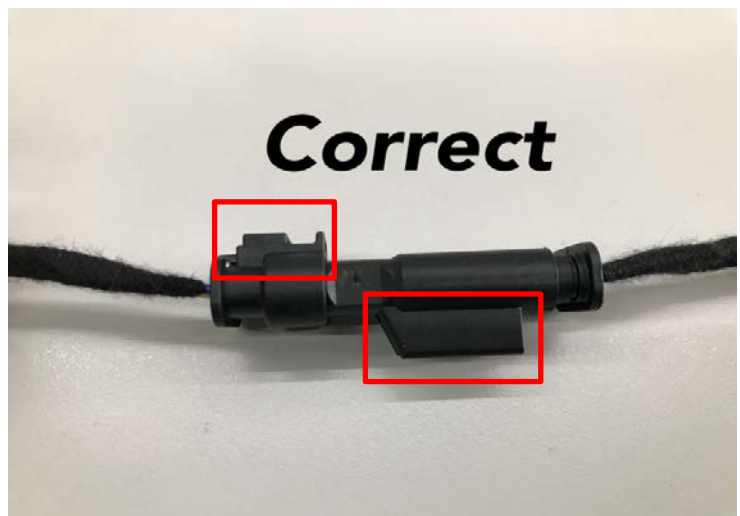
The correct way for connecting the extension cord (side view) 連接延長線的正確方式(側面視角)
