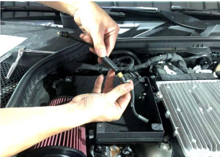
Figure 14: Electrical extensions to plug them back in to the factory wiring harness. 圖十四: 將電子延長線插回原廠線束內
