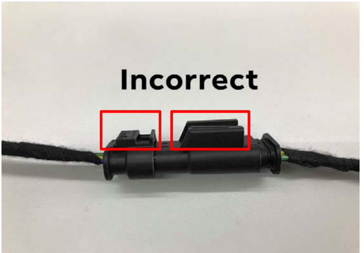
This is the incorrect way for connecting which will trigger the engine management light 這是不正確的連接方法。會使引擎室管理的燈亮起。
