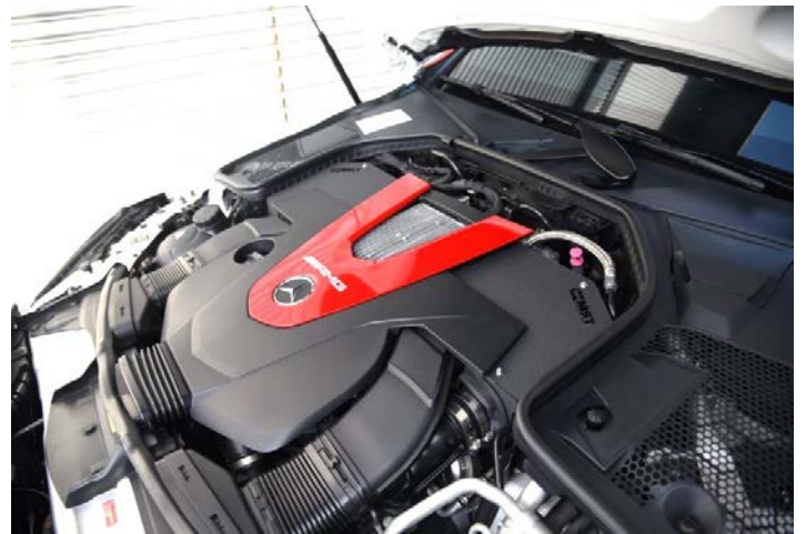
Figure 20: Congratulations! You have just completed the installation of this intake system. Periodically, check the alignment of the intake, normal wear and tear can cause nuts and bolts to come loose.
