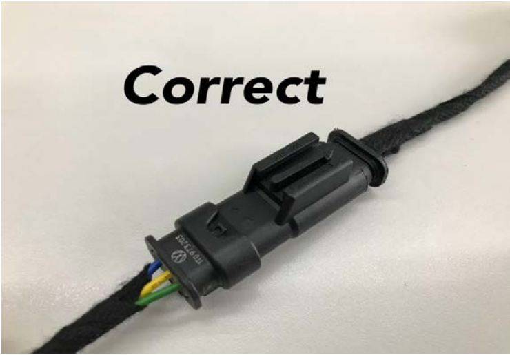
The correct way for connecting the extension cord (front view) 連接延長線的正確方式(前方視角)
