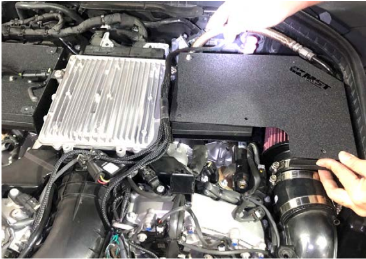
Figure 16: Install the heat shield cover and secure with bolt. M4 Bolt 8mm x5 圖十六: 安裝善熱蓋並用螺栓鎖緊。 M4 螺栓 8mm x5
