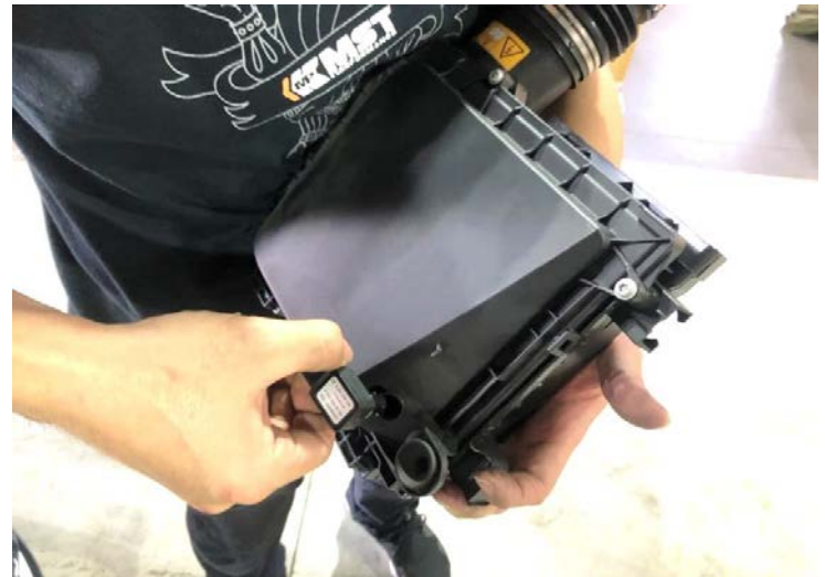
Figure 11: Remove the sensors from the factory airbox carefully 圖十一: 小心的將感應器從原廠空氣箱拔下
