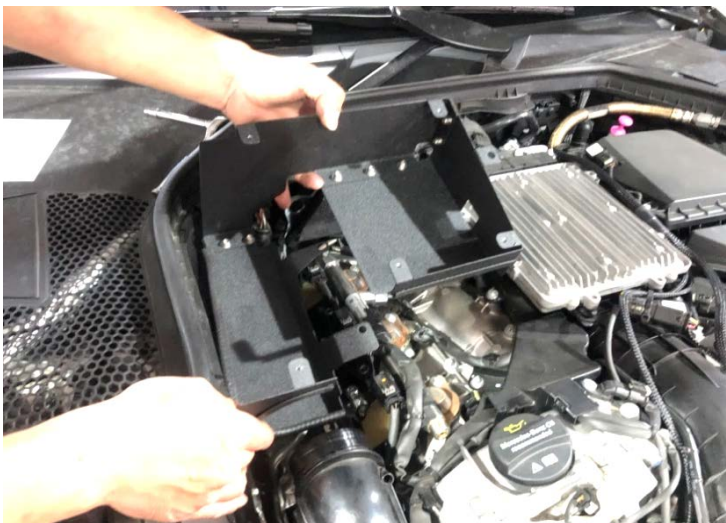
Figure 8: Set the heat shield. 圖八: 安裝防熱蓋
