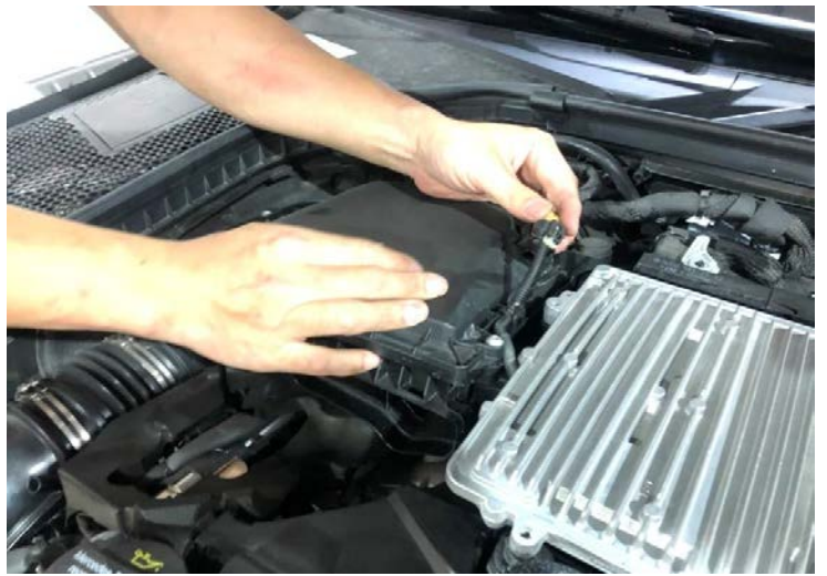
Figure 4: Unclip the sensor. 圖四: 鬆開感應器
