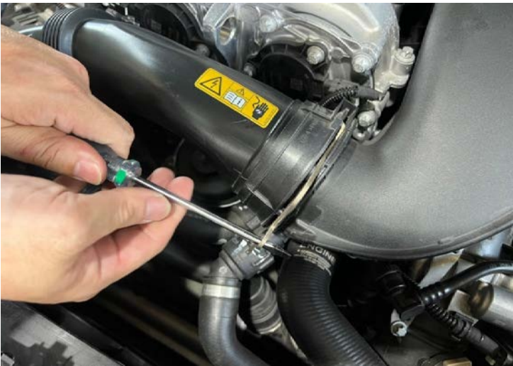
Figure 3: Remove the spring from the stock intake tube. 從進料管上拆下彈簧
