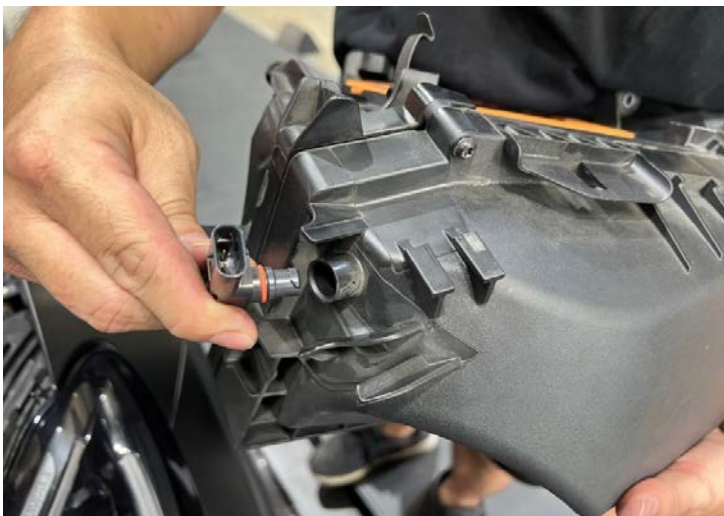
Figure 32: Remove the pressur sensor from stock air box. 從原廠空氣箱取出壓力感知器
