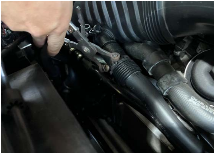
Figure 2: Remove the PCV plug.拆下 PCV 插頭
