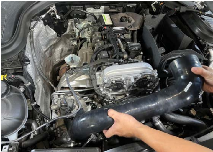
Figure 26: Install the silicone hose.安裝矽膠軟管
