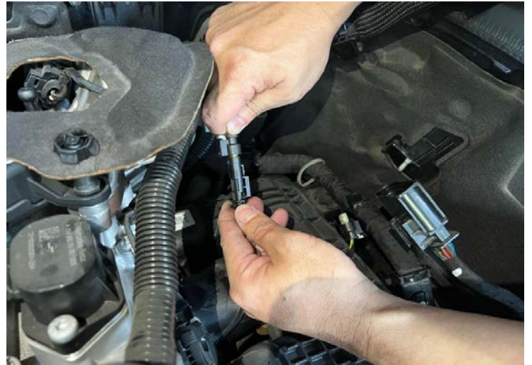
Figure 22: Connect the electrical extension.連接電氣擴展
