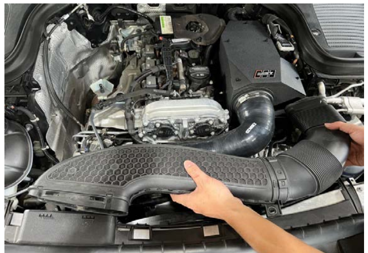
Figure 36: Reinstall the factory scoop. 重新安裝原廠導風管
