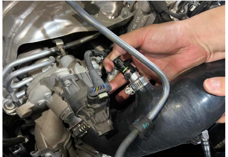
Figure 28: Connect the PCV plug * 4.連接PCV插頭*4
