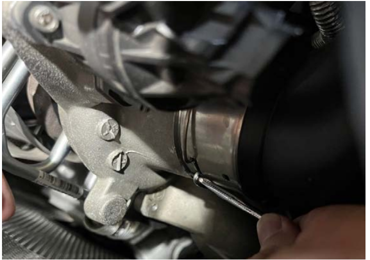
Figure 4: Remove the spring from the stock intake tube. 從進料管上拆下彈簧
