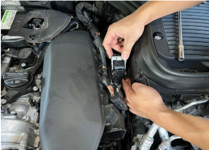
Figure 8: Remove the plug. 拔下插頭
