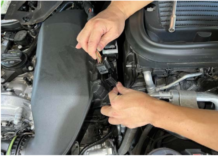
Figure 7: Remove the plug. 拔下插頭
