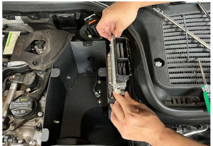
Figure 30: Install the DME on the heat shield. 將 DME 安裝在隔熱罩上
