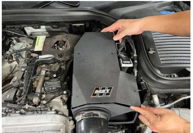
Figure 35: Install the heat shield cover.安裝隔熱罩
