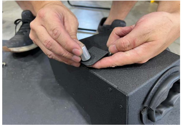
Figure 16: Install the mounts on the brackets. 將安裝座安裝到支架上
