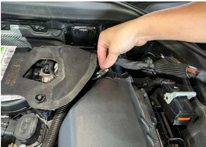
Figure 9: Remove the pressure sensor plug from air box. 從氣箱中拆下壓力感知器插頭
