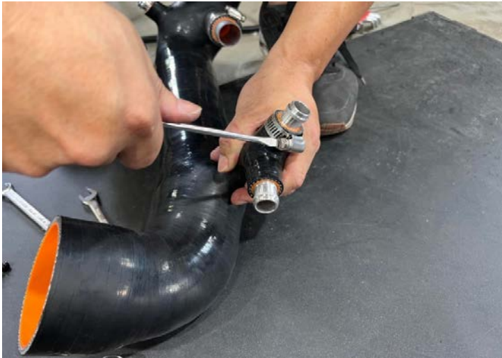
Figure 25: Install the PCV hose connector on the silicone hose.將 PCV 軟管接頭安裝到矽膠軟管上
