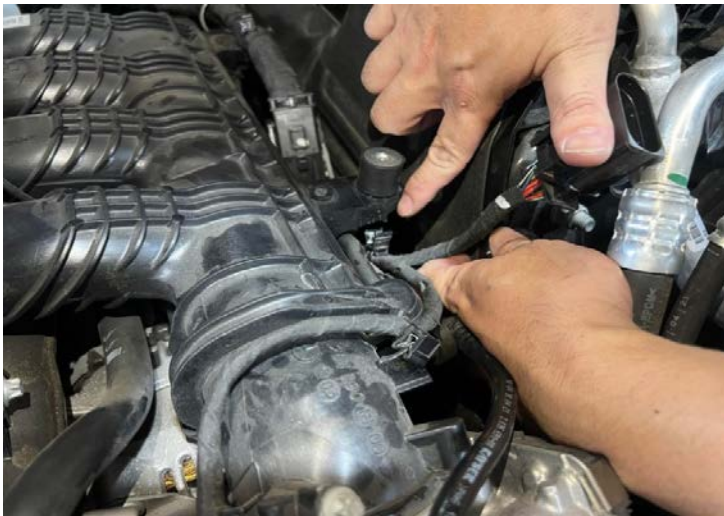
Figure 20: Remove the clip.取下夾子
