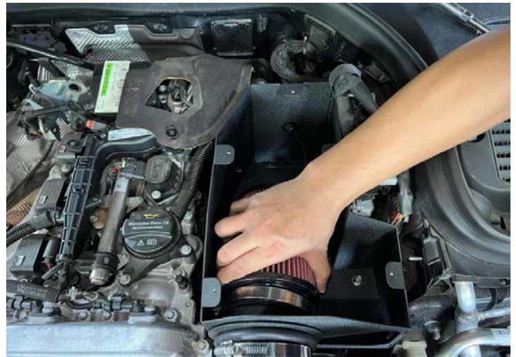
Figure 34: Install the MST filter.安裝 MST 過濾器
