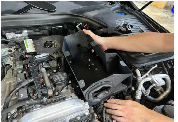
Figure 23: Install the MST heat shield.安裝 MST 隔熱罩
