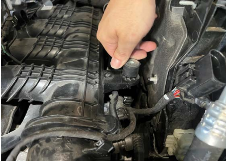
Figure 19: Install the cylindrical mount. 安裝圓柱形安裝座
