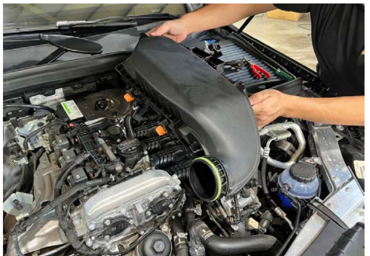
Figure 12: Remove the stock air box. 拆下庫存空氣箱
