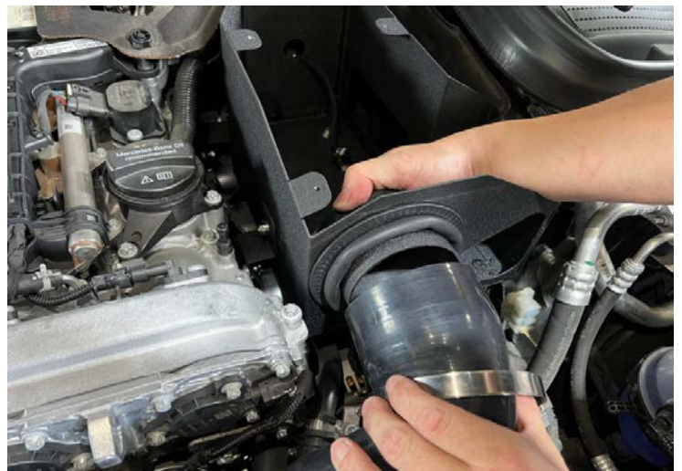
Figure 29: Install the 83-89 tube.安裝83-89鋁管
