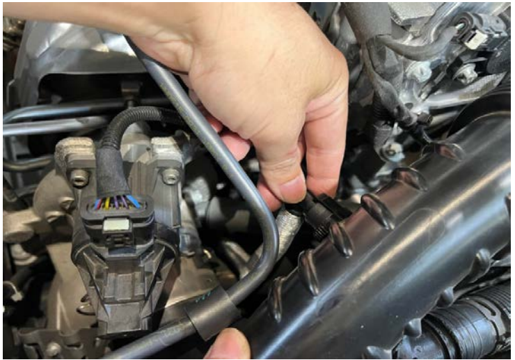
Figure 5: Remove the PCV plug.拆下 PCV 插頭
