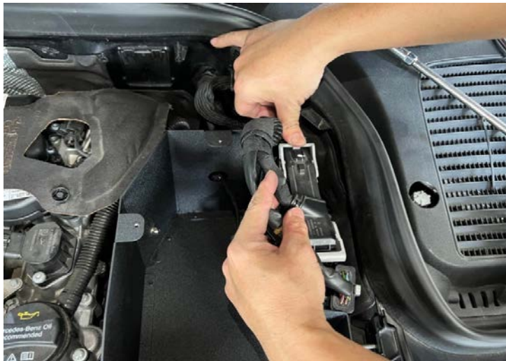
Figure 31: Connect the DME plug. 連接 DME 插頭
