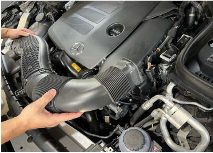
Figure 1: Remove the factory scoop from the vehicle. 從車上拆下導風管
