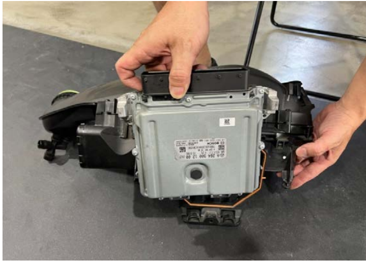
Figure 13: Remove the DME from stock air box. 從備用空氣箱中取出 DME
