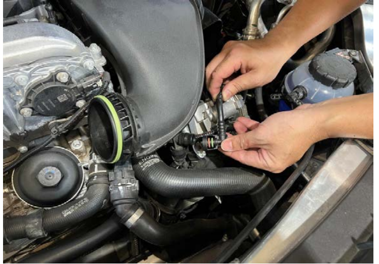
Figure 11: Remove the PCV plug. 拆下 PCV 插頭
