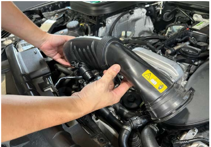
Figure 6: Remove the stock intake tube.拆下進料管
